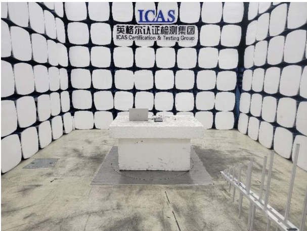
Radiated Emission test set-up for 30M-1GHz, TM133
