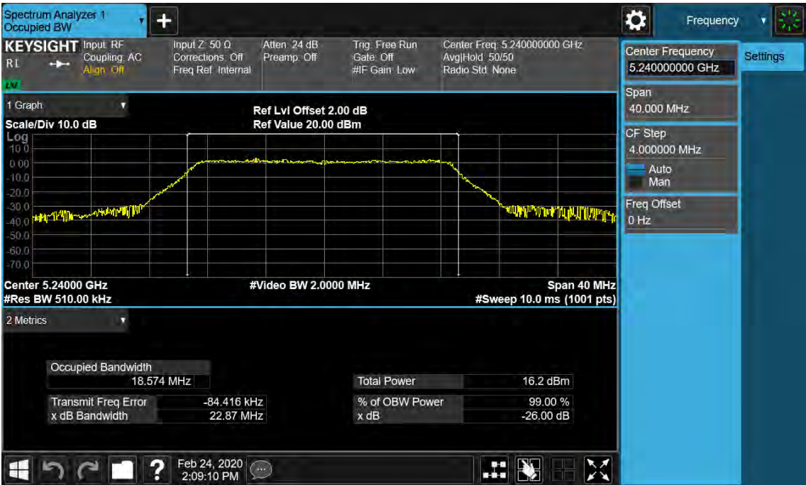
Figure 10: 26dB Bandwidth and 99% Bandwidth, 802.11n(HT40), 5190MHz
