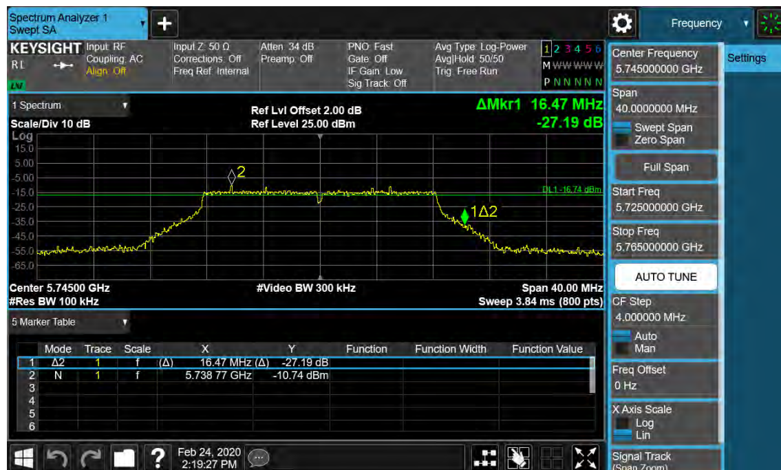
Figure 29: 6dB Bandwidth, 802.11a, 5745MHz
