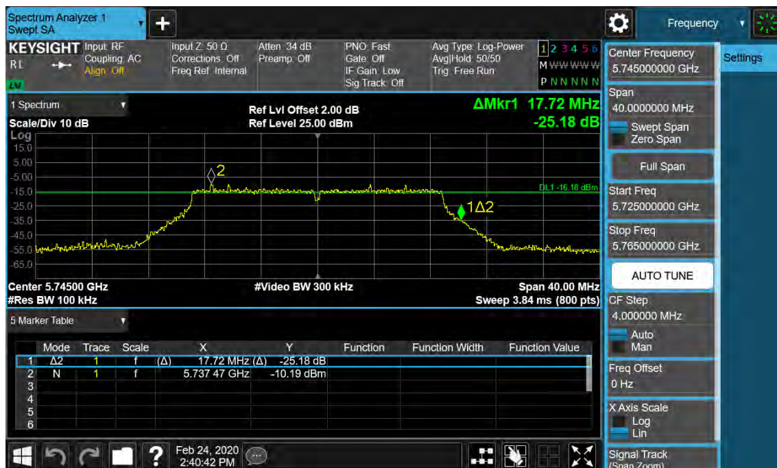
Figure 35: 6dB Bandwidth, 802.11ac(VHT20), 5745MHz
