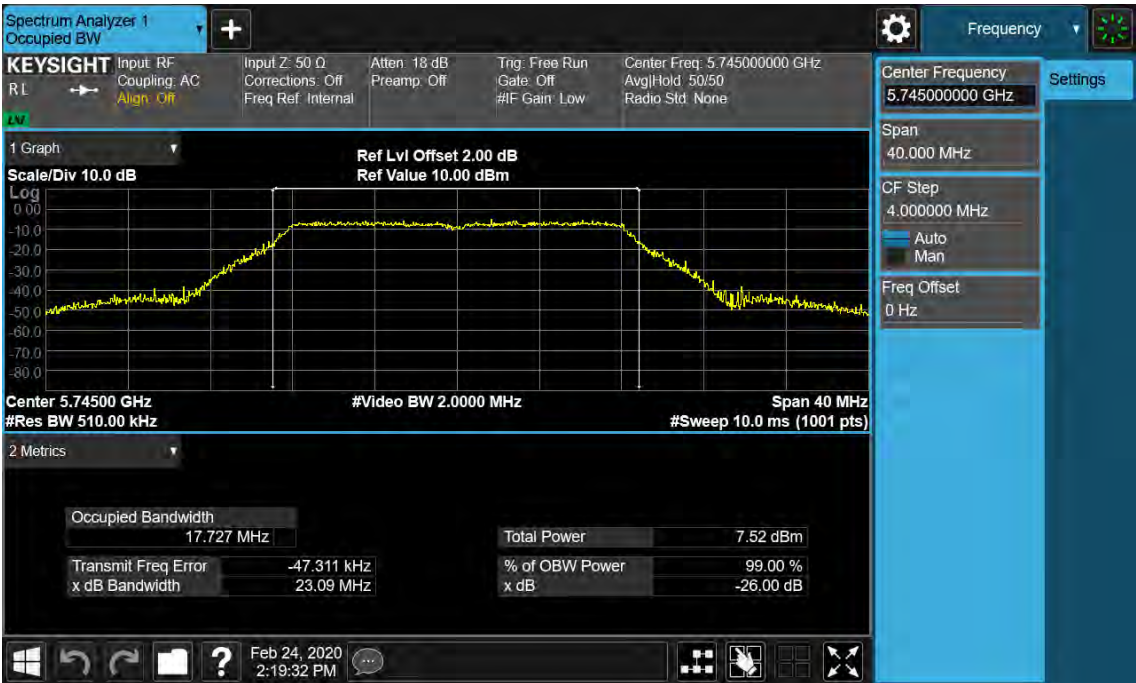
Figure 16: 26dB Bandwidth and 99% Bandwidth, 802.11a, 5785MHz
