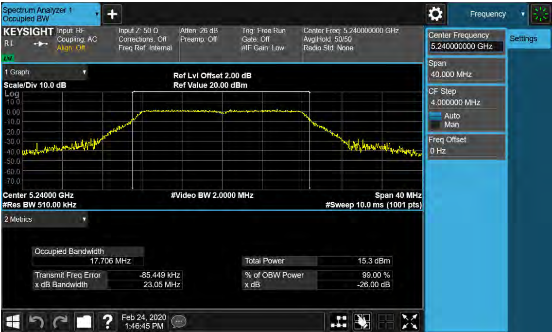
Figure 4: 26dB Bandwidth and 99% Bandwidth, 802.11n(HT20), 5180MHz
