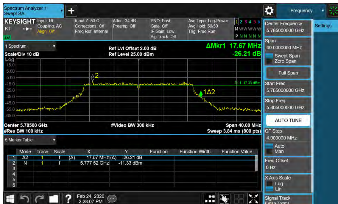
Figure 33: 6dB Bandwidth, 802.11n(HT20), 5785MHz
