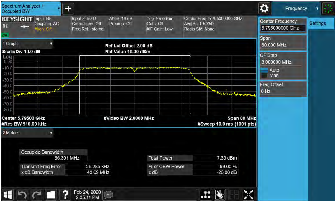
Figure 26: 26dB Bandwidth and 99% Bandwidth, 802.11ac(VHT40), 5755MHz
