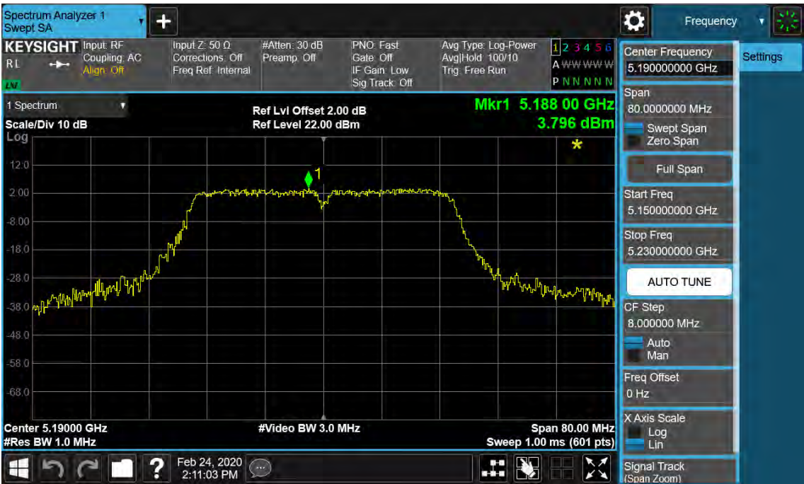
Figure 54: Power Spectral Density, 802.11ac(VHT40), 5190MHz
