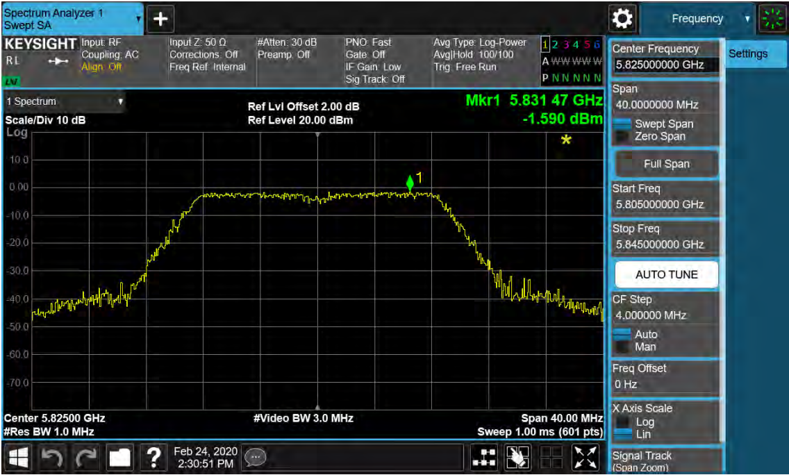
Figure 62: Power Spectral Density, 802.11n(HT20), 5825MHz
