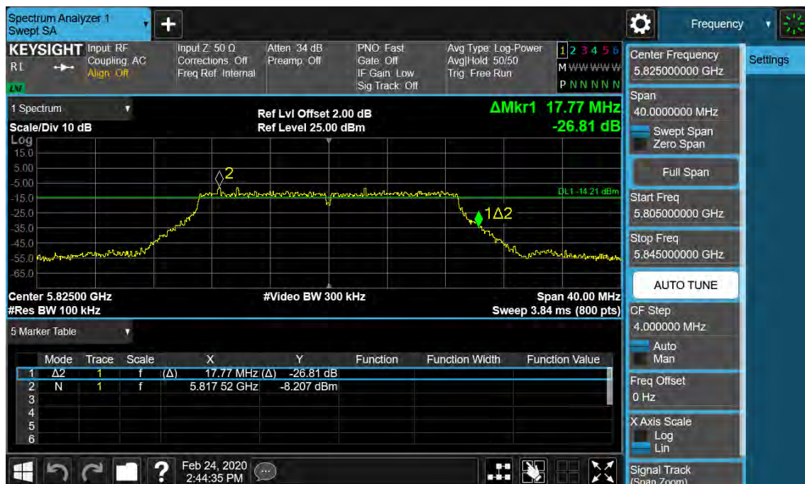
Figure 37: 6dB Bandwidth, 802.11ac(VHT20), 5825MHz
