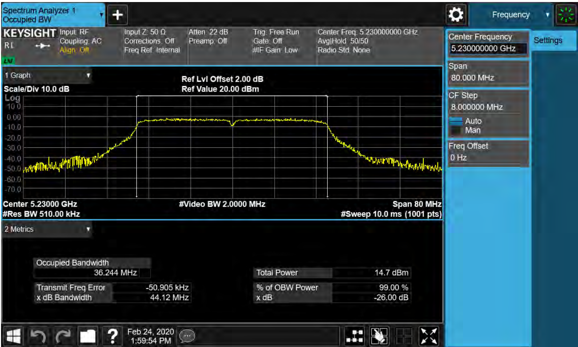
Figure 12: 26dB Bandwidth and 99% Bandwidth, 802.11ac(VHT40), 5190MHz
