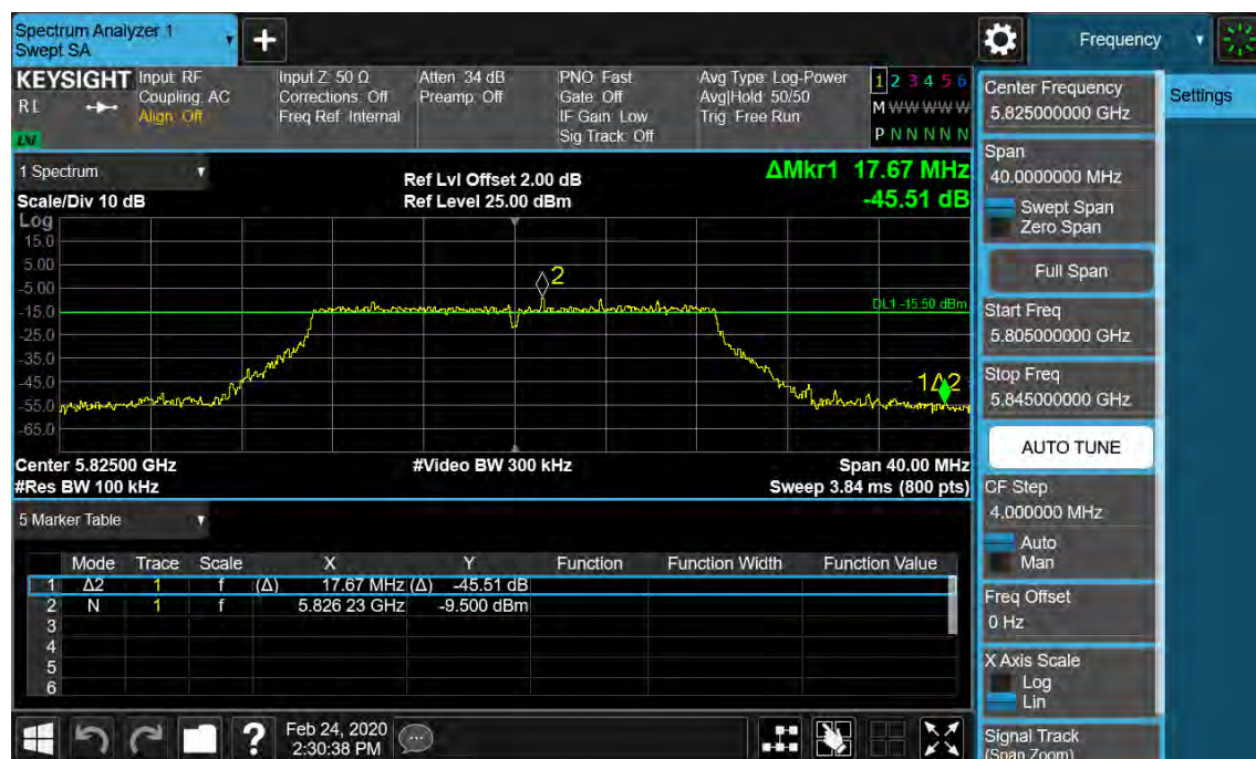
Figure 34: 6dB Bandwidth, 802.11n(HT20), 5825MHz
