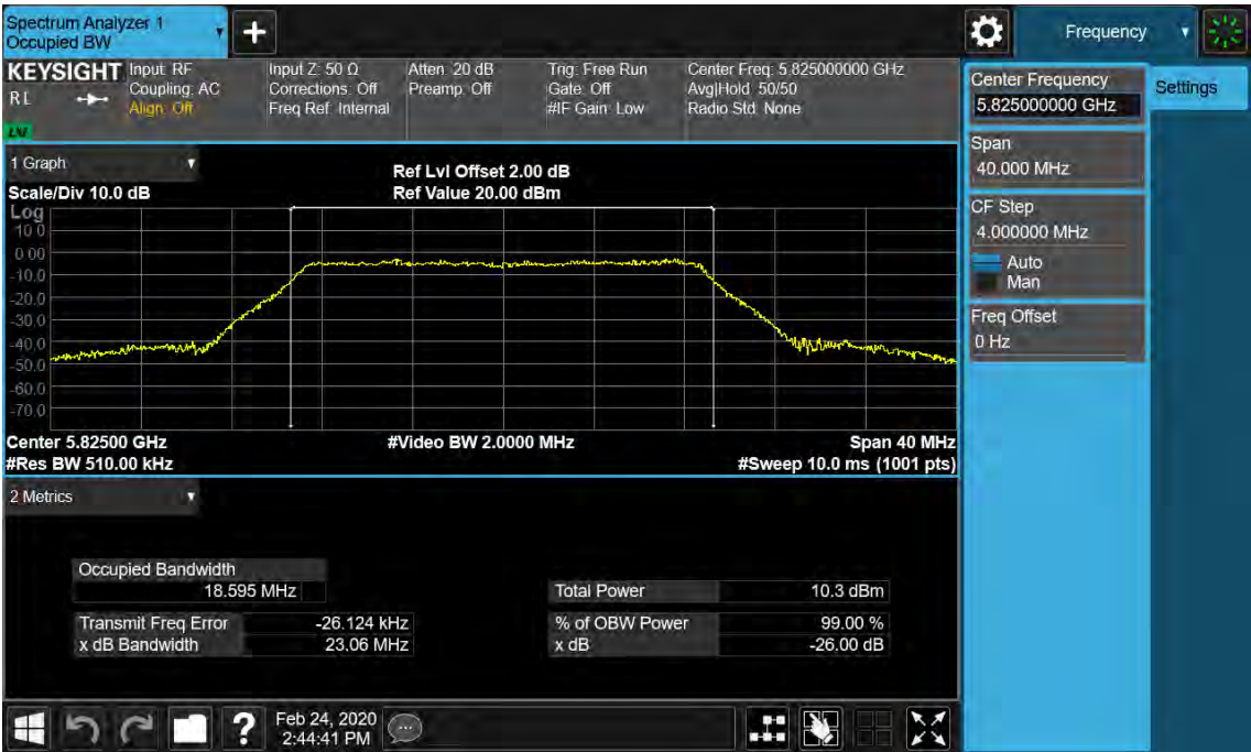
Figure 24: 26dB Bandwidth and 99% Bandwidth, 802.11n(HT40), 5755MHz
