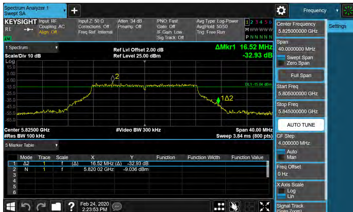
Figure 31: 6dB Bandwidth, 802.11a, 5825MHz
