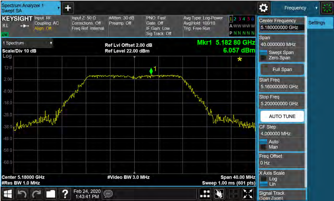
Figure 43: Power Spectral Density, 802.11a, 5180MHz
