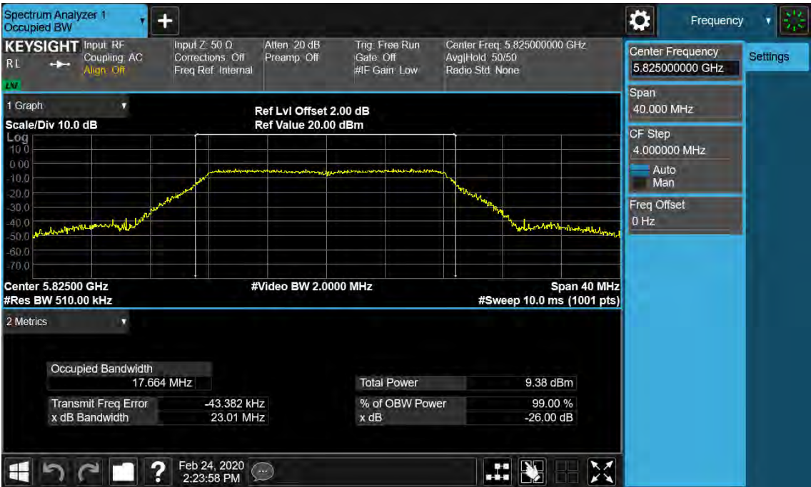
Figure 18: 26dB Bandwidth and 99% Bandwidth, 802.11n(HT20), 5745MHz
