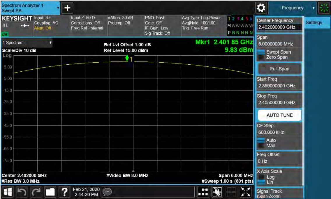
Figure 7: Maximum Conducted Output Power, 2402MHz, 8-DPSK
