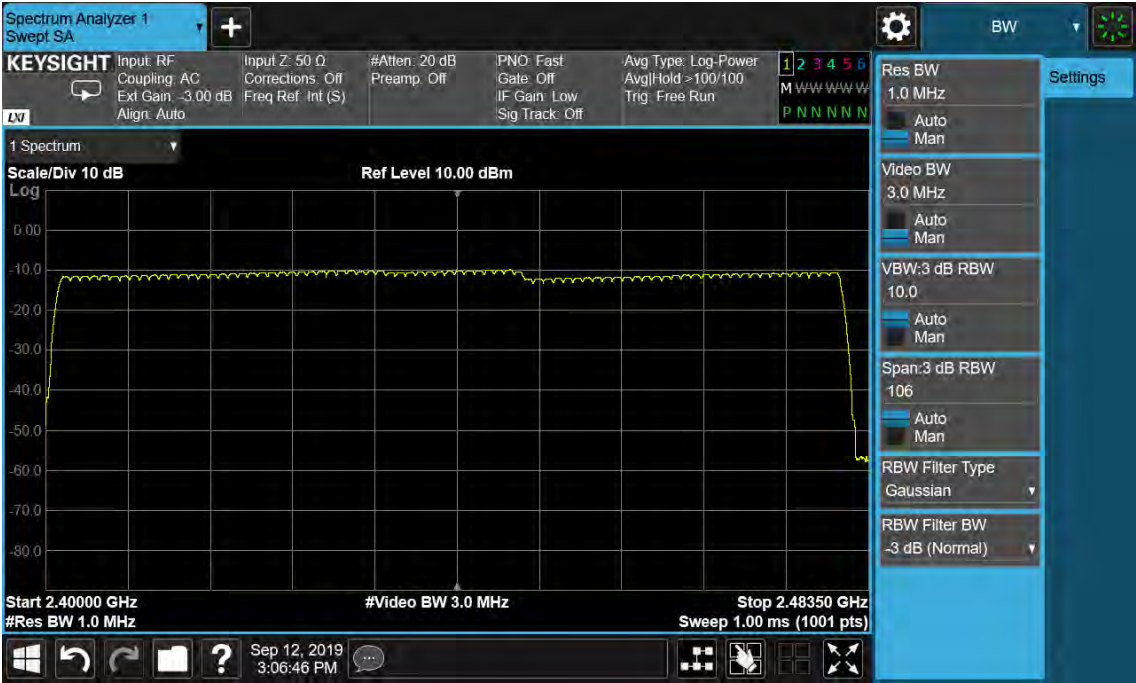
Figure 41: Number of Hopping Frequency, Hopping Mode, GFSK
