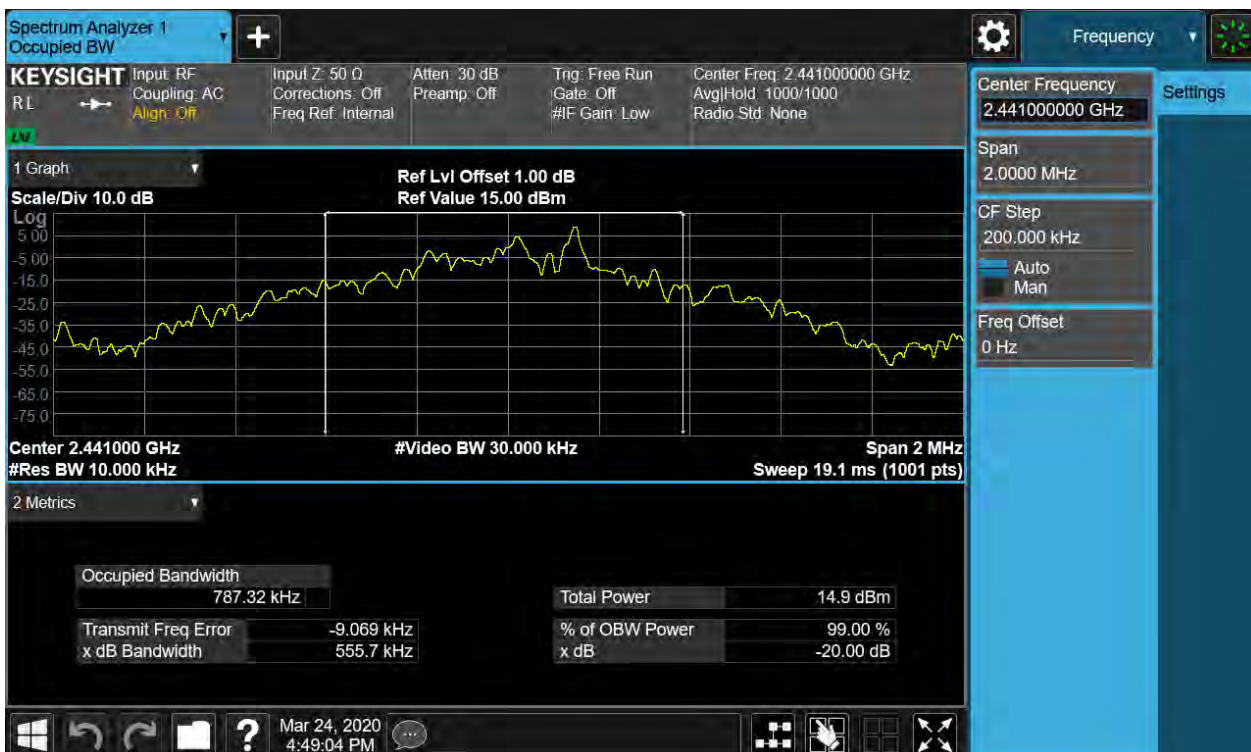
Figure 11: 20dB Bandwidth and 99% Bandwidth, 2441MHz, GFSK
