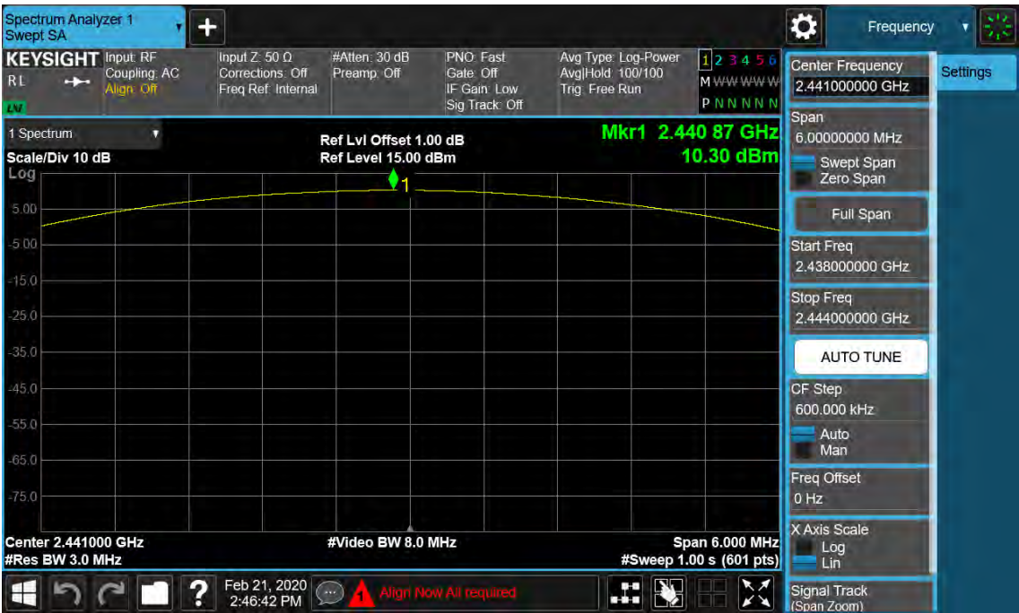
Figure 8: Maximum Conducted Output Power, 2441MHz, 8-DPSK
