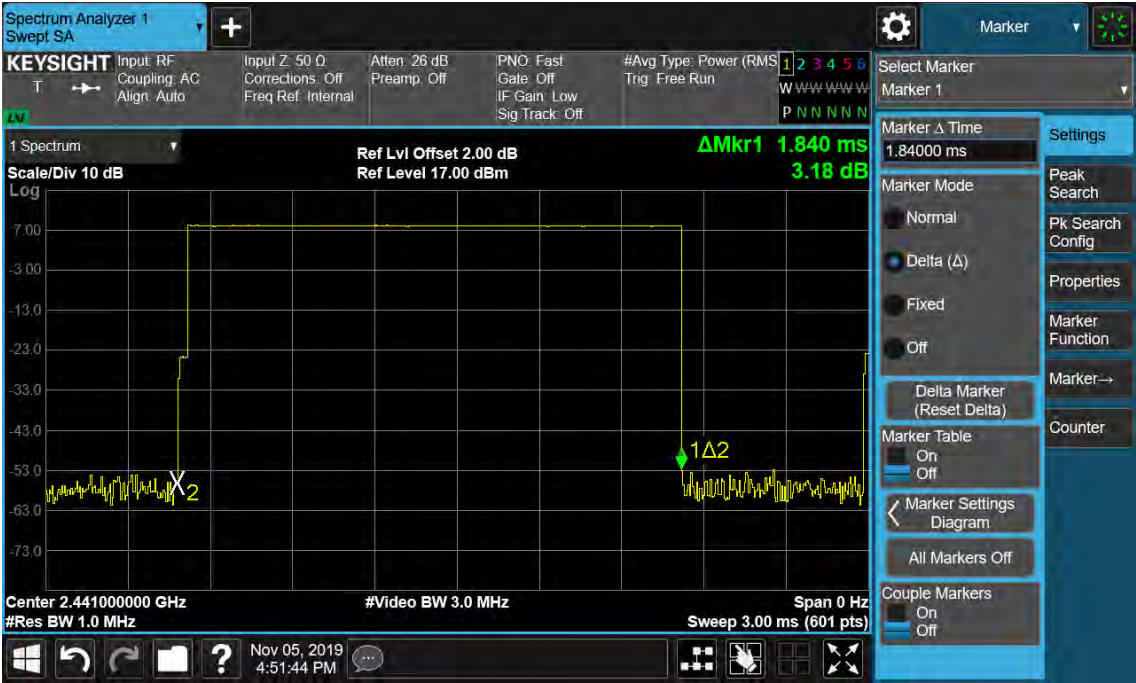
Figure 47: Time of Occupancy, 2441MHz, 8-DPSK DH3
