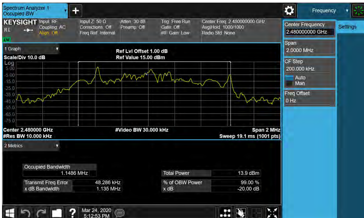
Figure 15: 20dB Bandwidth and 99% Bandwidth, 2480MHz, 8-DPSK
