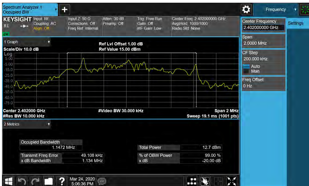
Figure 13: 20dB Bandwidth and 99% Bandwidth, 2402MHz, 8-DPSK
