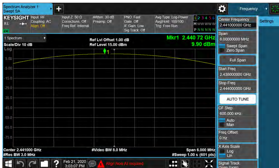
Figure 5: Maximum Conducted Output Power, 2441MHz, \pi/4 -DQPSK
