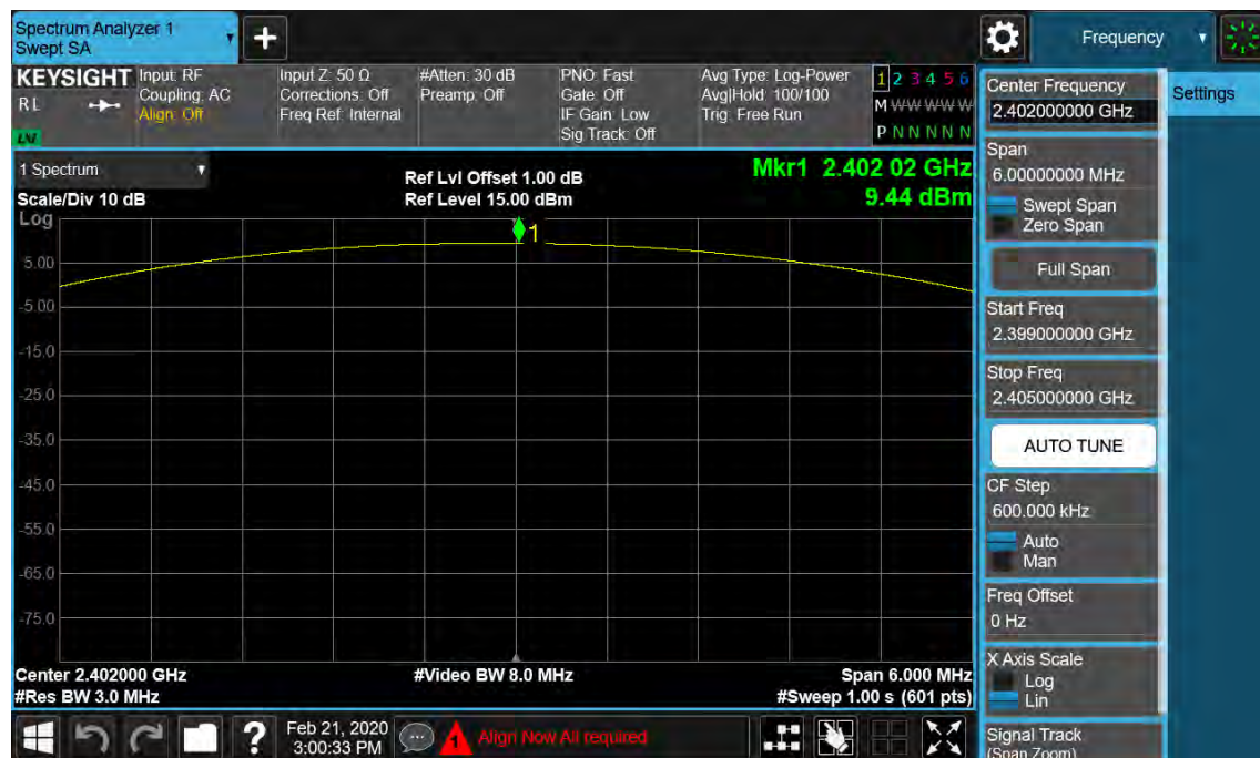
Figure 4: Maximum Conducted Output Power, 2402MHz, \pi/4 -DQPSK
