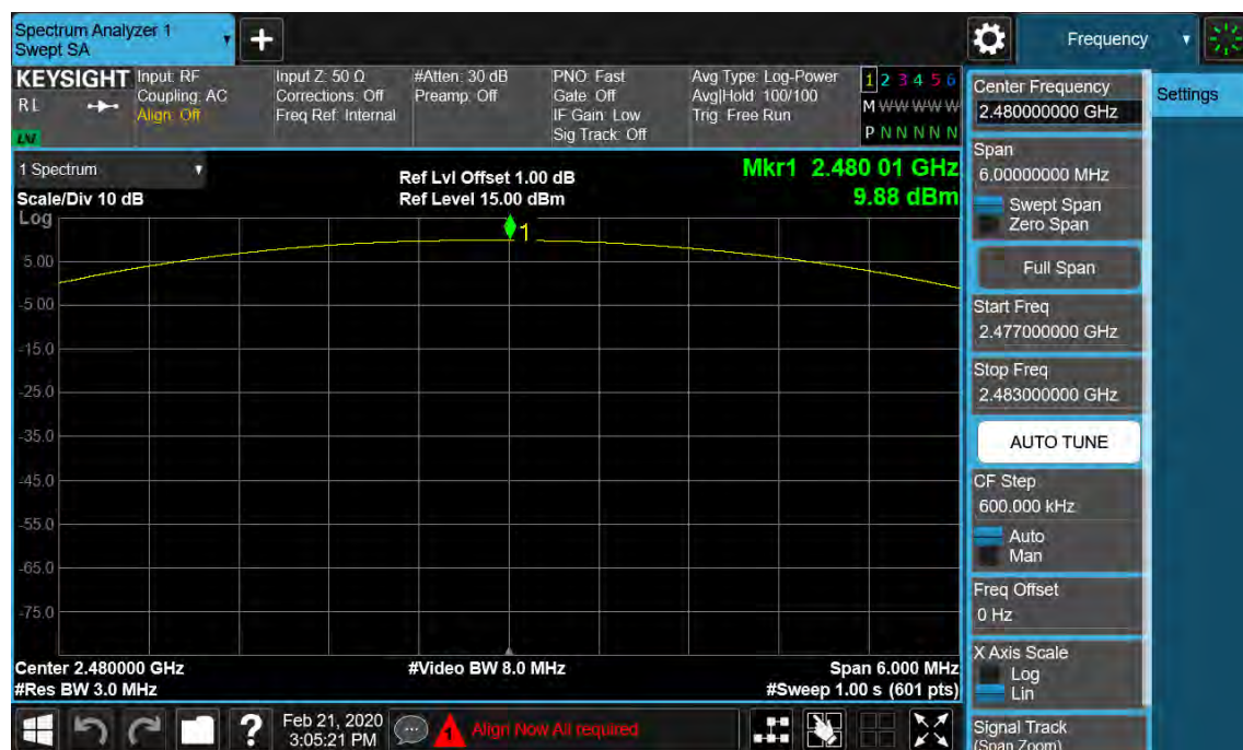
Figure 6: Maximum Conducted Output Power, 2480MHz, \pi/4 -DQPSK
