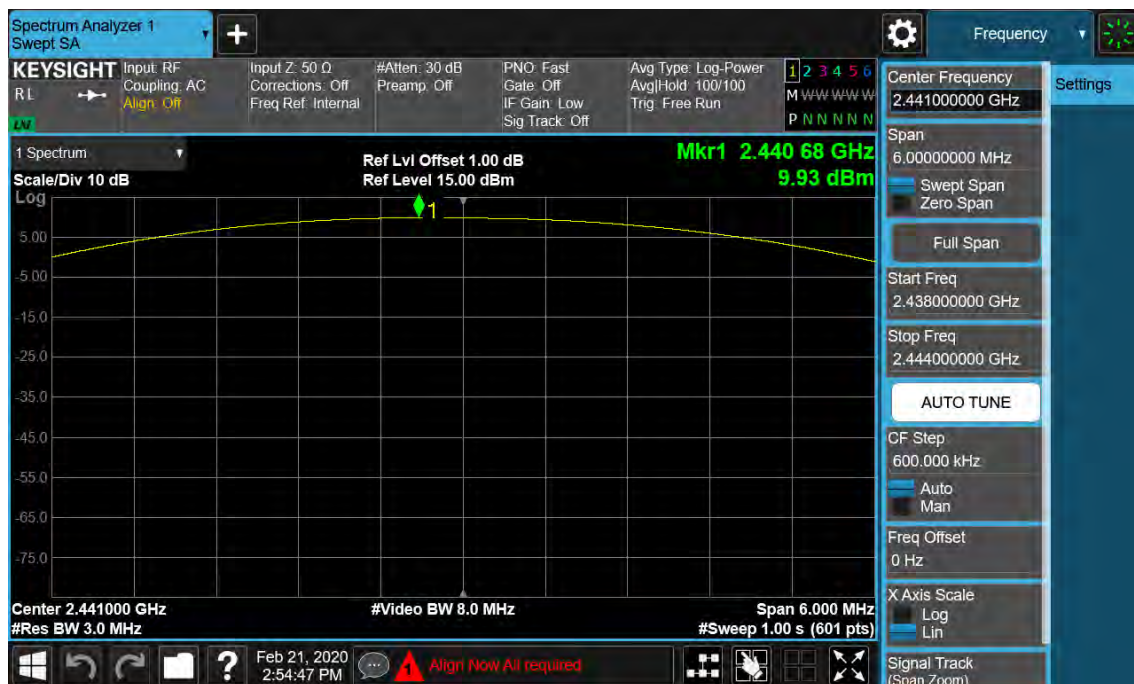
Figure 2: Maximum Conducted Output Power, 2441MHz, GFSK
