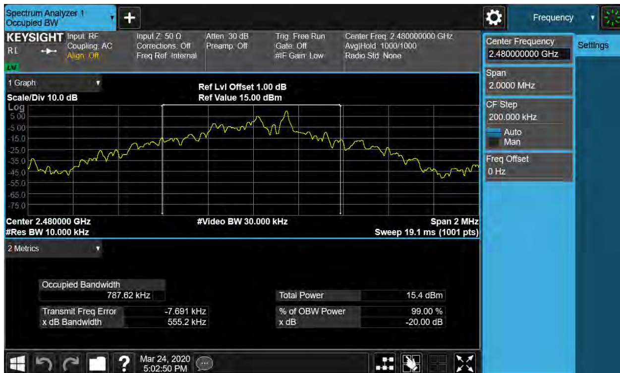
Figure 12: 20dB Bandwidth and 99% Bandwidth, 2480MHz, GFSK
