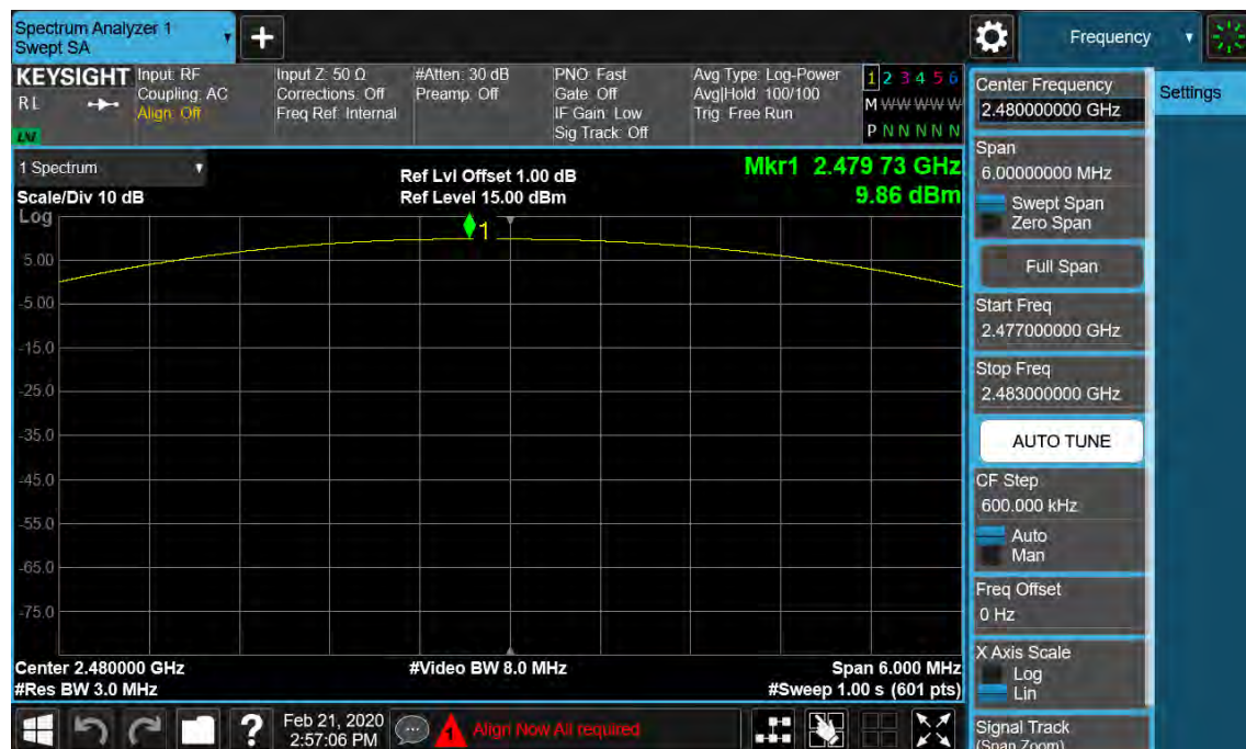
Figure 3: Maximum Conducted Output Power, 2480MHz, GFSK
