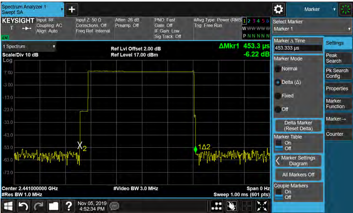
Figure 46: Time of Occupancy, 2441MHz, 8-DPSK DH1
