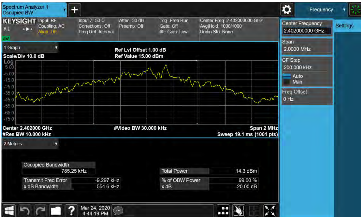
Figure 10: 20dB Bandwidth and 99% Bandwidth, 2402MHz, GFSK
