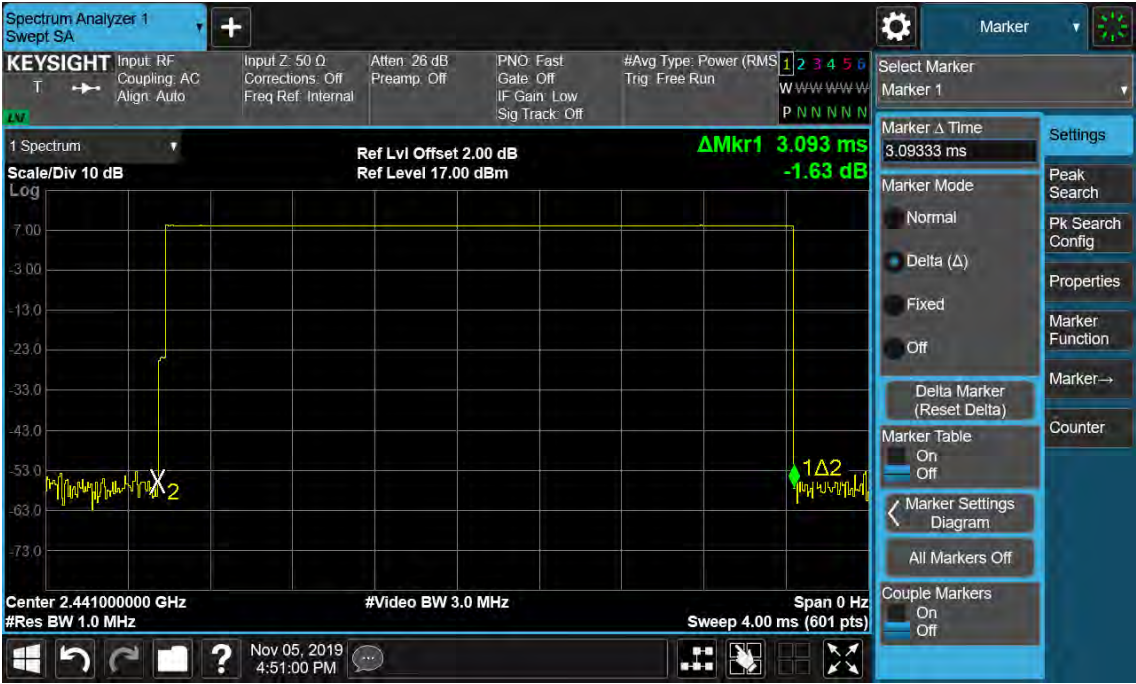
Figure 48: Time of Occupancy, 2441MHz, 8-DPSK DH5
