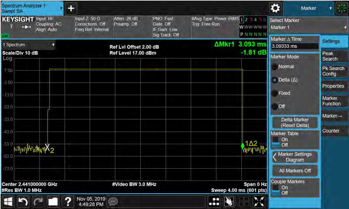
Figure 45: Time of Occupancy, 2441MHz, GFSK DH5
