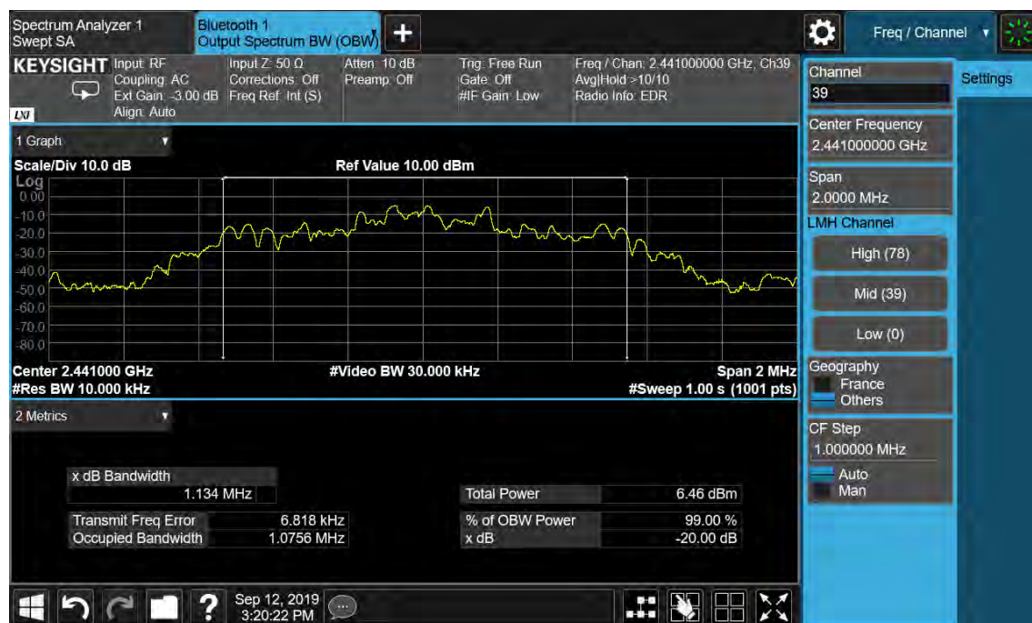
Figure 14: 20dB Bandwidth and 99% Bandwidth, 2441MHz, 8-DPSK
