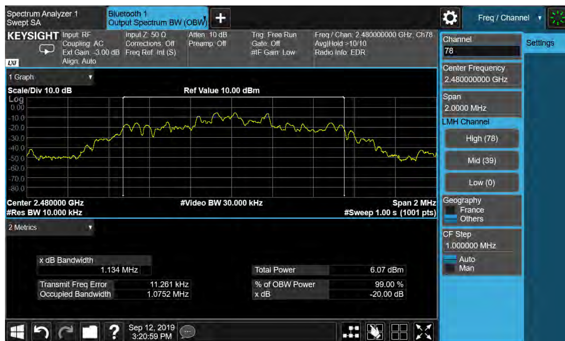
Figure 15: 20dB Bandwidth and 99% Bandwidth, 2480MHz, 8-DPSK
