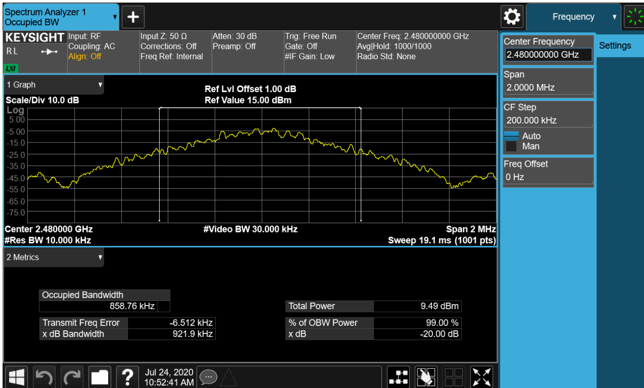
Figure 12: 20dB Bandwidth and 99% Bandwidth, 2480MHz, GFSK
