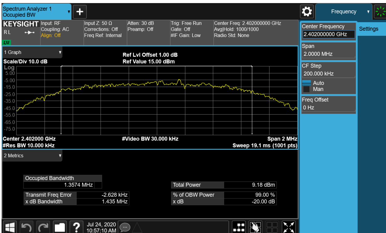
Figure 13: 20dB Bandwidth and 99% Bandwidth, 2402MHz, 8-DPSK
