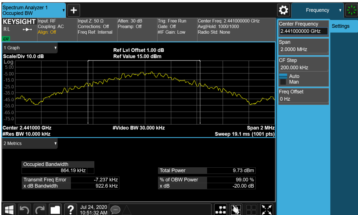
Figure 11: 20dB Bandwidth and 99% Bandwidth, 2441MHz, GFSK
