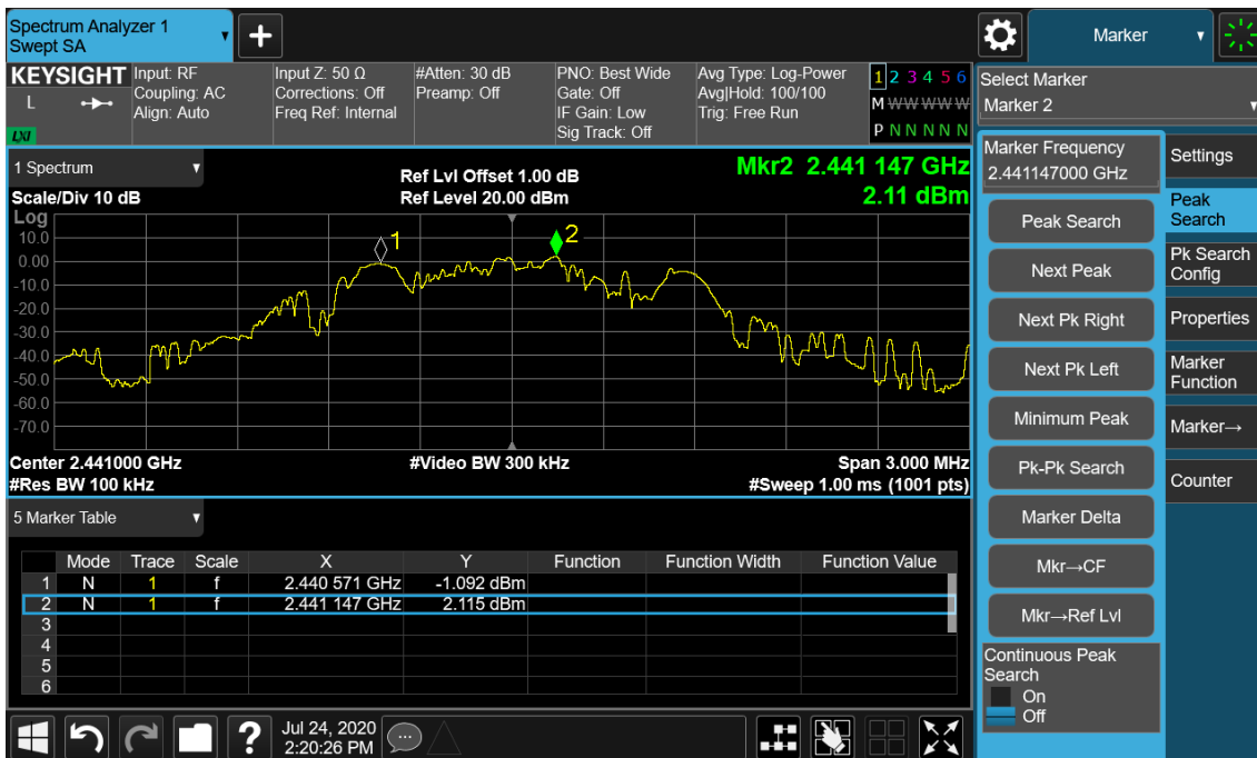
Figure 25: Hopping Frequency Separation, Hopping Mode, 8DPSK
