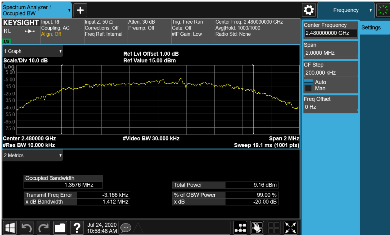
Figure 10: 20dB Bandwidth and 99% Bandwidth, 2402MHz, GFSK
