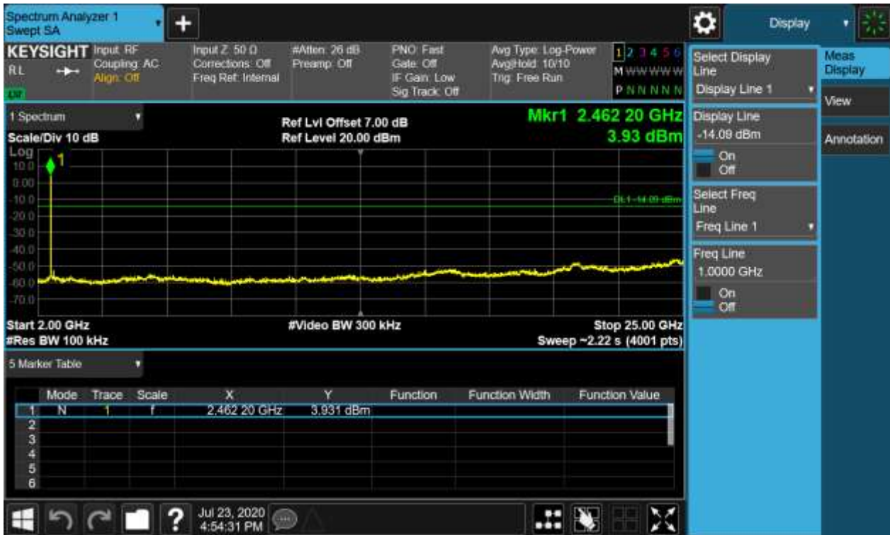
Chain 1 Conducted Spurious Emission & Authorized-band band-edge, 802.11g, 2412MHz Carrier Level
