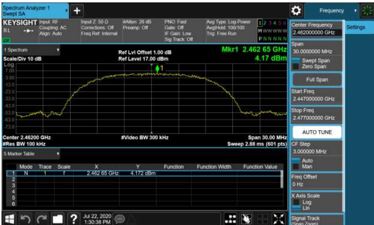
Chain 2 Conducted Spurious Emission & Authorized-band band-edge, 802.11b, 2462MHz Carrier Level
