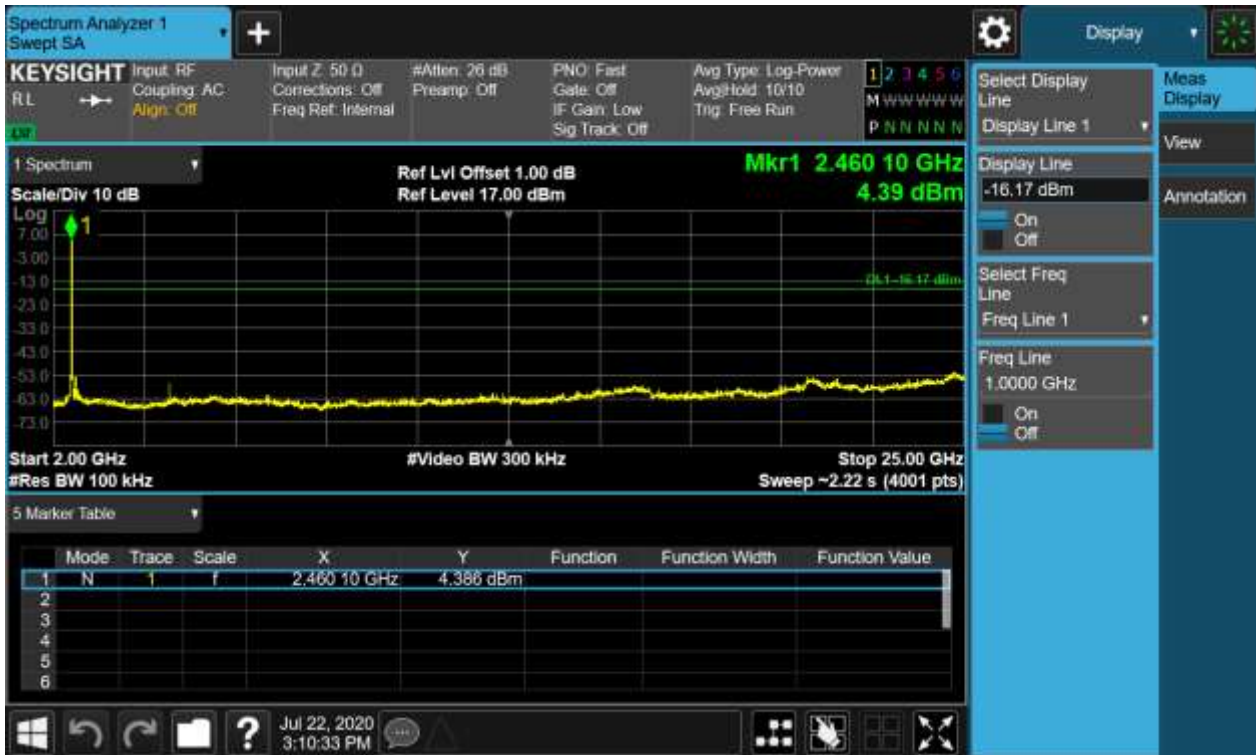
Chain 2 Conducted Spurious Emission & Authorized-band band-edge, 802.11b, 2462MHz Carrier Level
