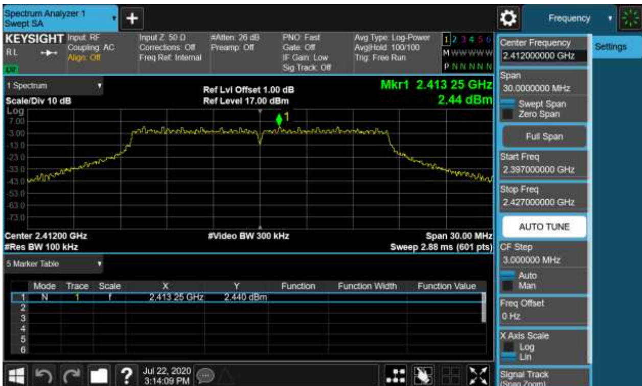
Chain 1 Conducted Spurious Emission & Authorized-band band-edge, 802.11g, 2412MHz Carrier Level
