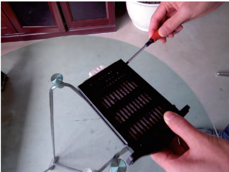
Picture 12: HDD enclosure installation image 1
