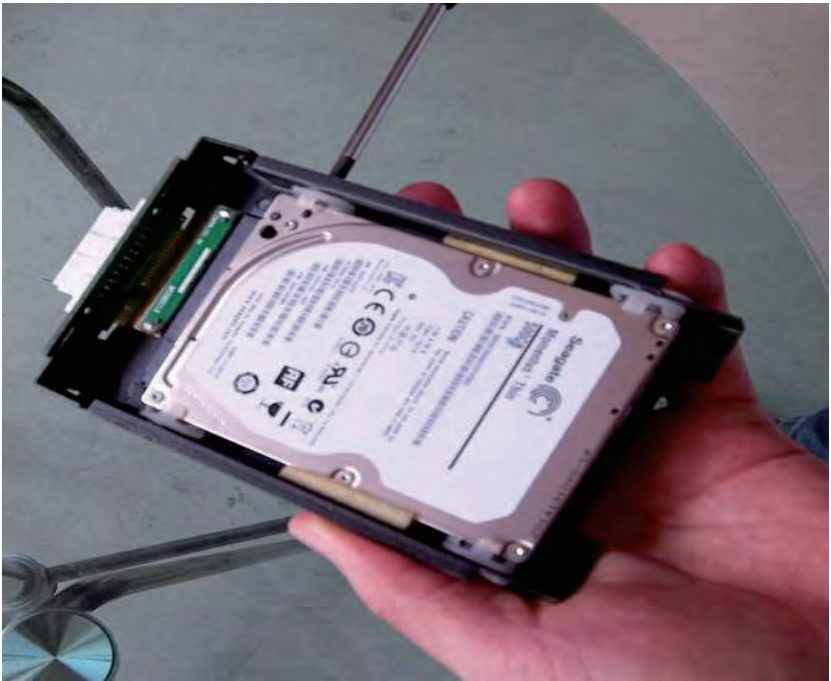
Picture 14: HDD enclosure installation image 3
