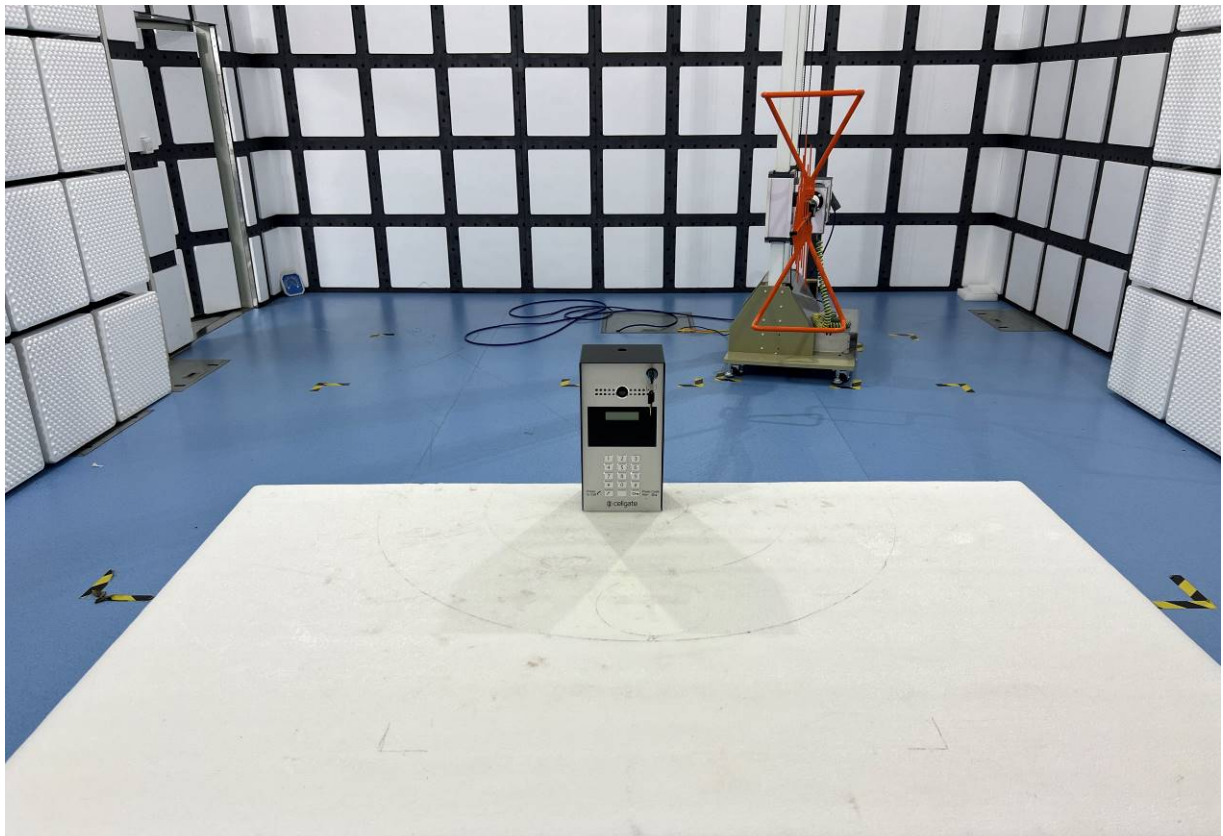
Radiated Emission-Rear View(Below 1GHz)
