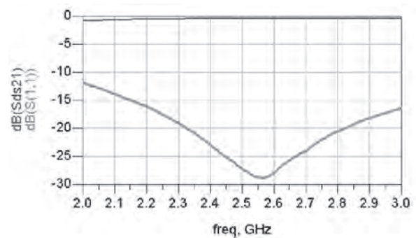
Insertion and Return Loss
