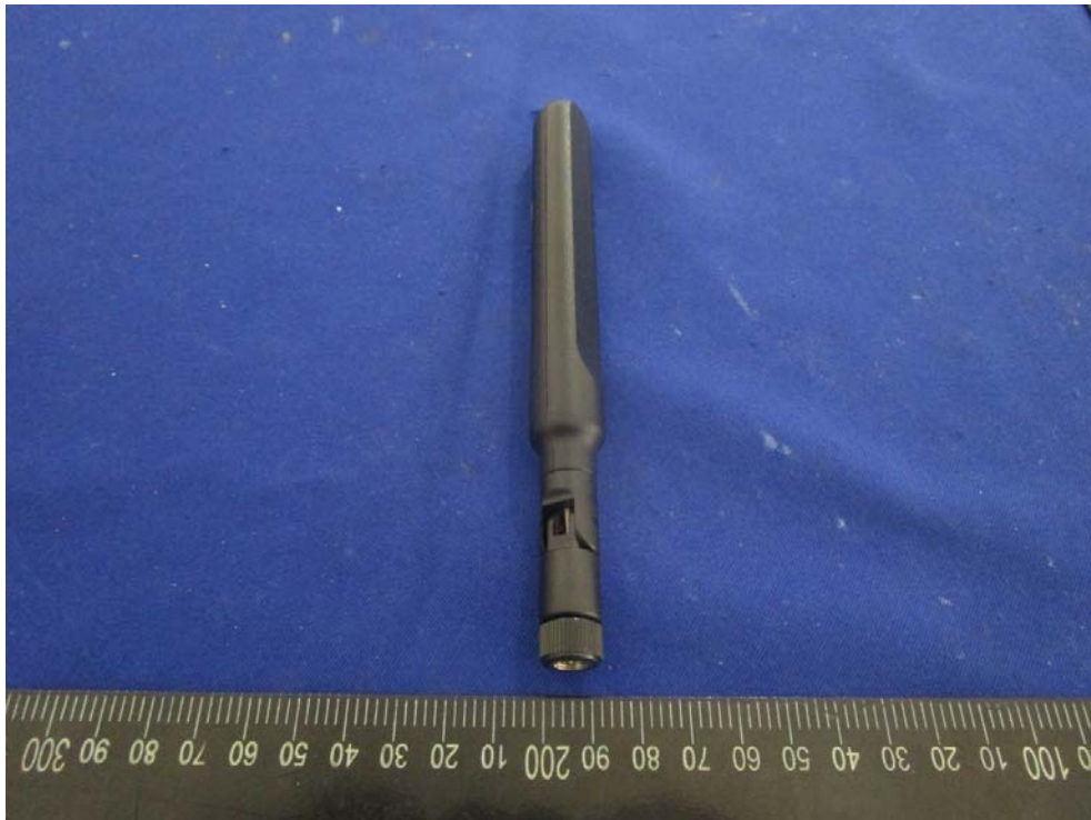
EUT – WLAN ANT View
