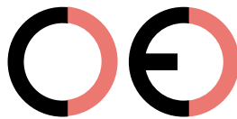
False CE Mark (too far)
