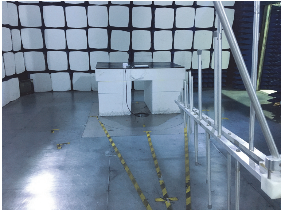
Radiation Emission Test Setup (30MHz to 1GHz)
