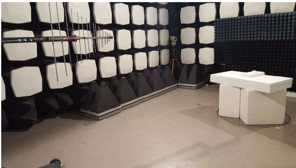
Photo 4 - Radiated emission test setup for 200 - 1000 MHz.
