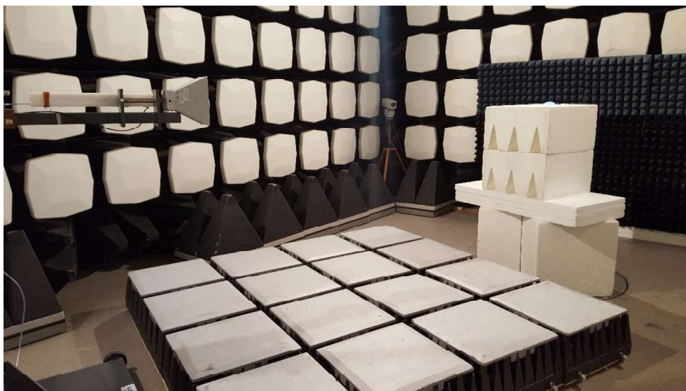
Photo 5 - Radiated emission test setup for 1 – 14 GHz.
