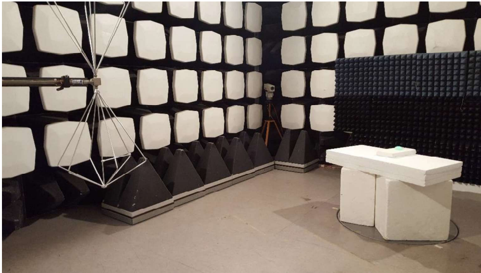
Photo 3 - Radiated emission test setup for 30 - 200 MHz.
