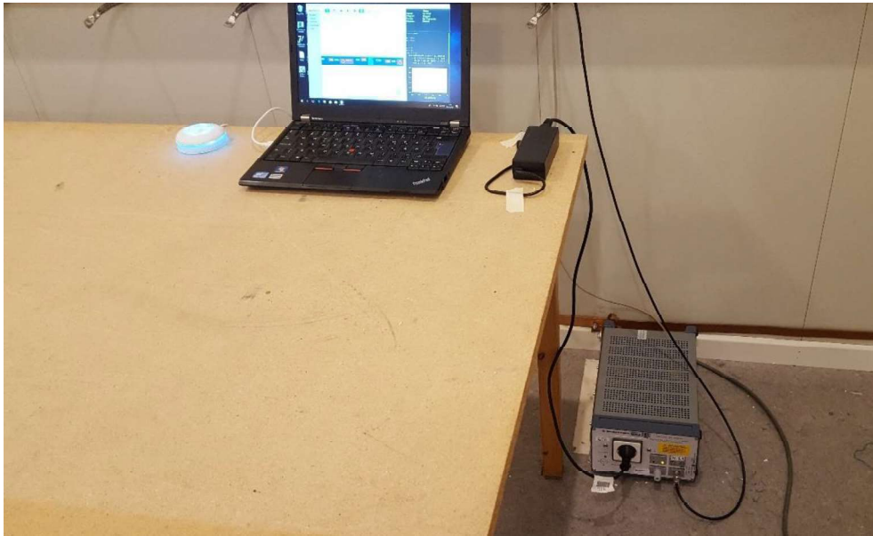
Photo 10. AC Conducted emission test set up. Powered by laptop
