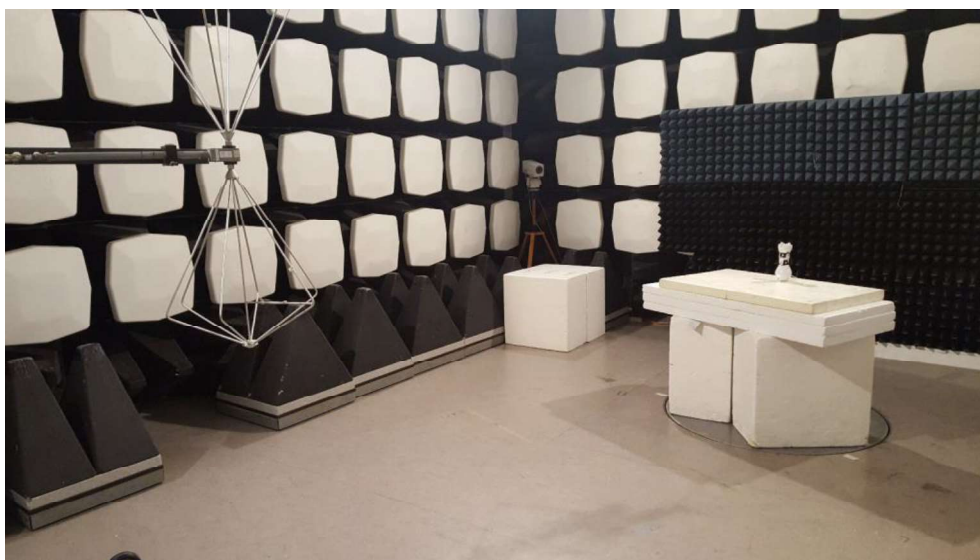
Photo 4 - Radiated emission test setup for 30 - 200 MHz.
