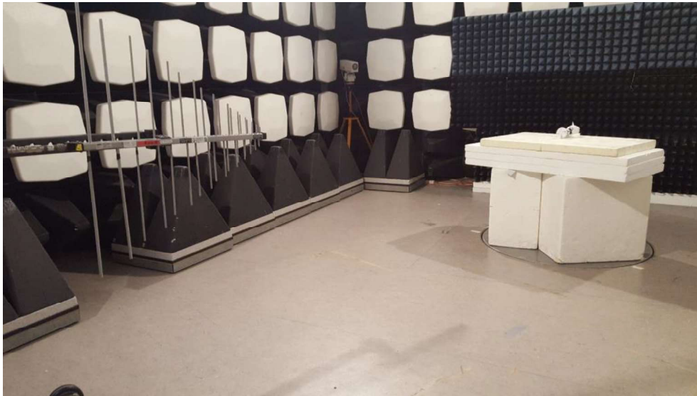
Photo 5 - Radiated emission test setup for 200 - 1000 MHz.
