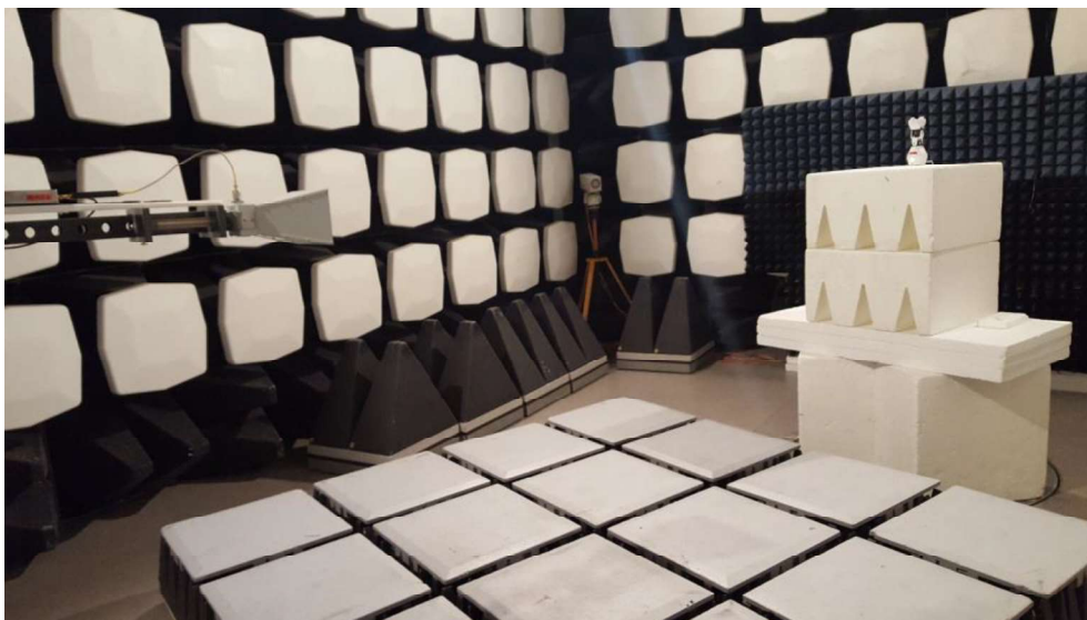
Photo 6 - Radiated emission test setup for 1 – 14 GHz.
