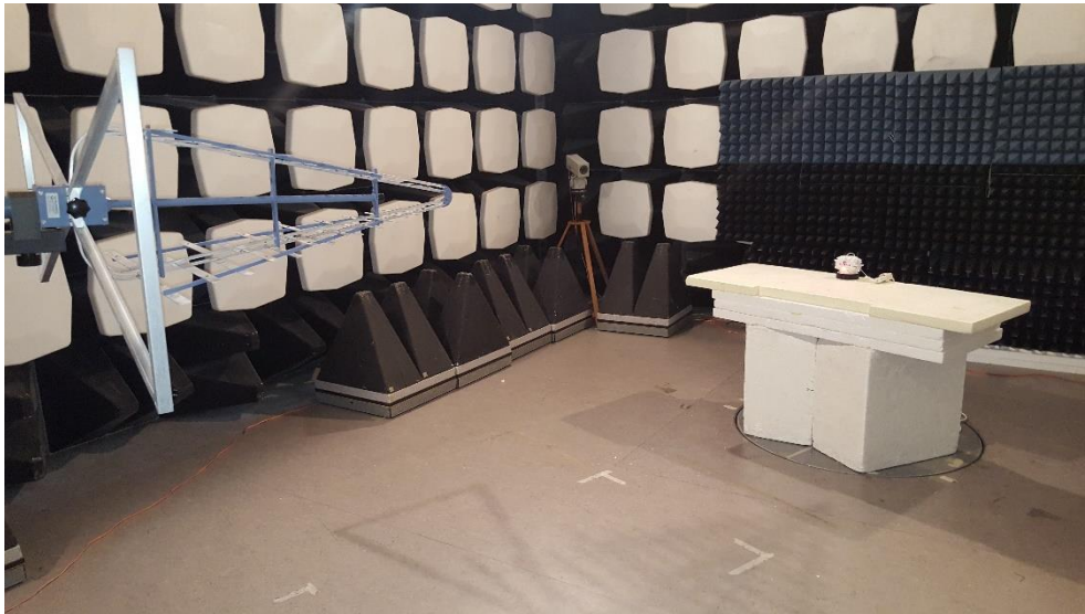
Photo 3 - Radiated emission test setup for 30 - 1000 MHz.
