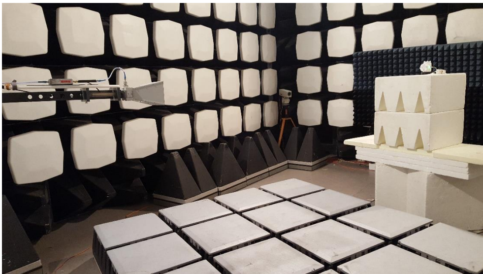
Photo 4 - Radiated emission test setup for 1 - 14 GHz.
