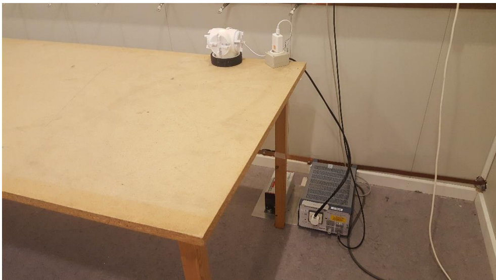
Photo 6. AC Conducted emission test set up.
