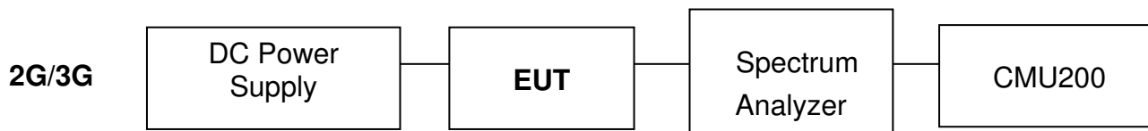
Fig. 2-1 Configuration of Tested System (Fixed Channel-Conducted)
