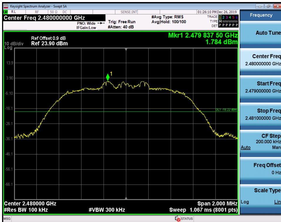
RF Conducted Spurious Emissions_2DH5_2480
