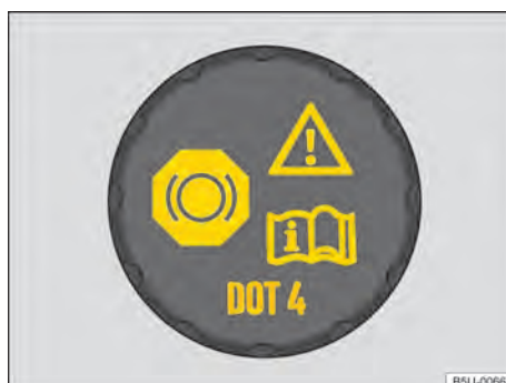
Fig. 192 On the engine compartment: brake fluid reservoir cap.
