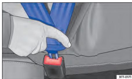
Fig. 27 Inserting the seat belt latch plate into the buckle.
