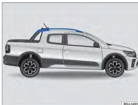
Fig. 157 Roof rack longitudinal supports (both sides).
