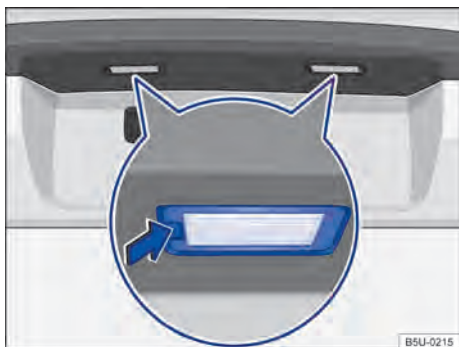
Fig. 173 On the rear bumper: remove the number plate light.
