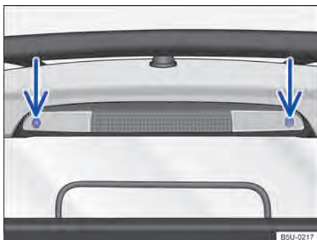
Fig. 175 On the bed: remove the elevated brake light.
