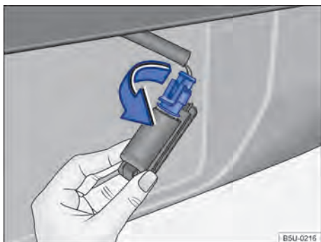
Fig. 174 Number plate light: remove the bulb socket.
