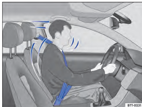
Fig. 26 Driver restrained by a properly positioned seat belt during a sudden braking manoeuvre.
