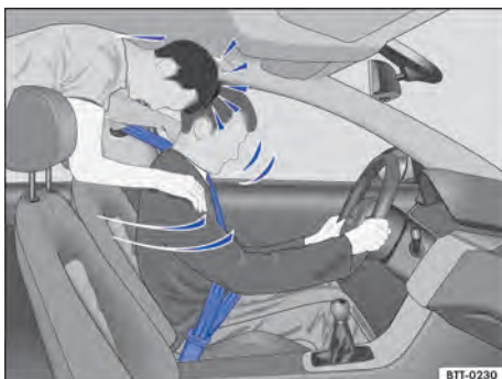
Fig. 25 The unbelted rear passenger is thrown forward violently, hitting the belted driver.
