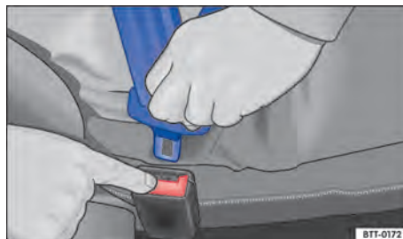
Fig. 28 Removing the seat belt latch plate into the buckle.
