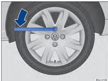
Fig. 204 Changing the wheel: loosen wheel bolts.
