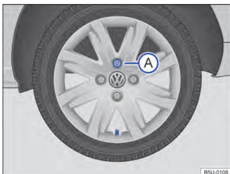
Fig. 207 Wheel replacement: wheel bolt removal sequence.
