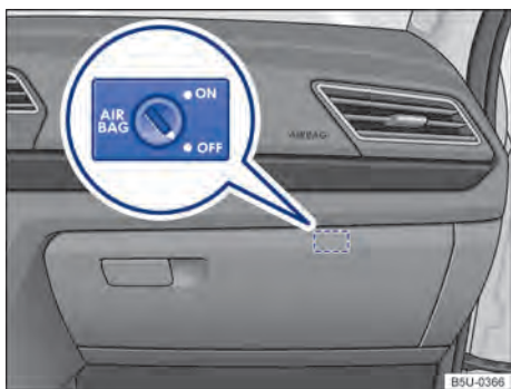
Fig. 35 On the stowage compartment: switch deactivated by the key to switch the passenger front airbag on and off.
