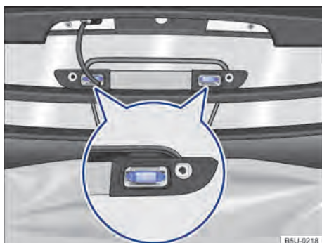
Fig. 176 Elevated brake light: remove the bulb from the bed light.
