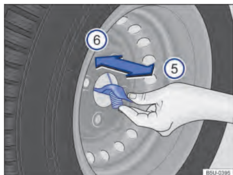
Fig. 200 On the spare wheel: remove the spare wheel cable.
