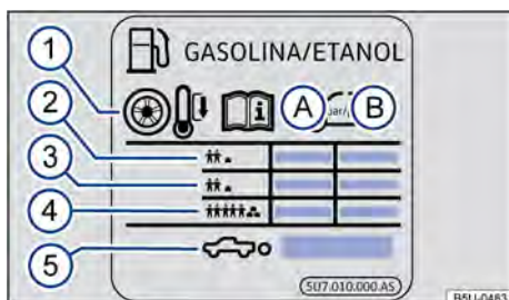
Fig. 196 Sticker with the tyre pressures.
