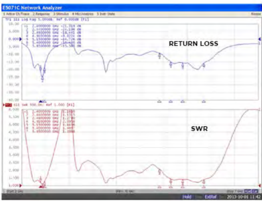
Bent Antenna Position
