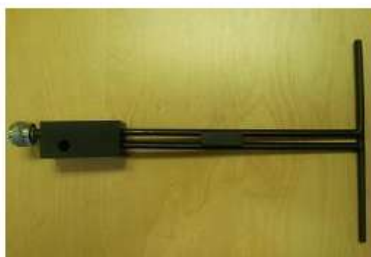
Figure 1 – MVG COMOSAR Validation Dipole
