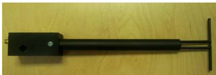
Figure 1 – MVG COMOSAR Validation Dipole
