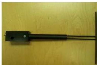
Figure 1 – MVG COMOSAR Validation Dipole
