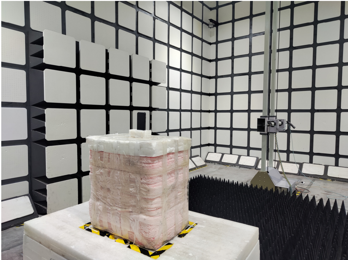
Radiated Emissions View (18-40 GHz)
