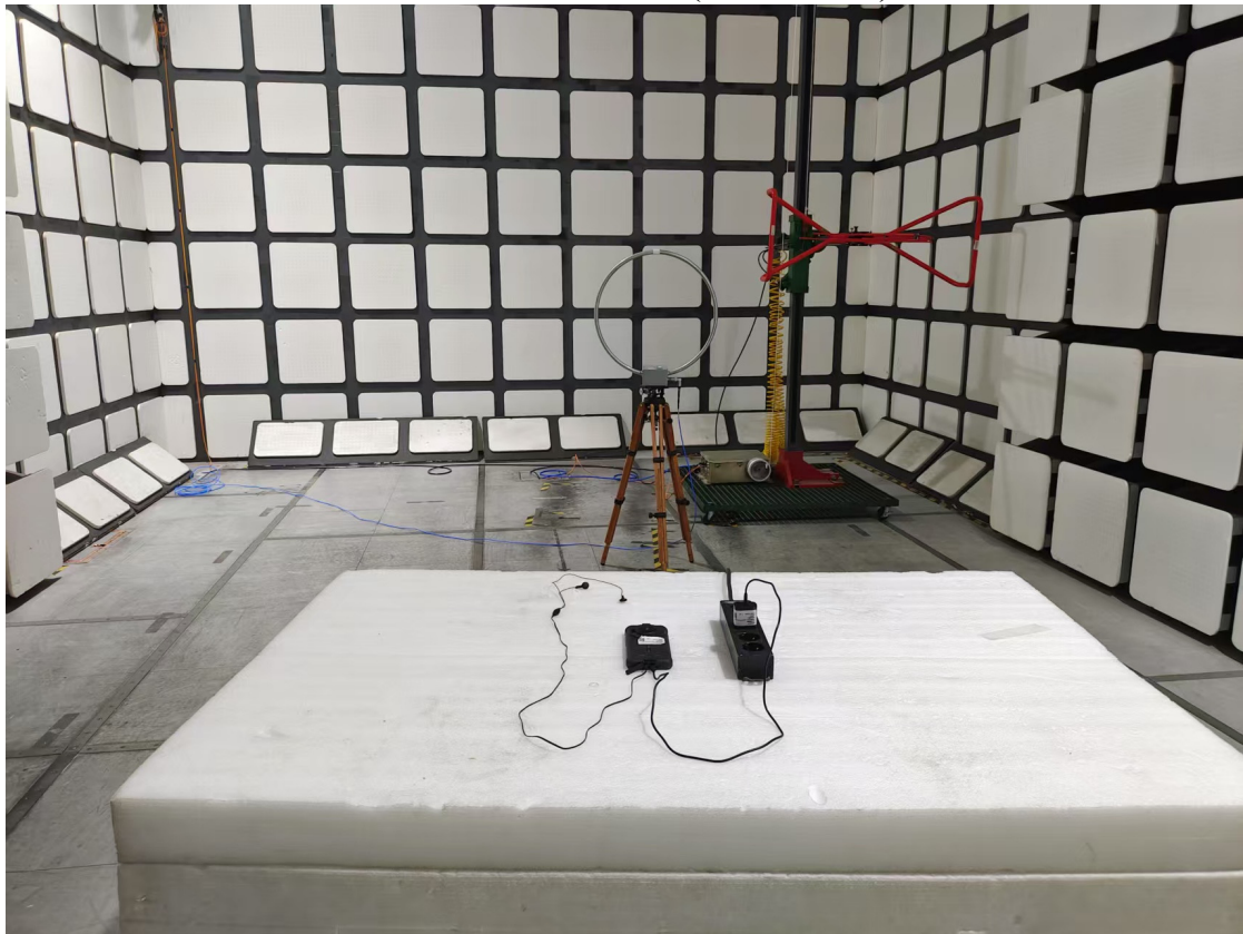
Radiated Emissions View (Below 1 GHz)
