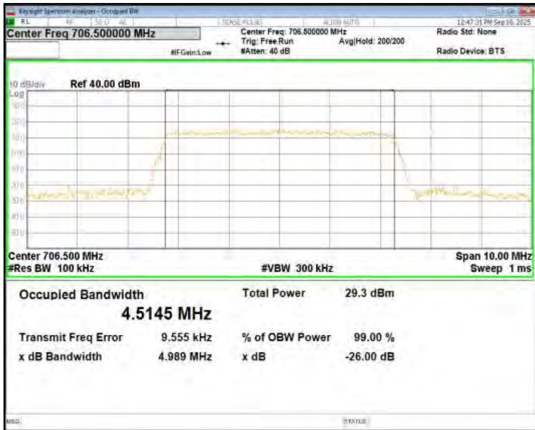
Band17 16QAM BW=5MHz Channel=23790 RB Size=25 Position=#0
