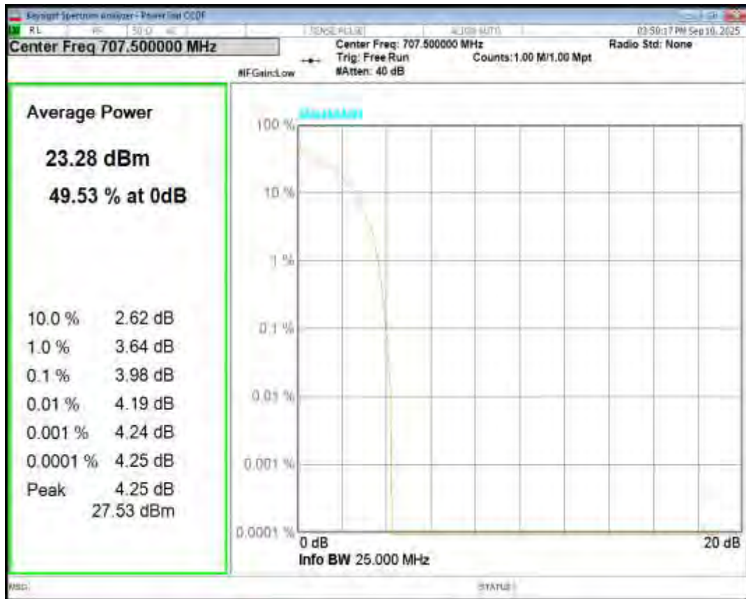
Band12 QPSK BW=1.4MHz Channel=23173 RB Size=1 Position=#0
