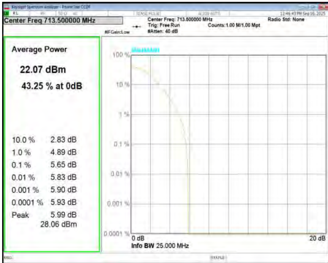
Band17 QPSK BW=10MHz Channel=23780 RB Size=1 Position=#0
