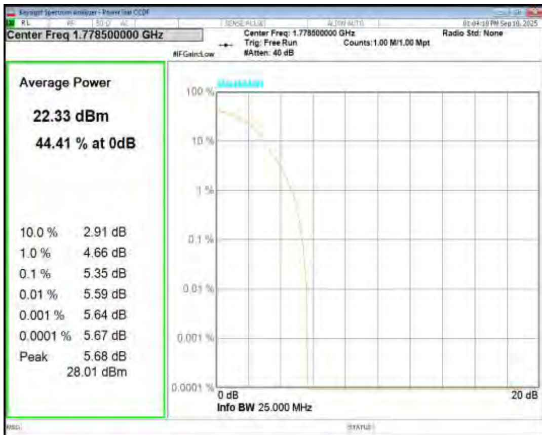
Band66 16QAM BW=5MHz Channel=131997 RB Size=1 Position=#0
