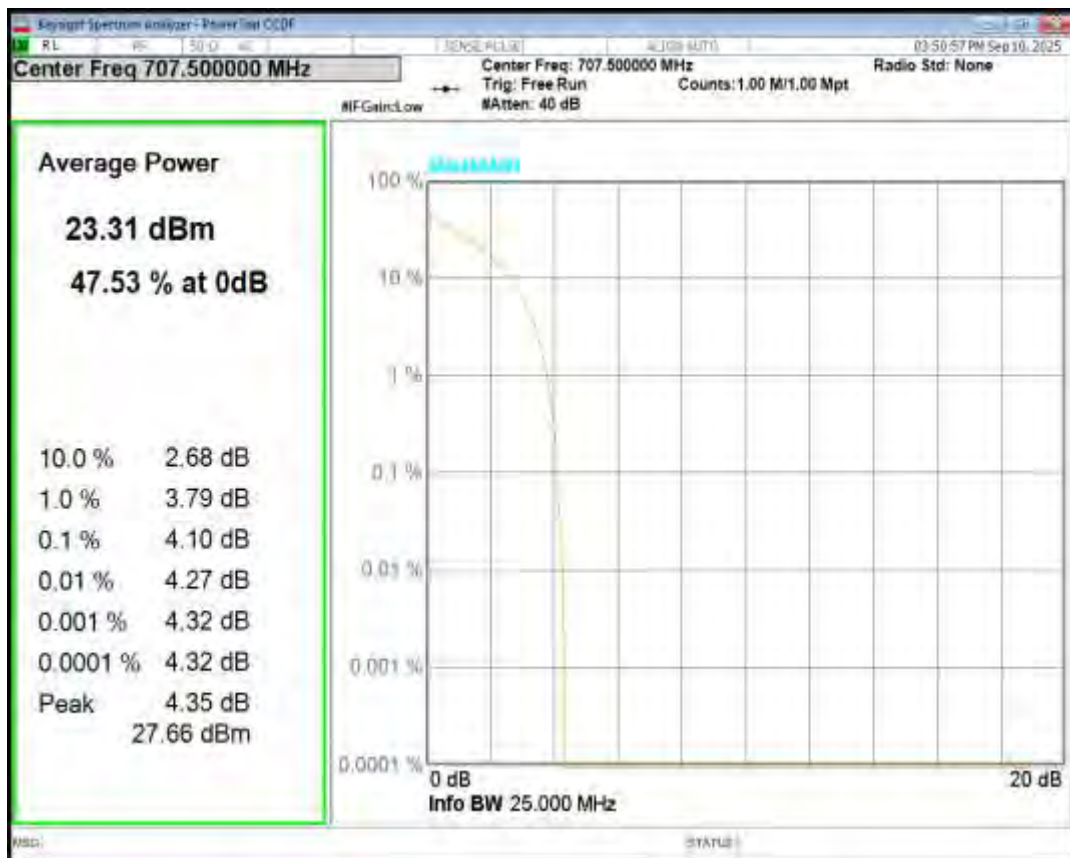
Band12 QPSK BW=5MHz Channel=23155 RB Size=1 Position=#0
