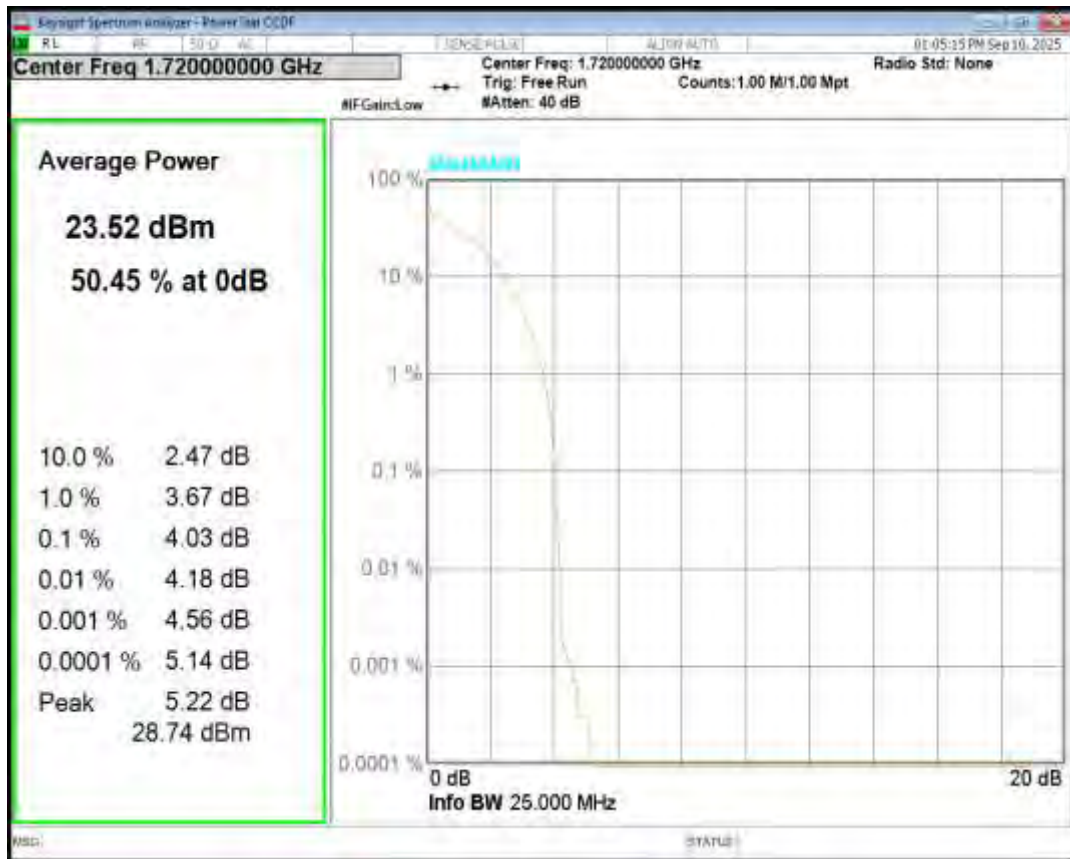
Band66 QPSK BW=20MHz Channel=132322 RB Size=1 Position=#0
