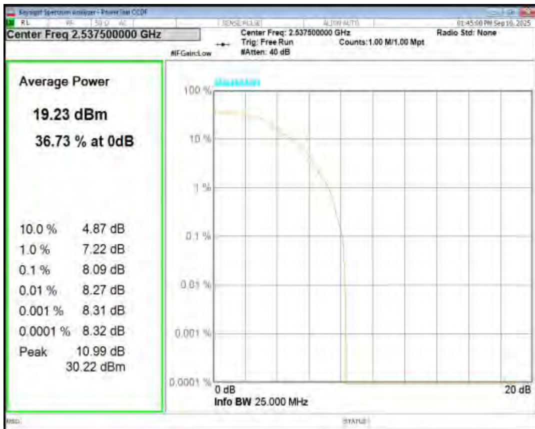
Band41(2535-2655) QPSK BW=5MHz Channel=41215 RB Size=1 Position=#0
