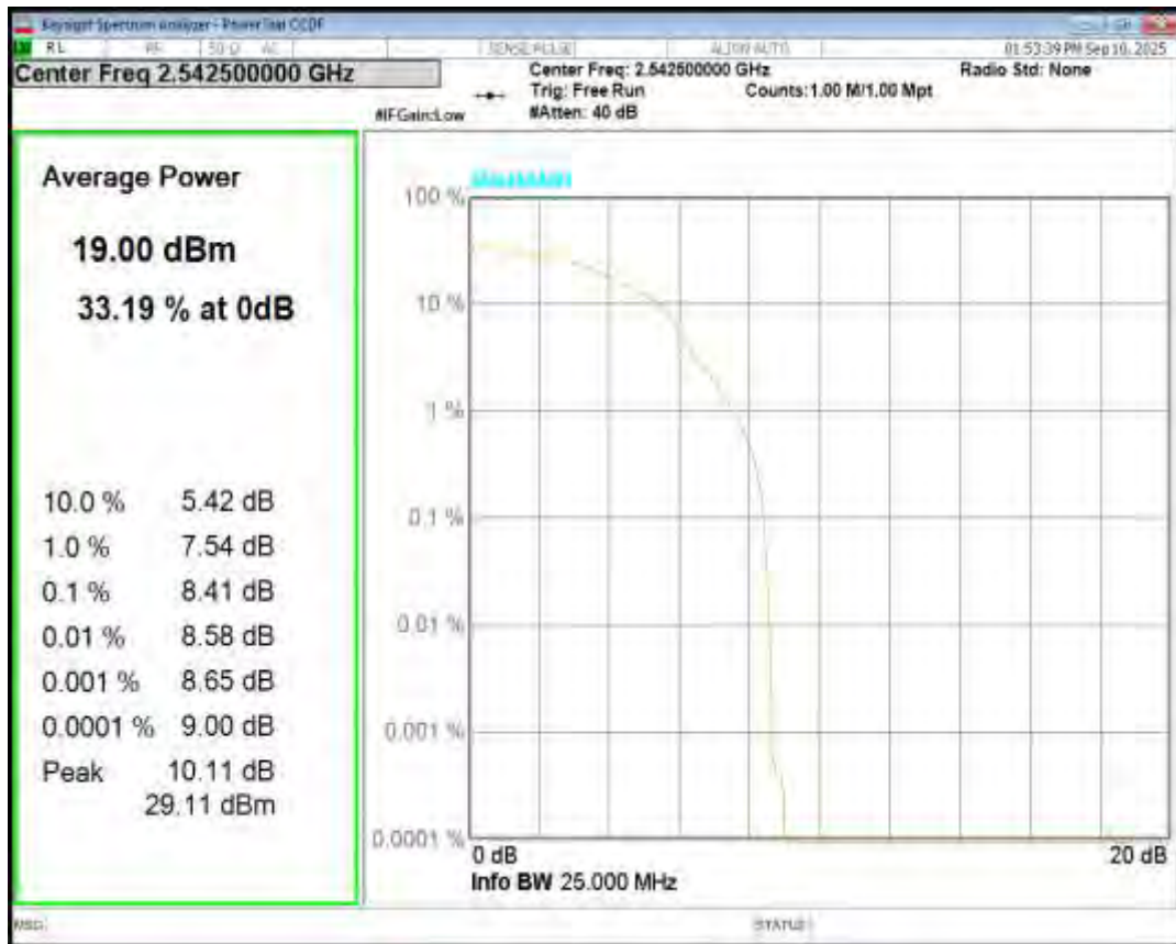
Band41(2535-2655) 16QAM BW=15MHz Channel=40640 RB Size=1 Position=#0
