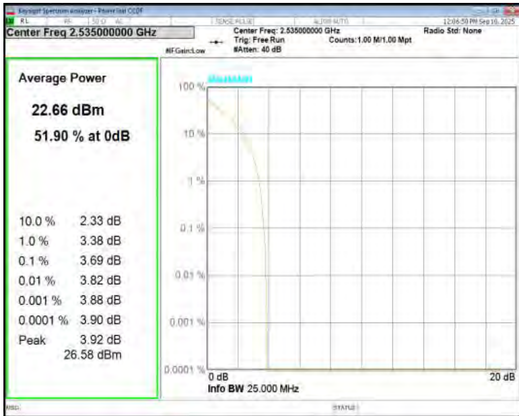
Band7 QPSK BW=10MHz Channel=21400 RB Size=1 Position=#0
