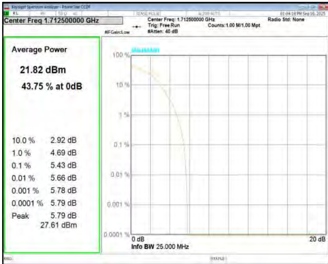
Band66 16QAM BW=5MHz Channel=132322 RB Size=1 Position=#0
