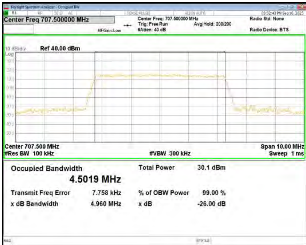
Band12 QPSK BW=5MHz Channel=23155 RB Size=25 Position=#0
