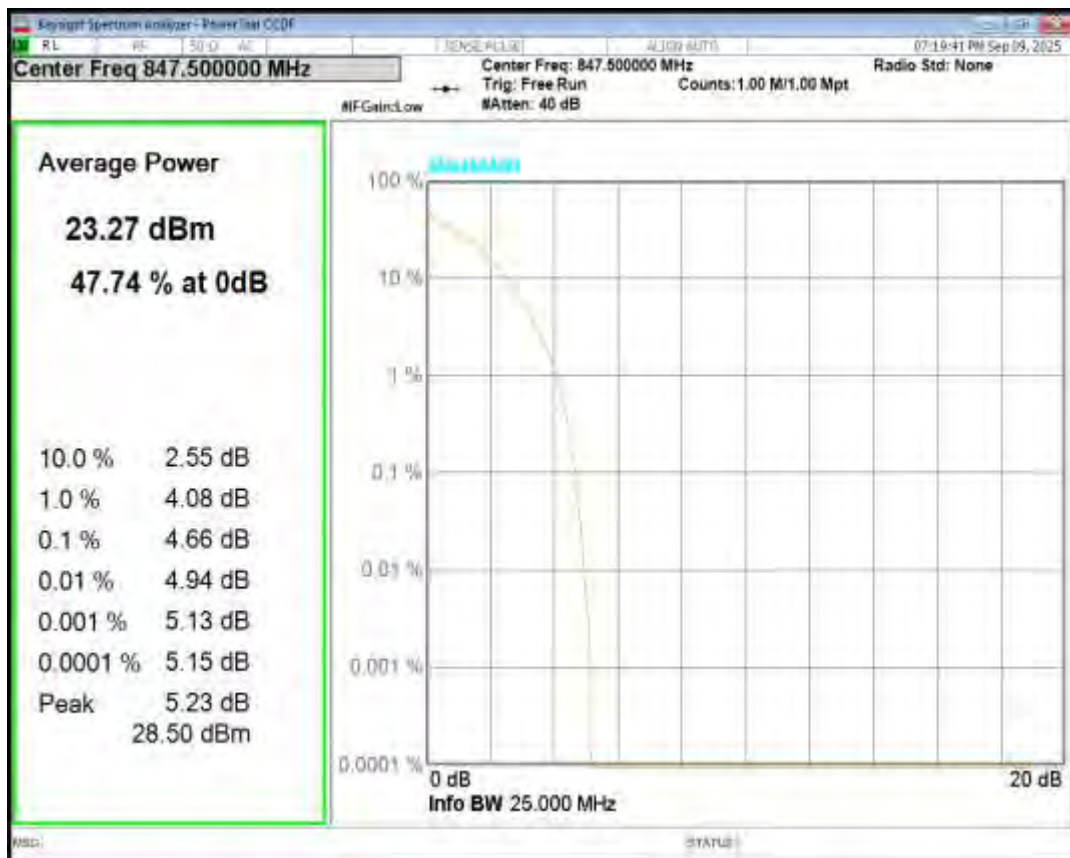
Band5 QPSK BW=5MHz Channel=20425 RB Size=1 Position=#0
