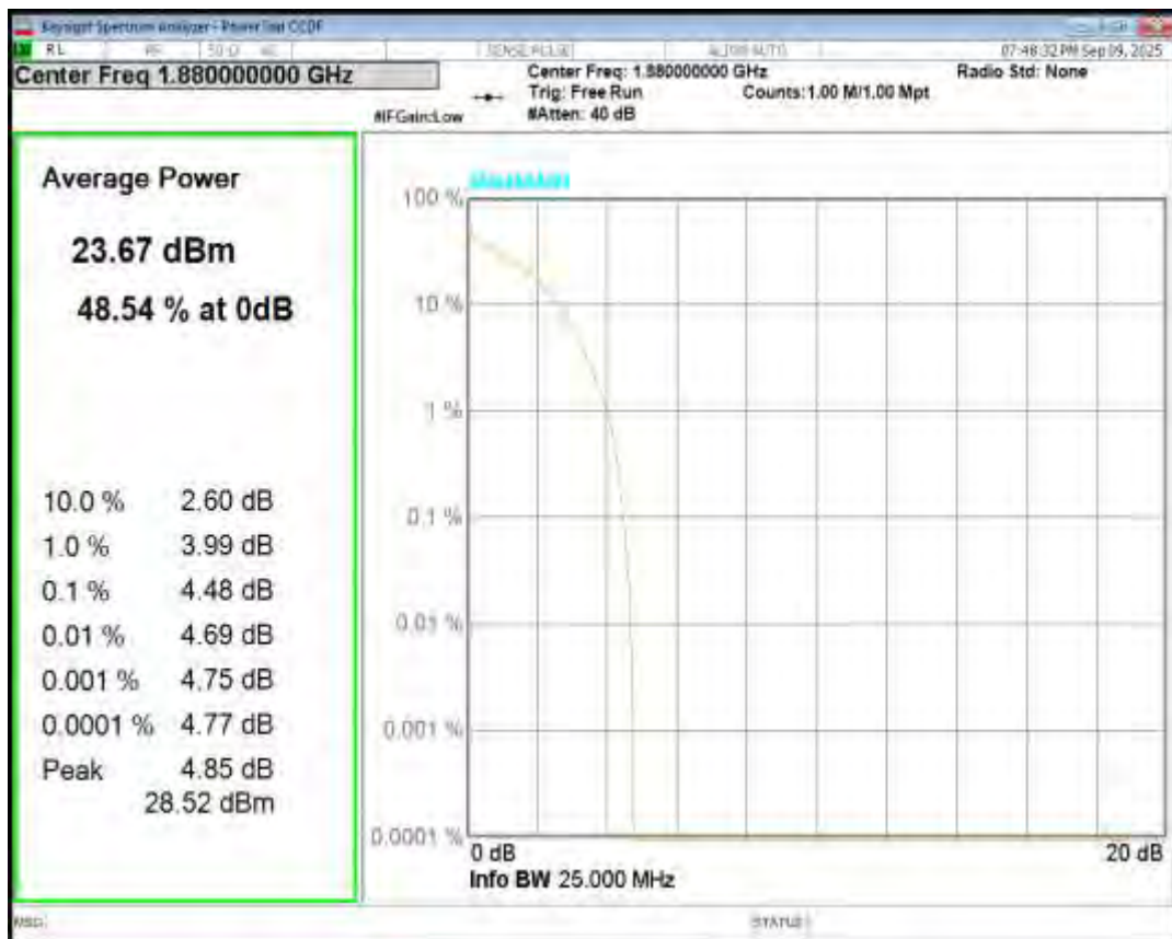
Band2 QPSK BW=10MHz Channel=19150 RB Size=1 Position=#0
