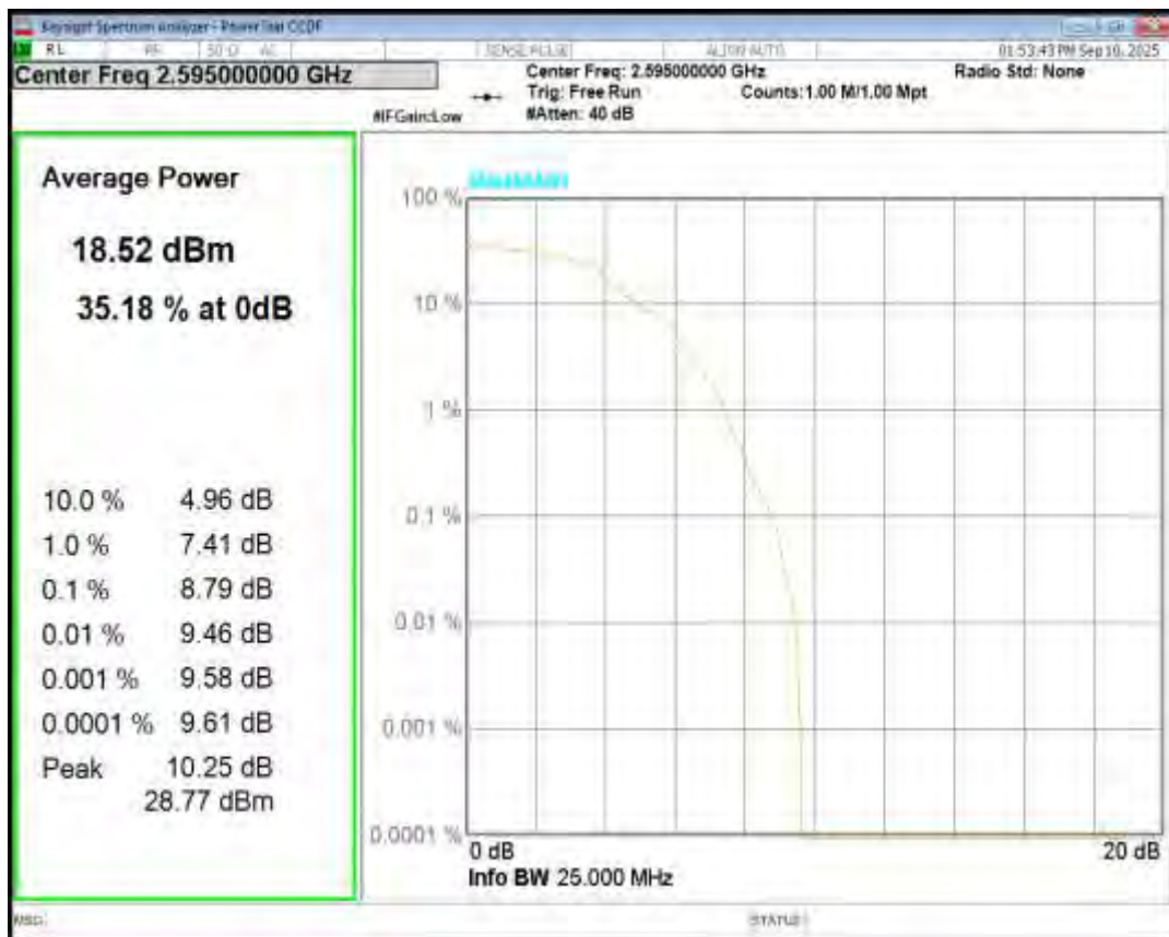
Band41(2535-2655) QPSK BW=15MHz Channel=41165 RB Size=1 Position=#0
