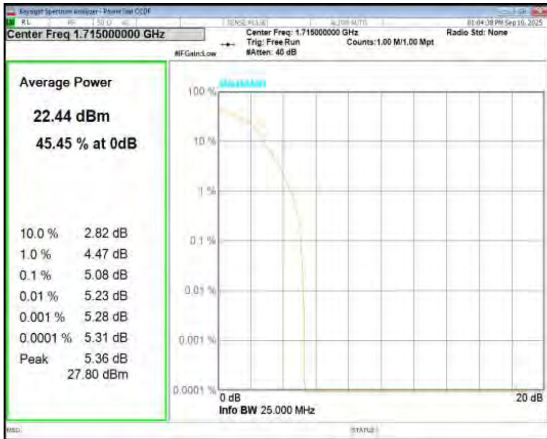
Band66 16QAM BW=10MHz Channel=132322 RB Size=1 Position=#0
