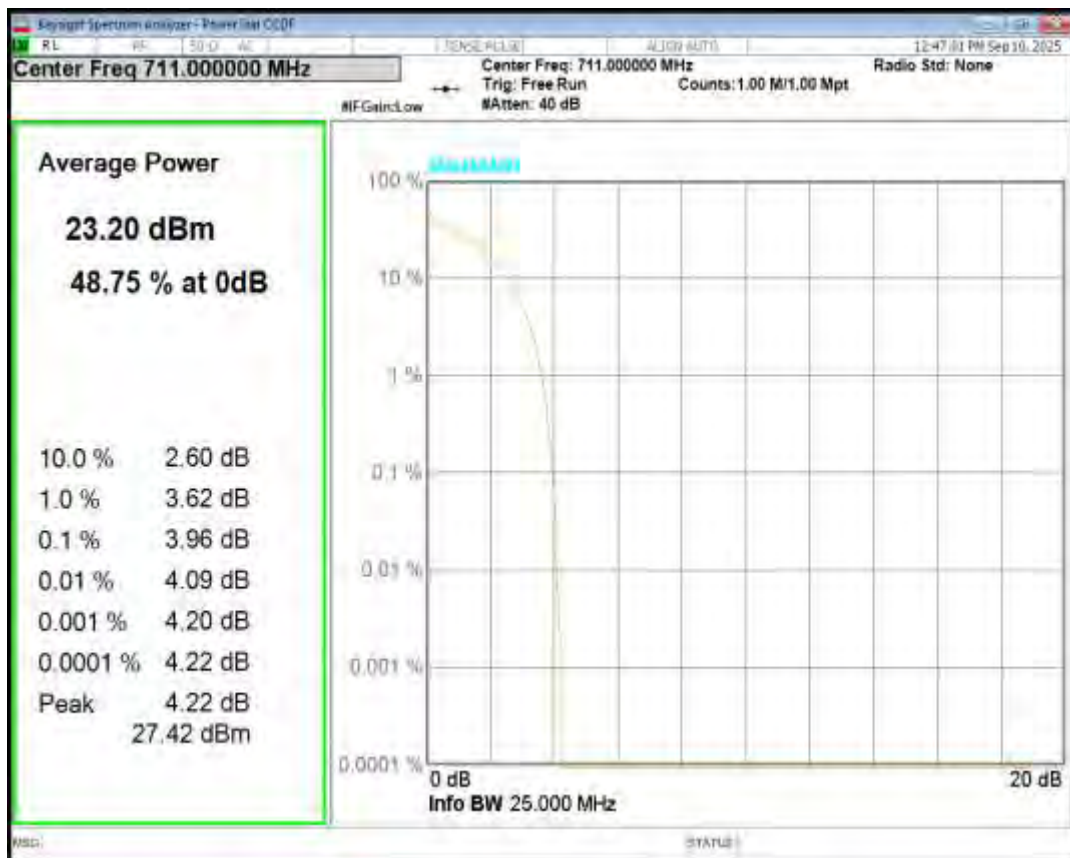
Band17 QPSK BW=5MHz Channel=23755 RB Size=1 Position=#0
