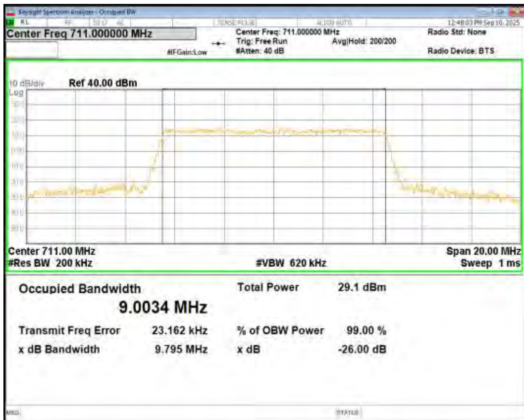
Band17 16QAM BW=5MHz Channel=23755 RB Size=25 Position=#0
