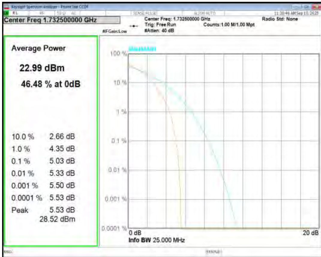
Band4 QPSK BW=3MHz Channel=20385 RB Size=1 Position=#0
