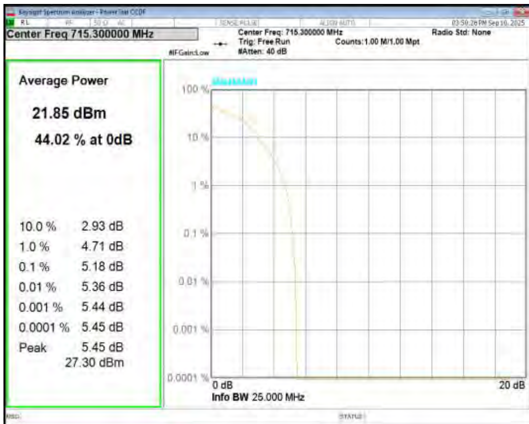
Band12 16QAM BW=10MHz Channel=23060 RB Size=1 Position=#0
