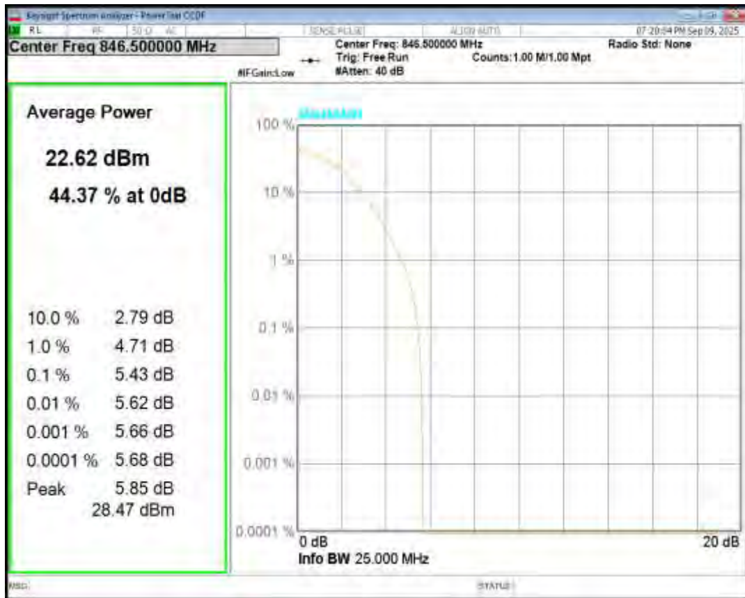
Band5 16QAM BW=5MHz Channel=20525 RB Size=1 Position=#0
