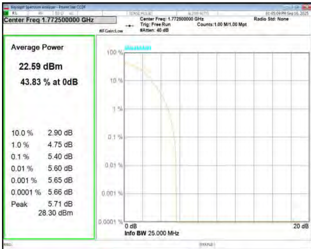
Band66 16QAM BW=20MHz Channel=132072 RB Size=1 Position=#0
