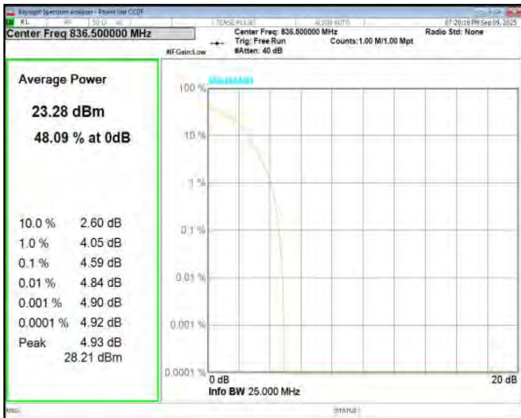
Band5 QPSK BW=10MHz Channel=20600 RB Size=1 Position=#0
