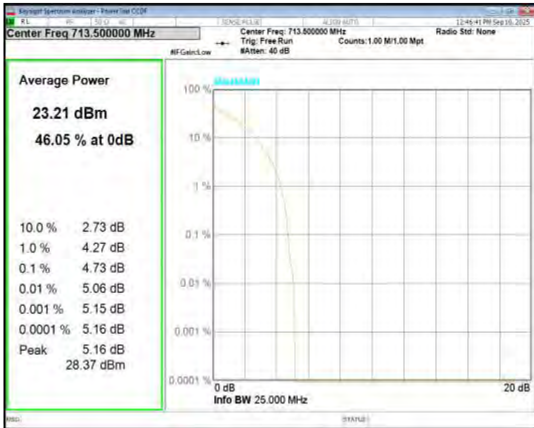
Band2 16QAM BW=1.4MHz Channel=18607 RB Size=1 Position=#0
