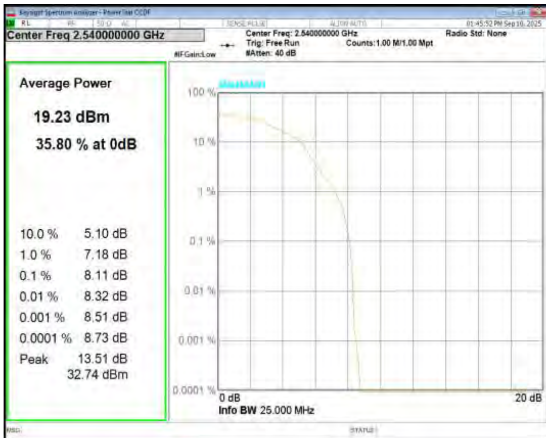
Band41(2535-2655) 16QAM BW=10MHz Channel=40640 RB Size=1 Position=#0
