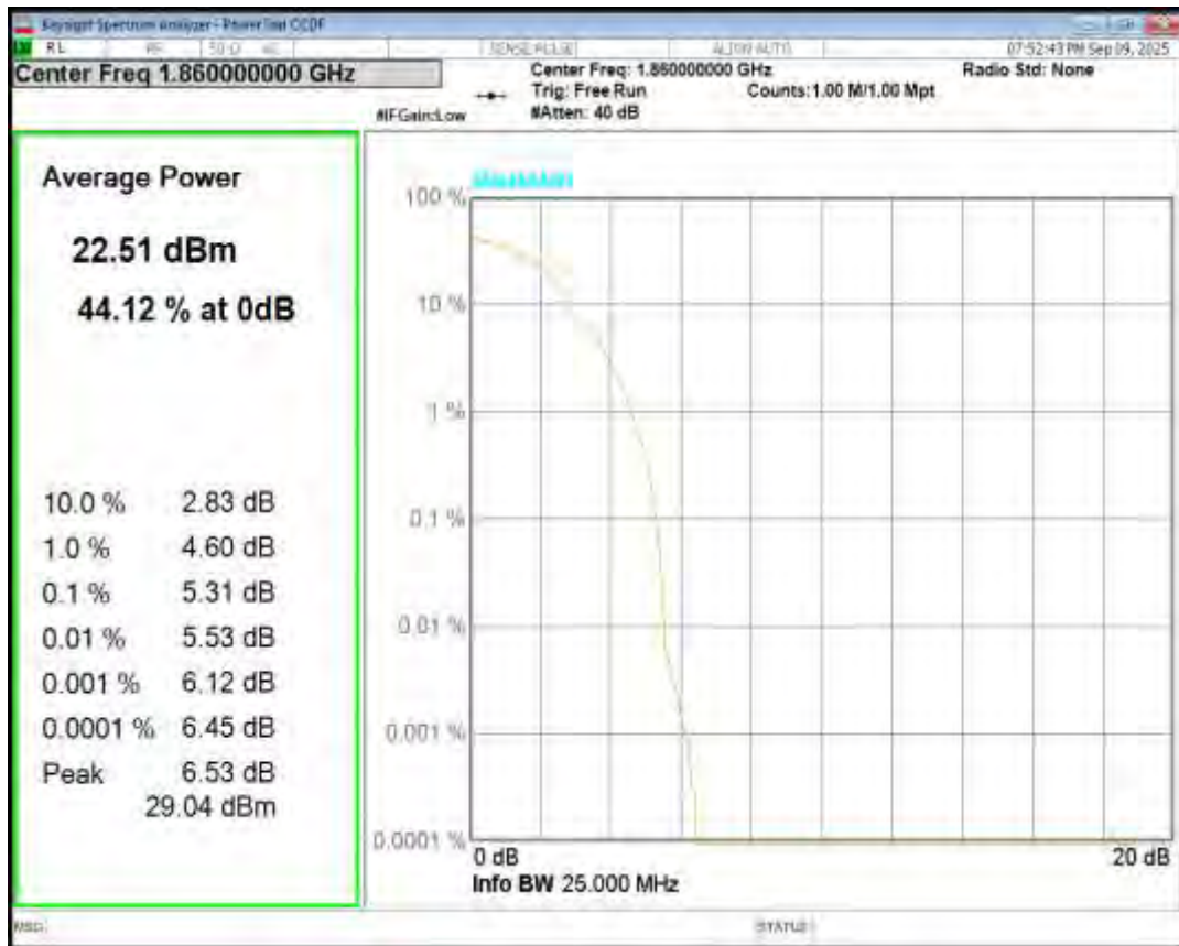
Band2 16QAM BW=20MHz Channel=18900 RB Size=1 Position=#0
