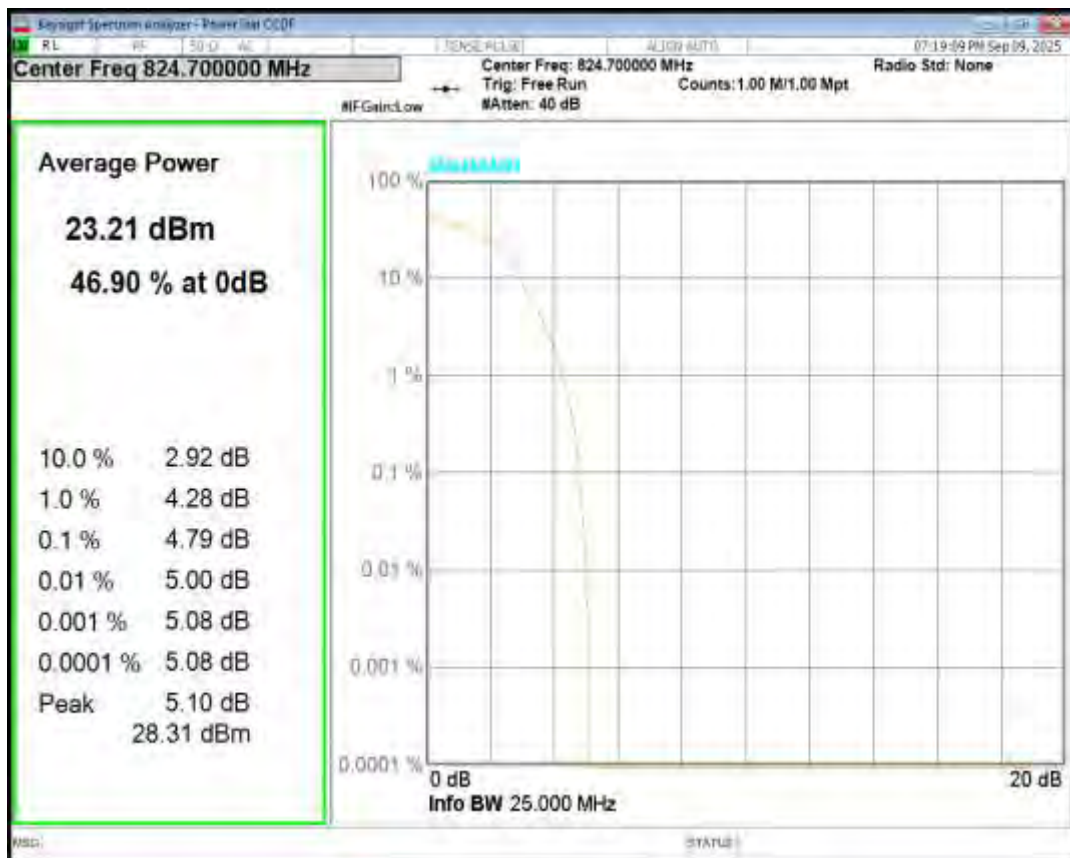
Band5 16QAM BW=1.4MHz Channel=20525 RB Size=1 Position=#0
