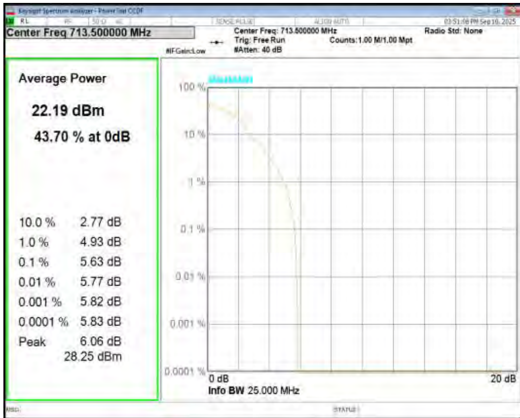
Band12 QPSK BW=1.4MHz Channel=23017 RB Size=1 Position=#0
