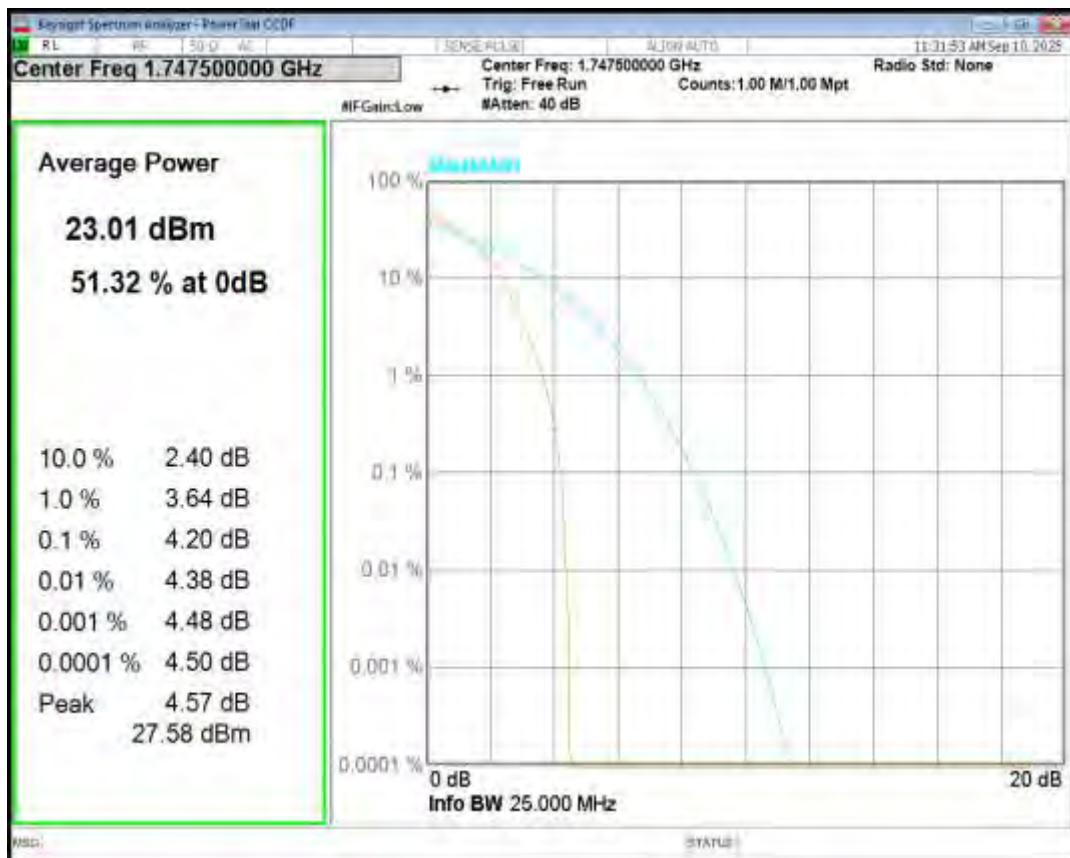
Band4 QPSK BW=20MHz Channel=20050 RB Size=1 Position=#0
