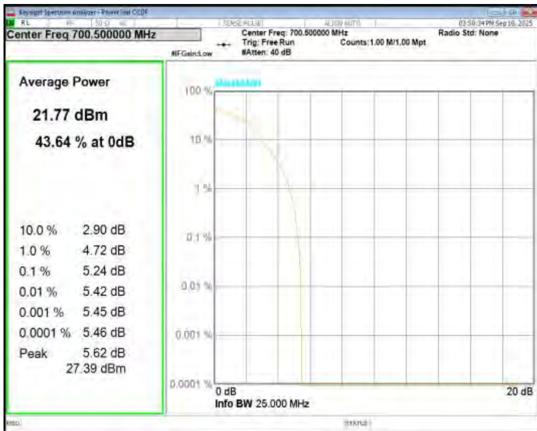
Band12 16QAM BW=3MHz Channel=23095 RB Size=1 Position=#0
