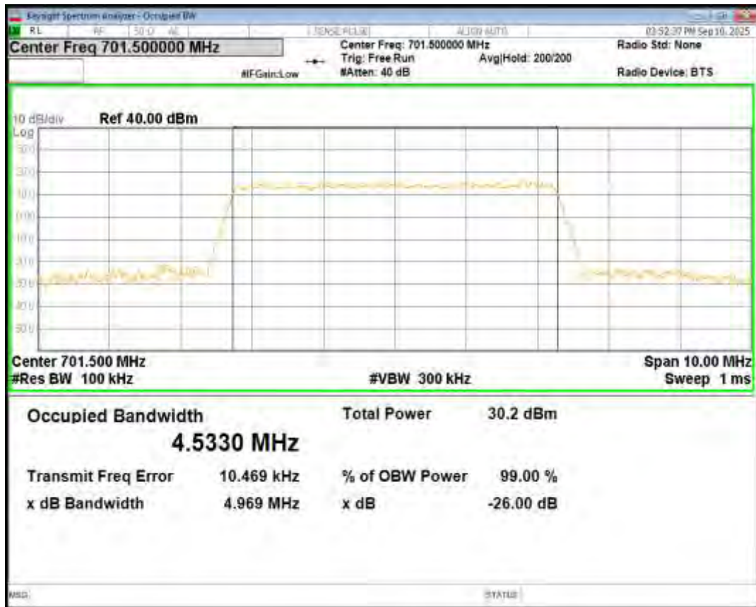
Band12 QPSK BW=5MHz Channel=23095 RB Size=25 Position=#0
