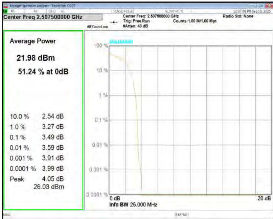
Band7 16QAM BW=15MHz Channel=21100 RB Size=1 Position=#0
