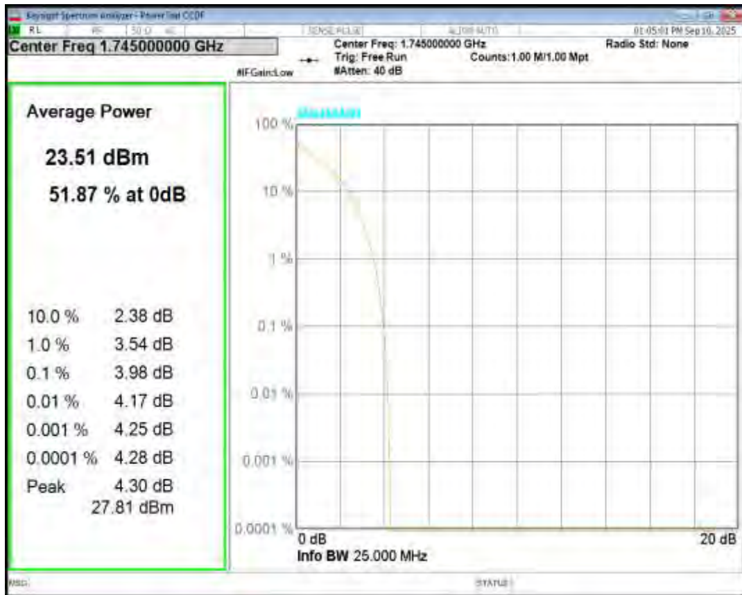
Band66 QPSK BW=15MHz Channel=132597 RB Size=1 Position=#0
