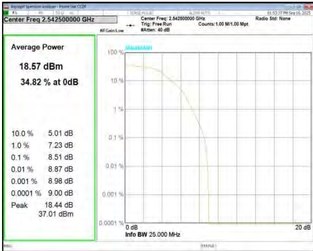
Band41(2535-2655) QPSK BW=15MHz Channel=40640 RB Size=1 Position=#0
