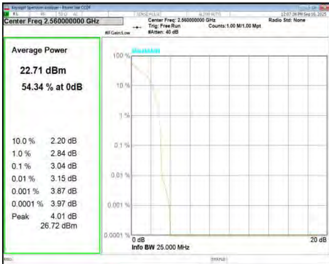
Band7 QPSK BW=5MHz Channel=21100 RB Size=1 Position=#0
