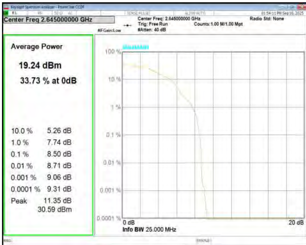
Band41(2535-2655) 16QAM BW=5MHz Channel=40065 RB Size=1 Position=#0
