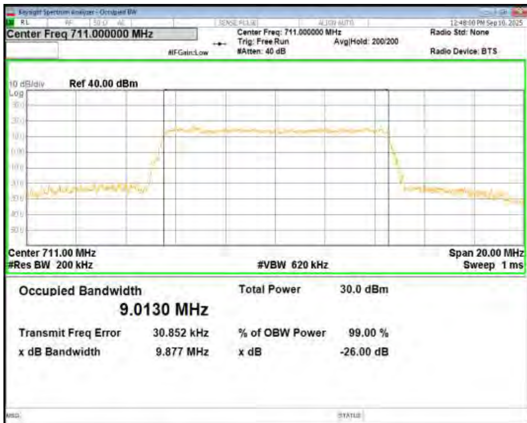
Band17 QPSK BW=5MHz Channel=23755 RB Size=25 Position=#0
