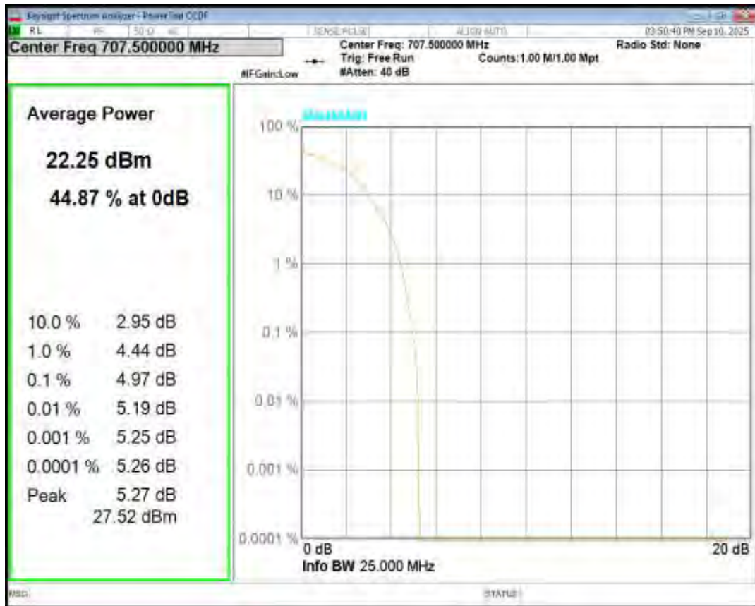
Band12 16QAM BW=3MHz Channel=23165 RB Size=1 Position=#0
