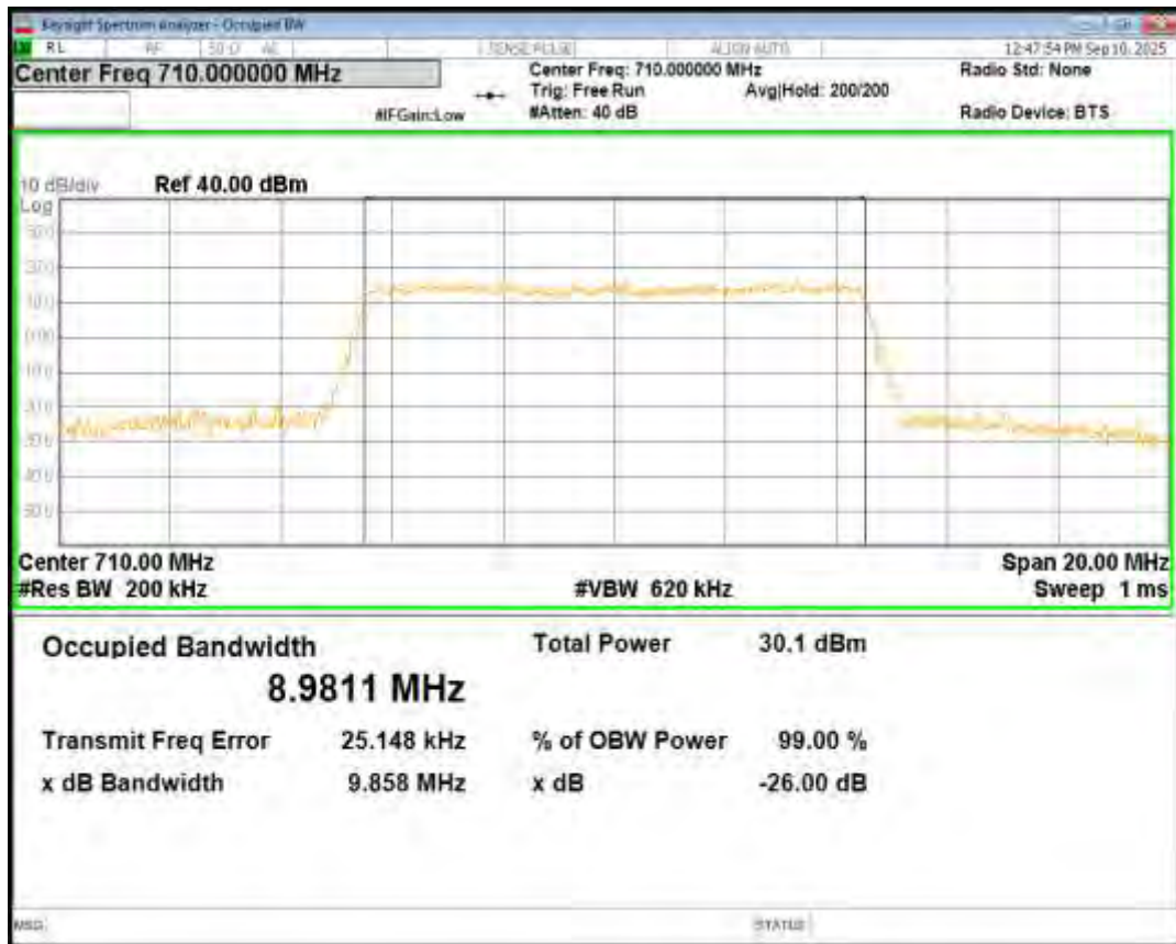
Band17 QPSK BW=10MHz Channel=23800 RB Size=50 Position=#0
