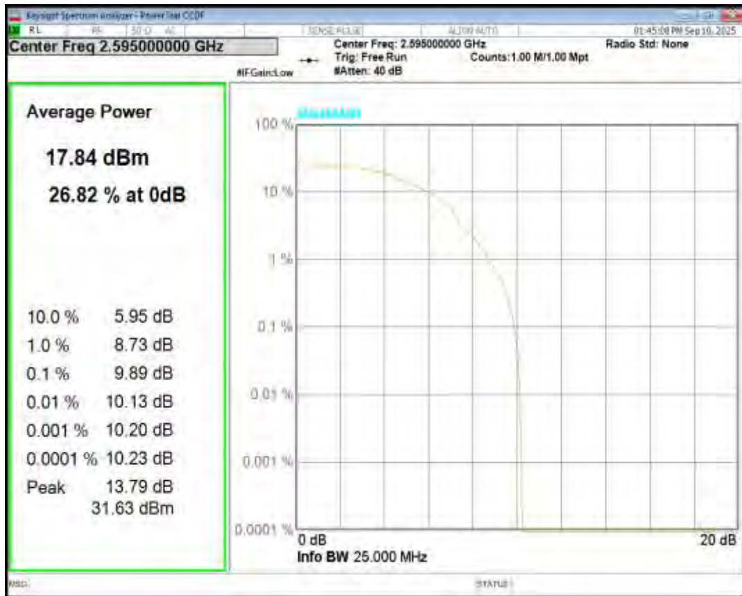
Band41(2535-2655) QPSK BW=10MHz Channel=40090 RB Size=1 Position=#0
