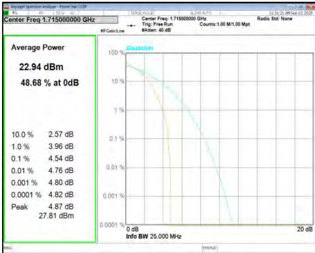
Band4 QPSK BW=10MHz Channel=20175 RB Size=1 Position=#0
