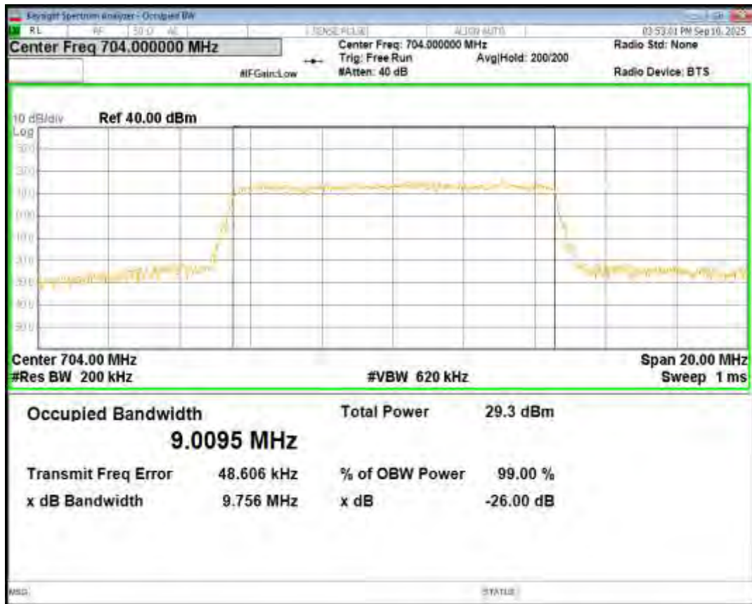
Band12 16QAM BW=10MHz Channel=23095 RB Size=50 Position=#0
