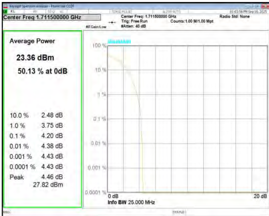
Band66 QPSK BW=3MHz Channel=132322 RB Size=1 Position=#0
