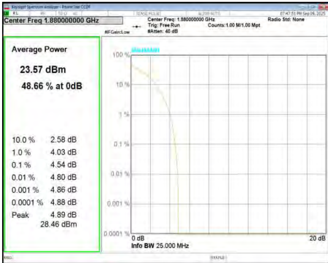
Band2 QPSK BW=3MHz Channel=19185 RB Size=1 Position=#0
