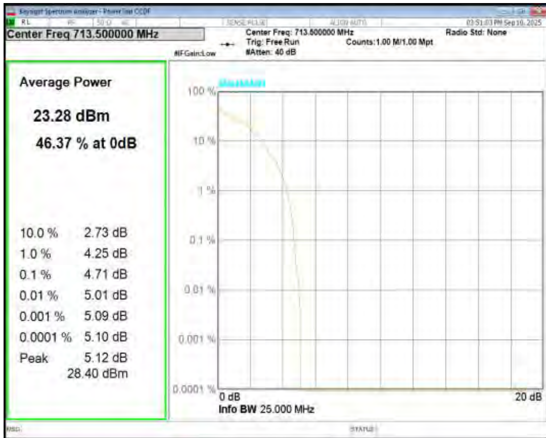
Band17 16QAM BW=10MHz Channel=23780 RB Size=1 Position=#0
