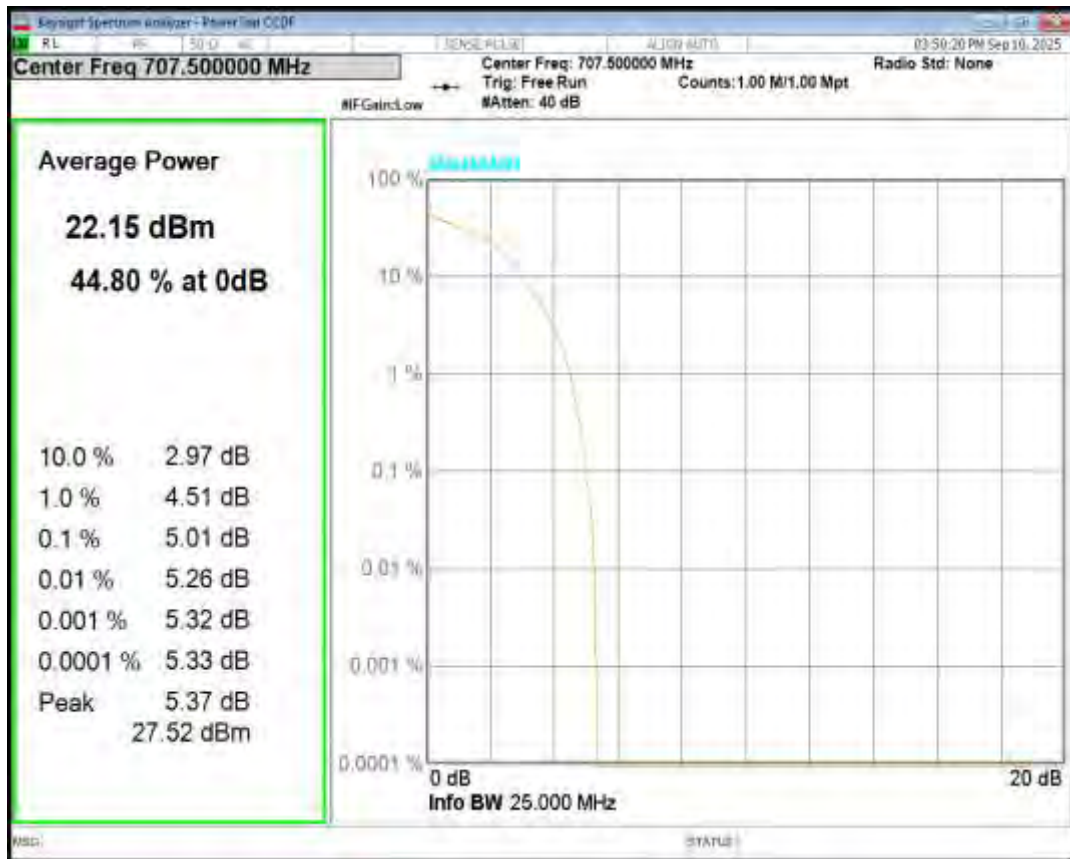
Band12 16QAM BW=1.4MHz Channel=23173 RB Size=1 Position=#0
