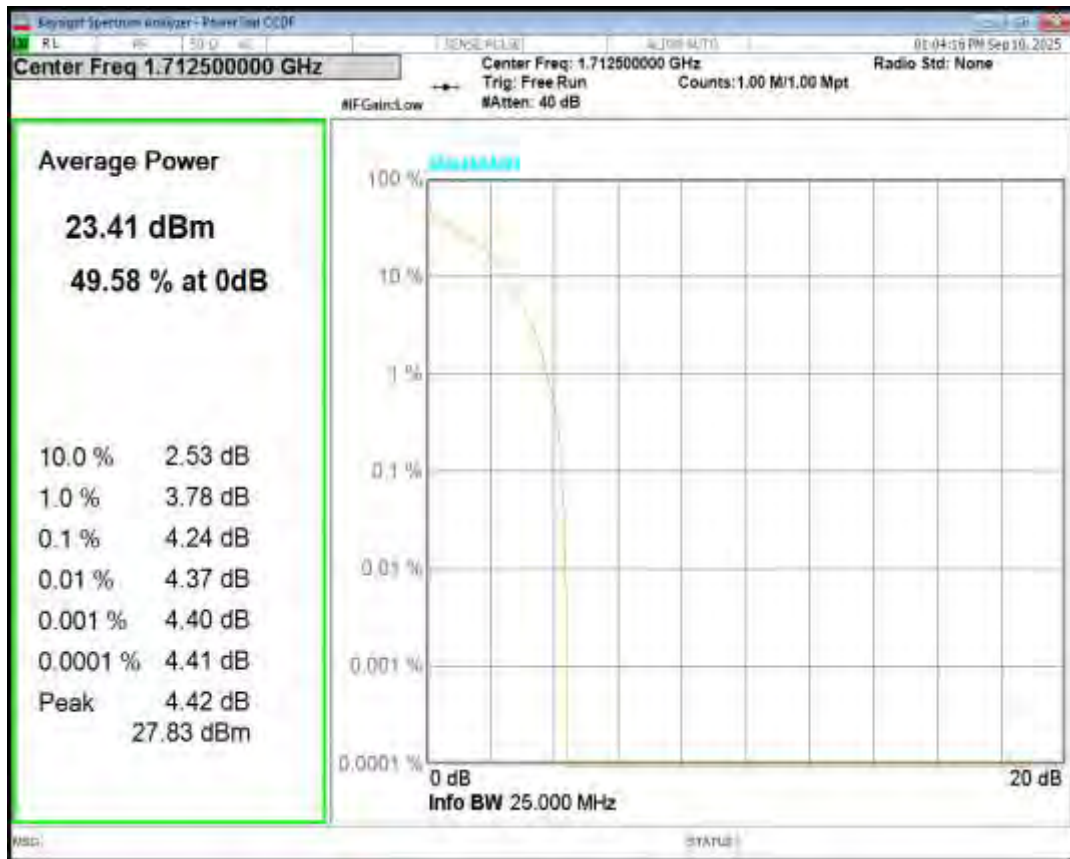
Band66 QPSK BW=5MHz Channel=132322 RB Size=1 Position=#0
