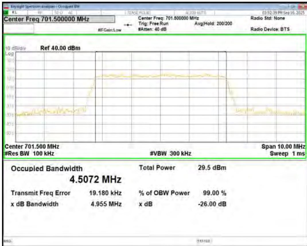
Band12 16QAM BW=5MHz Channel=23095 RB Size=25 Position=#0
