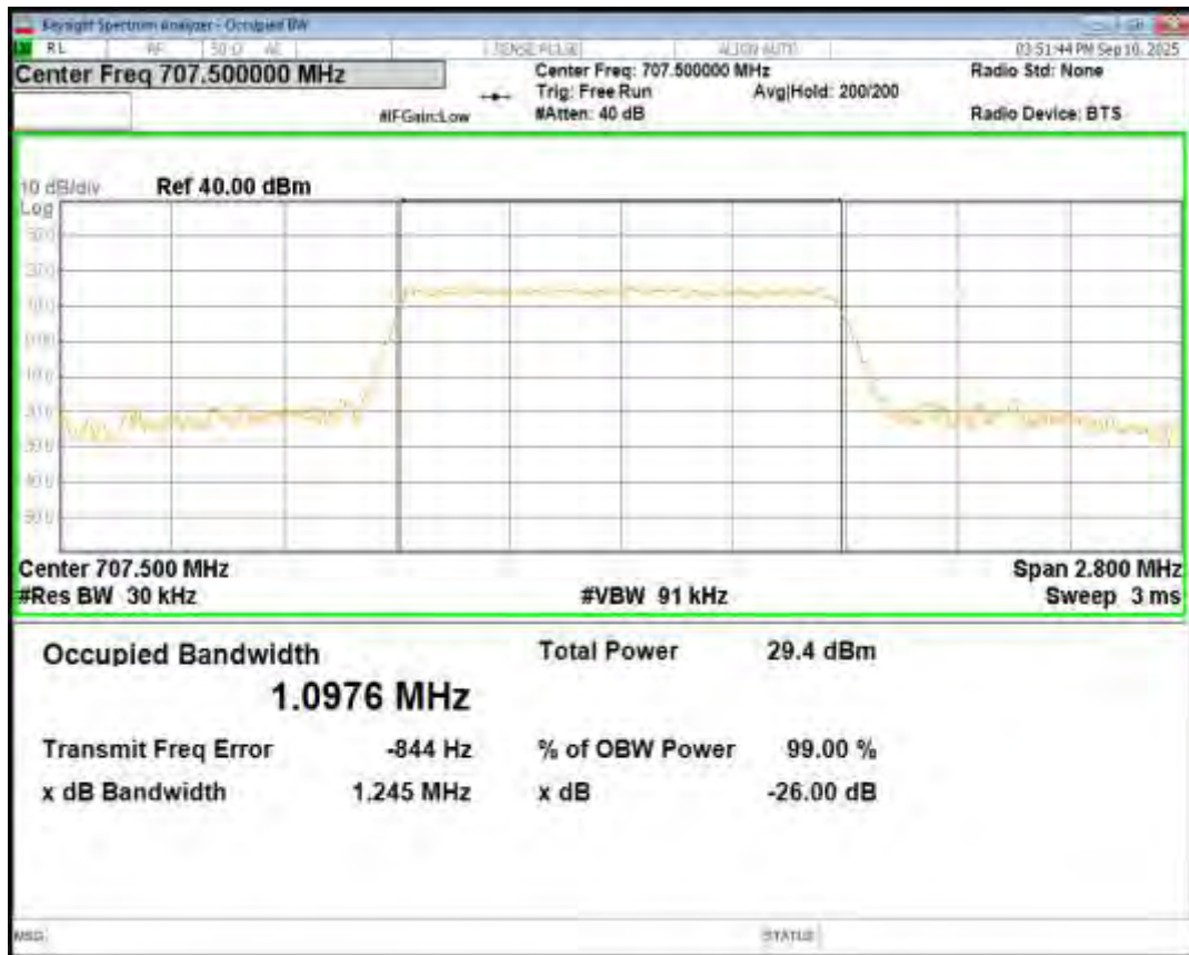
Band12 16QAM BW=1.4MHz Channel=23173 RB Size=6 Position=#0
