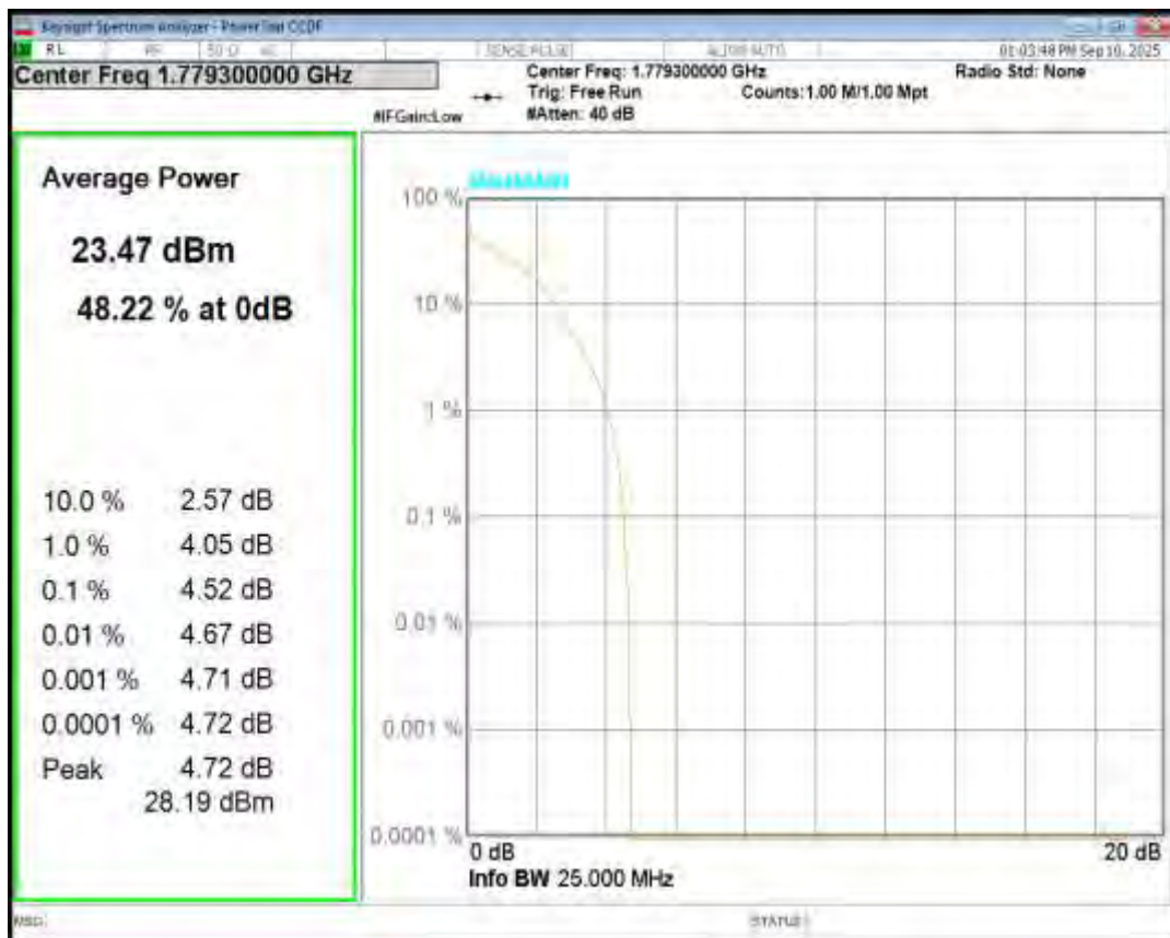
Band66 QPSK BW=10MHz Channel=132022 RB Size=1 Position=#0
