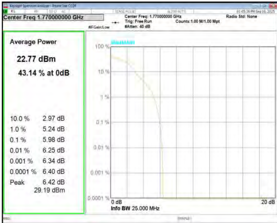
Band66 16QAM BW=3MHz Channel=131987 RB Size=1 Position=#0
