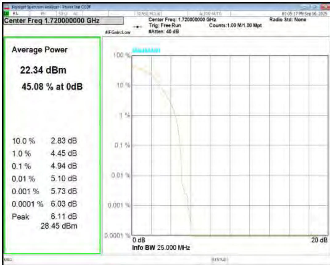
Band66 16QAM BW=20MHz Channel=132322 RB Size=1 Position=#0
