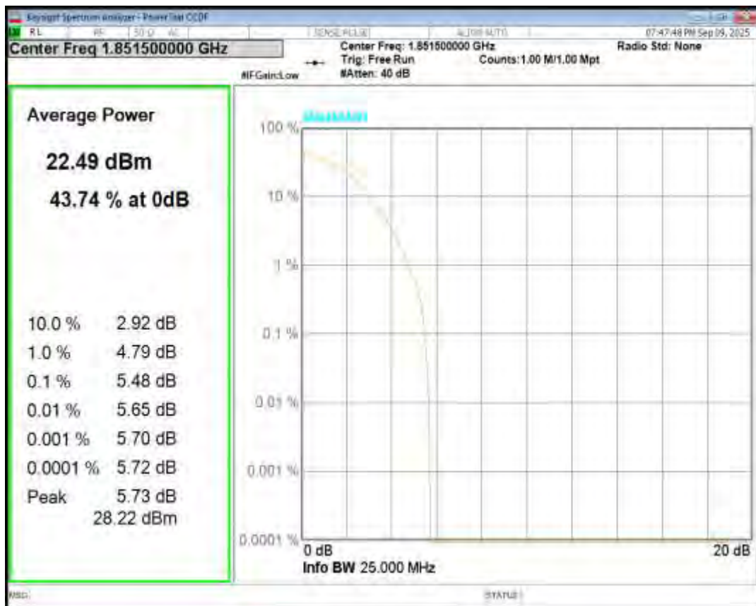
Band2 16QAM BW=3MHz Channel=18900 RB Size=1 Position=#0
