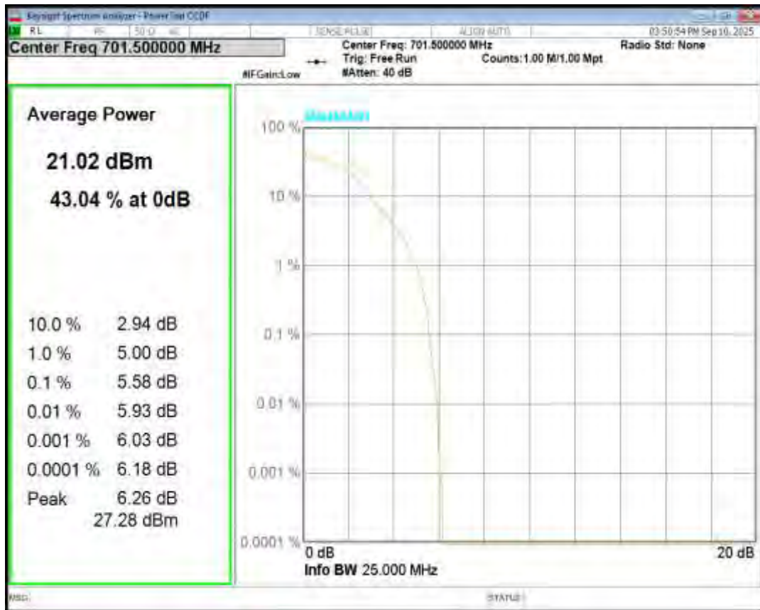
Band12 16QAM BW=5MHz Channel=23095 RB Size=1 Position=#0
