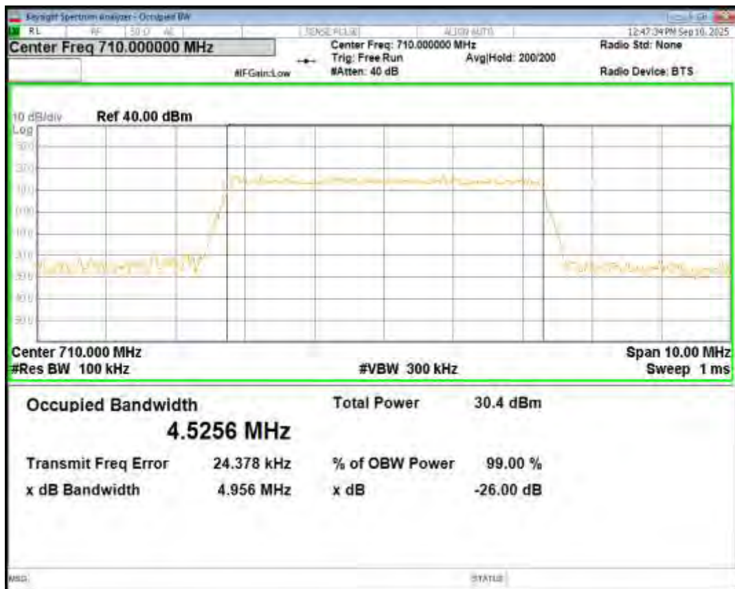
Band17 QPSK BW=5MHz Channel=23825 RB Size=25 Position=#0
