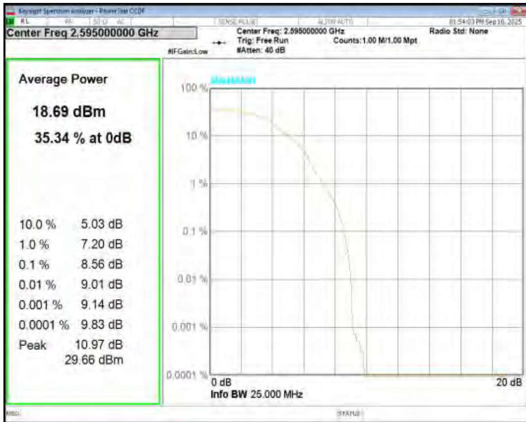
Band41(2535-2655) QPSK BW=5MHz Channel=40640 RB Size=1 Position=#0
