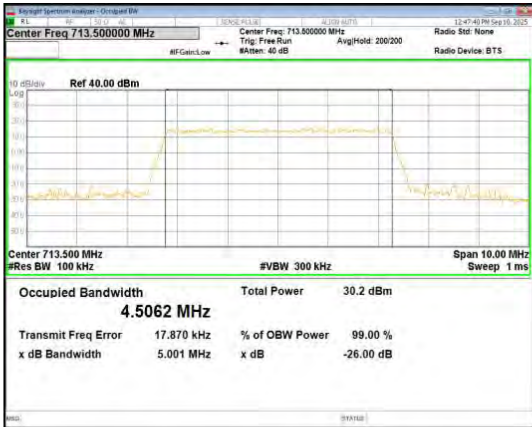
Band2 16QAM BW=1.4MHz Channel=18607 RB Size=6 Position=#0
