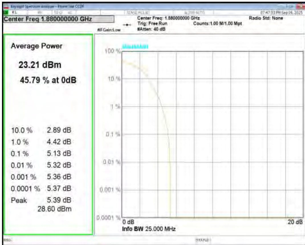
Band2 16QAM BW=3MHz Channel=19185 RB Size=1 Position=#0
