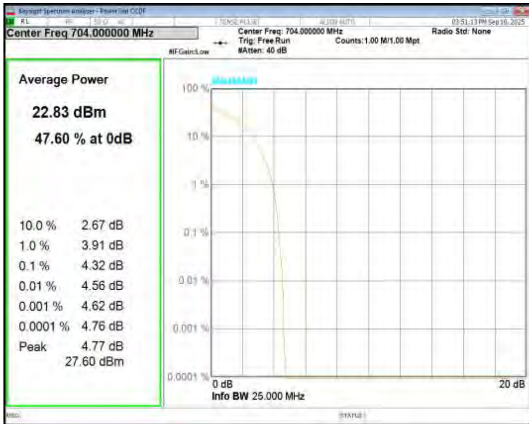
Band12 QPSK BW=10MHz Channel=23095 RB Size=1 Position=#0
