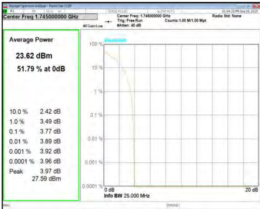
Band66 QPSK BW=5MHz Channel=132647 RB Size=1 Position=#0
