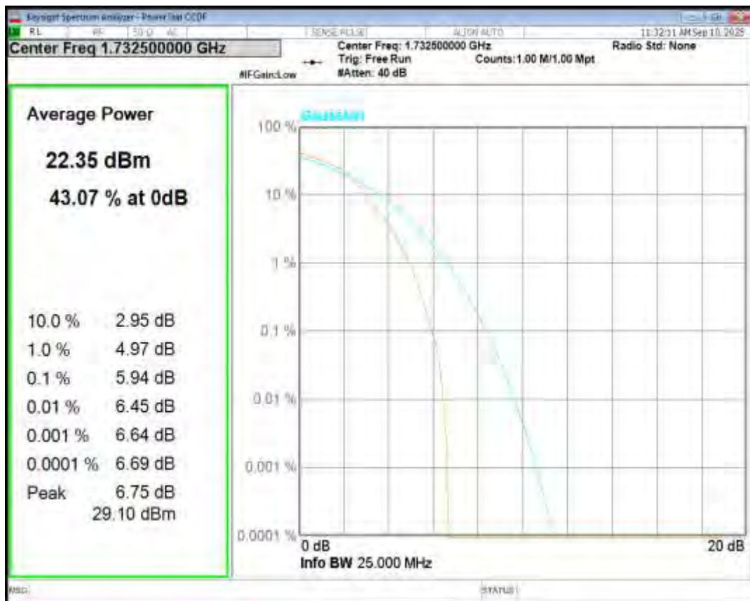
Band4 16QAM BW=20MHz Channel=20300 RB Size=1 Position=#0
