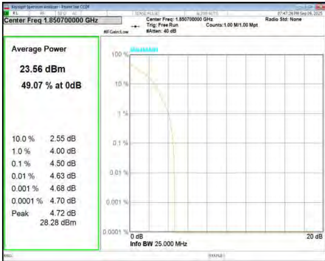
Band2 16QAM BW=5MHz Channel=19175 RB Size=1 Position=#0
