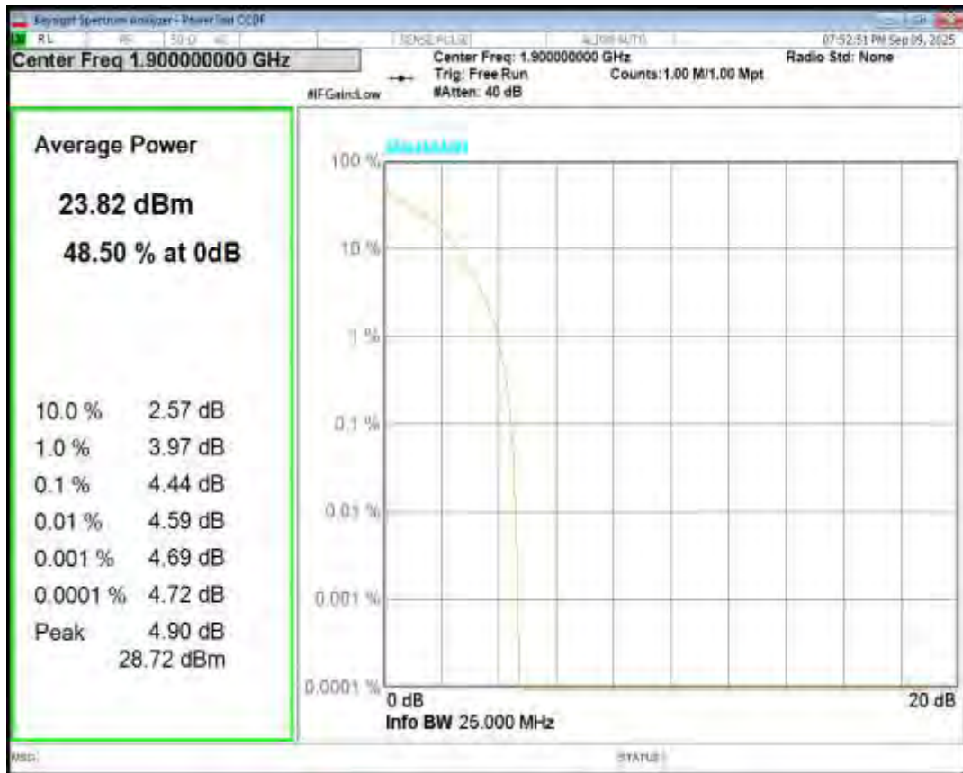
Band2 QPSK BW=3MHz Channel=18615 RB Size=1 Position=#0
