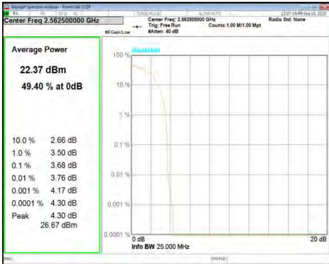
Band7 16QAM BW=20MHz Channel=20850 RB Size=1 Position=#0
