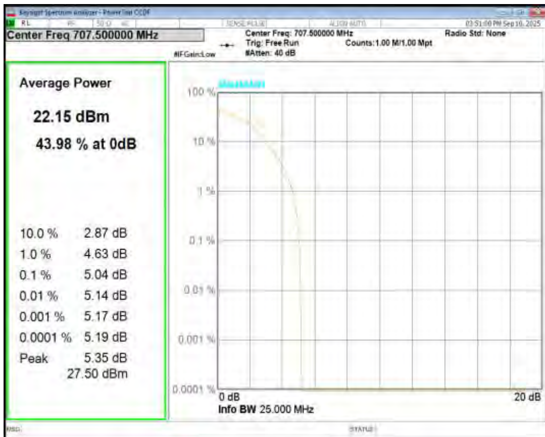
Band12 16QAM BW=5MHz Channel=23155 RB Size=1 Position=#0
