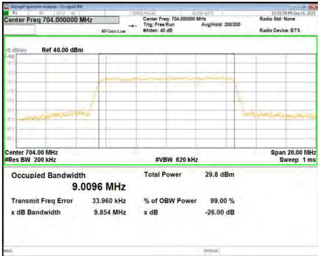
Band12 QPSK BW=10MHz Channel=23095 RB Size=50 Position=#0
