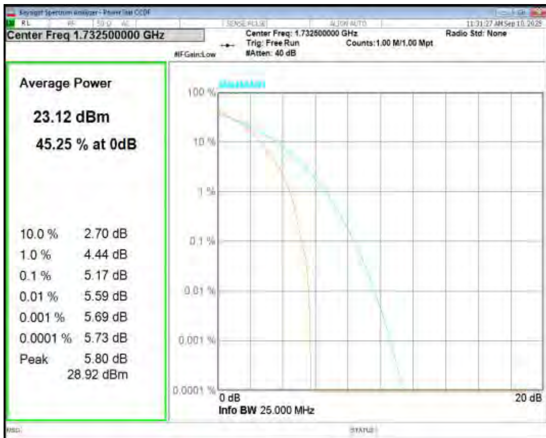
Band4 QPSK BW=10MHz Channel=20350 RB Size=1 Position=#0
