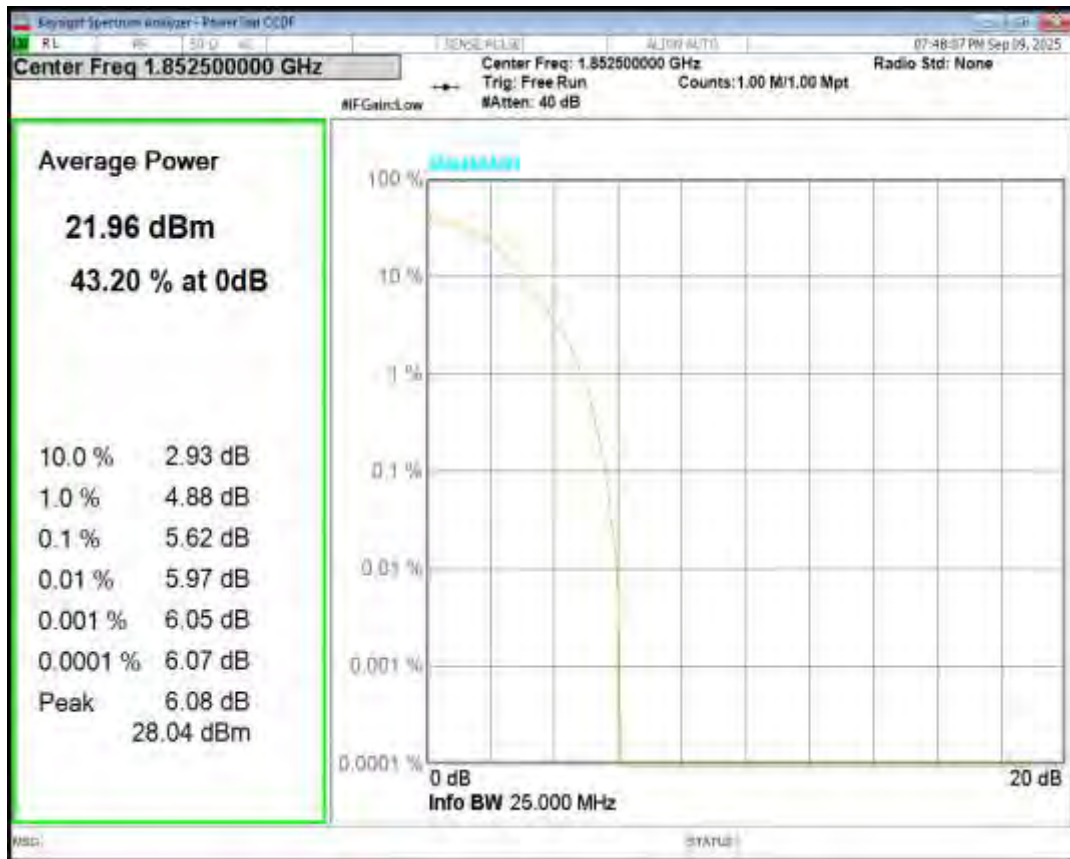
Band2 16QAM BW=5MHz Channel=18900 RB Size=1 Position=#0
