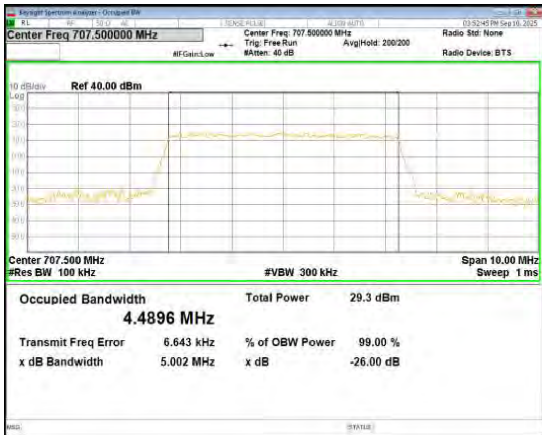
Band12 16QAM BW=5MHz Channel=23155 RB Size=25 Position=#0
