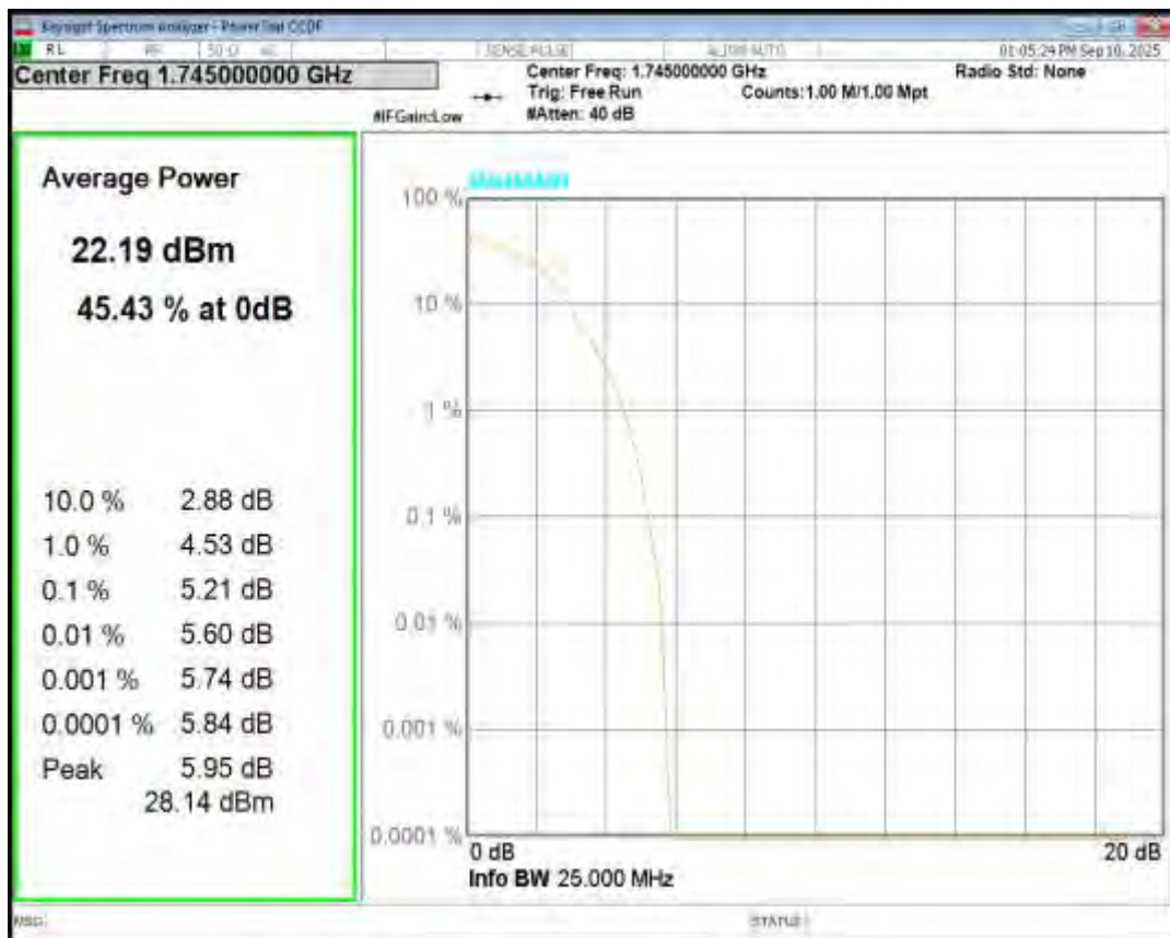
Band66 16QAM BW=20MHz Channel=132572 RB Size=1 Position=#0
