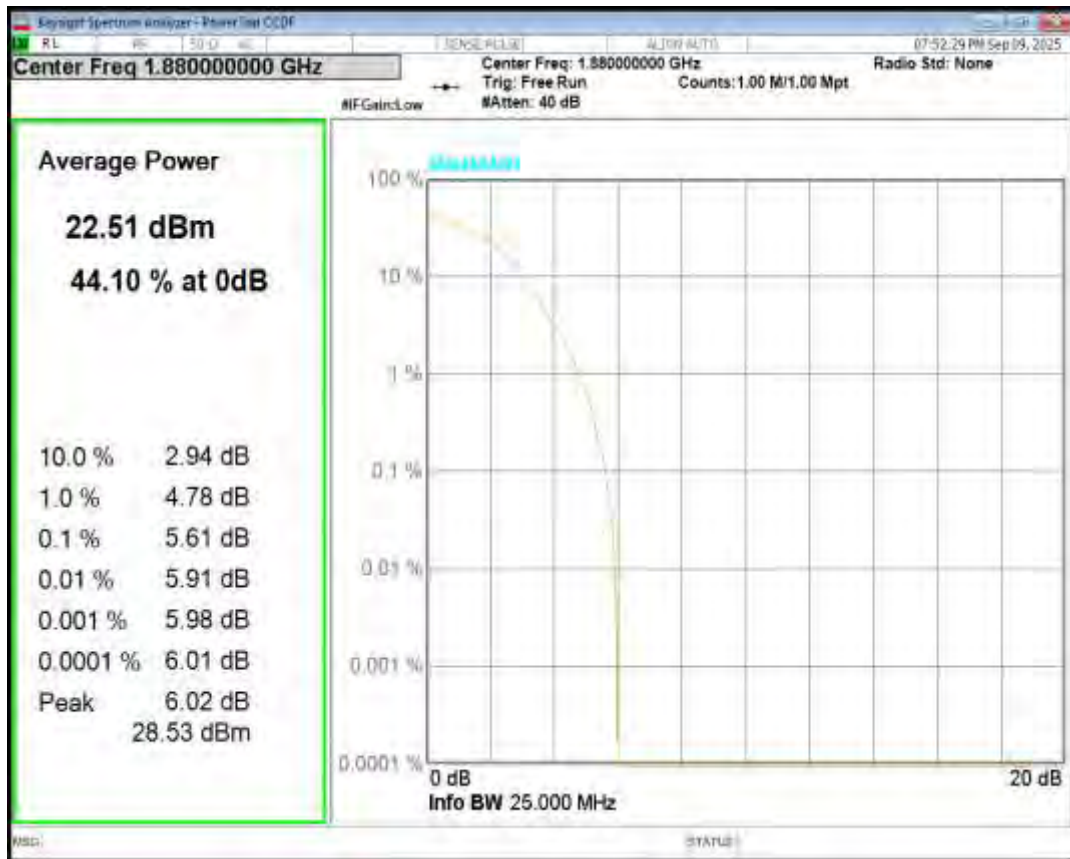
Band2 16QAM BW=15MHz Channel=19125 RB Size=1 Position=#0
