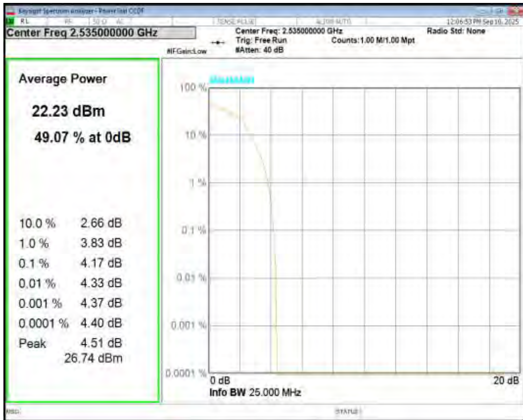
Band7 16QAM BW=10MHz Channel=21400 RB Size=1 Position=#0
