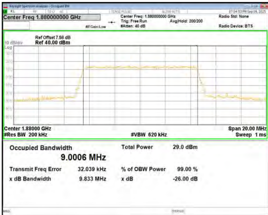
Band2 16QAM BW=10MHz Channel=19150 RB Size=50 Position=#0
