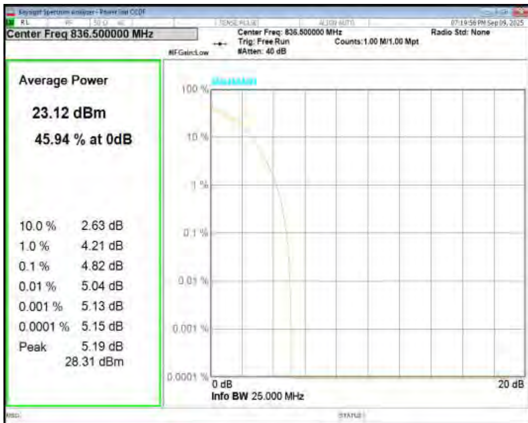
Band5 QPSK BW=5MHz Channel=20625 RB Size=1 Position=#0
