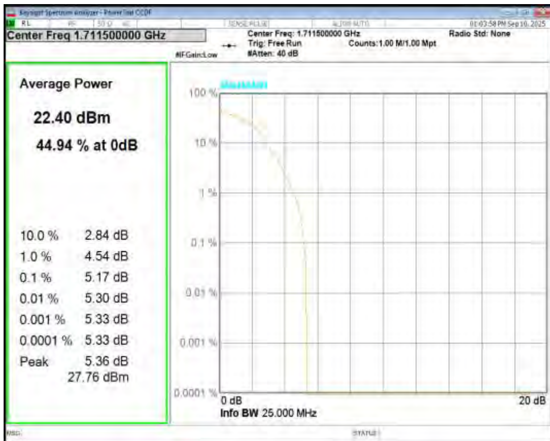
Band66 16QAM BW=3MHz Channel=132322 RB Size=1 Position=#0
