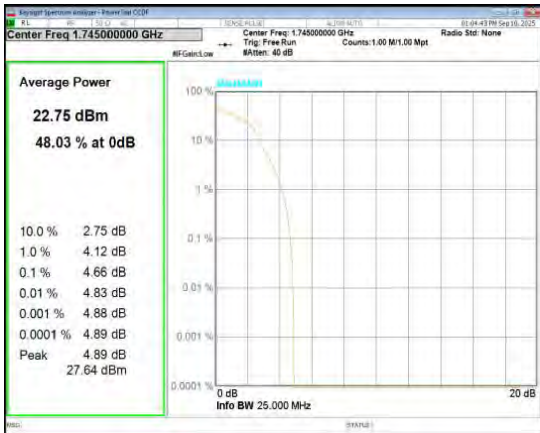
Band66 16QAM BW=10MHz Channel=132622 RB Size=1 Position=#0
