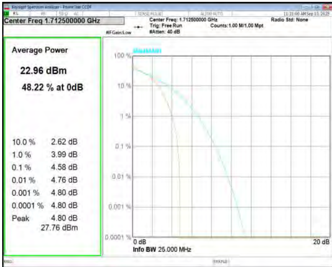
Band4 QPSK BW=5MHz Channel=20175 RB Size=1 Position=#0
