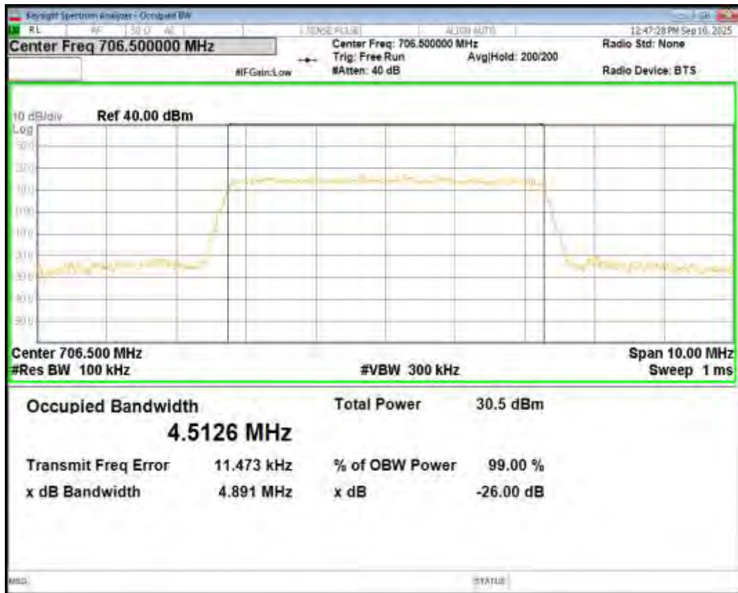
Band17 QPSK BW=5MHz Channel=23790 RB Size=25 Position=#0
