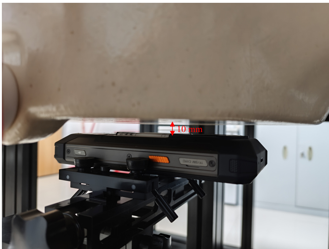
Main Ant Body Back Setup Photo (10 mm)
