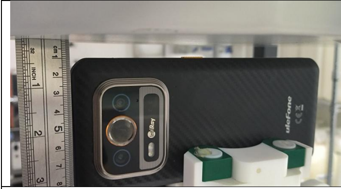
Top Side (Separation distance of 10mm)
