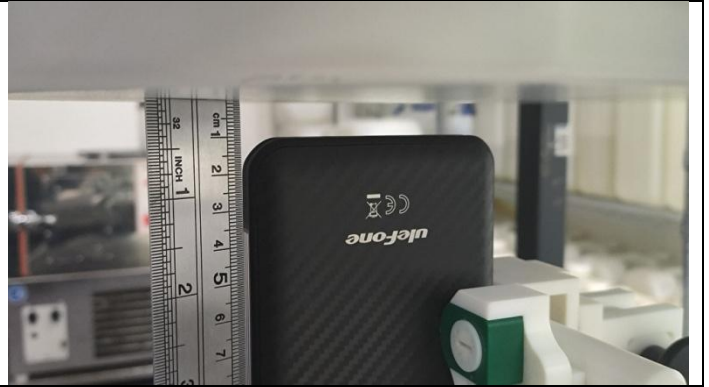
Bottom Side (Separation distance of 10mm)
