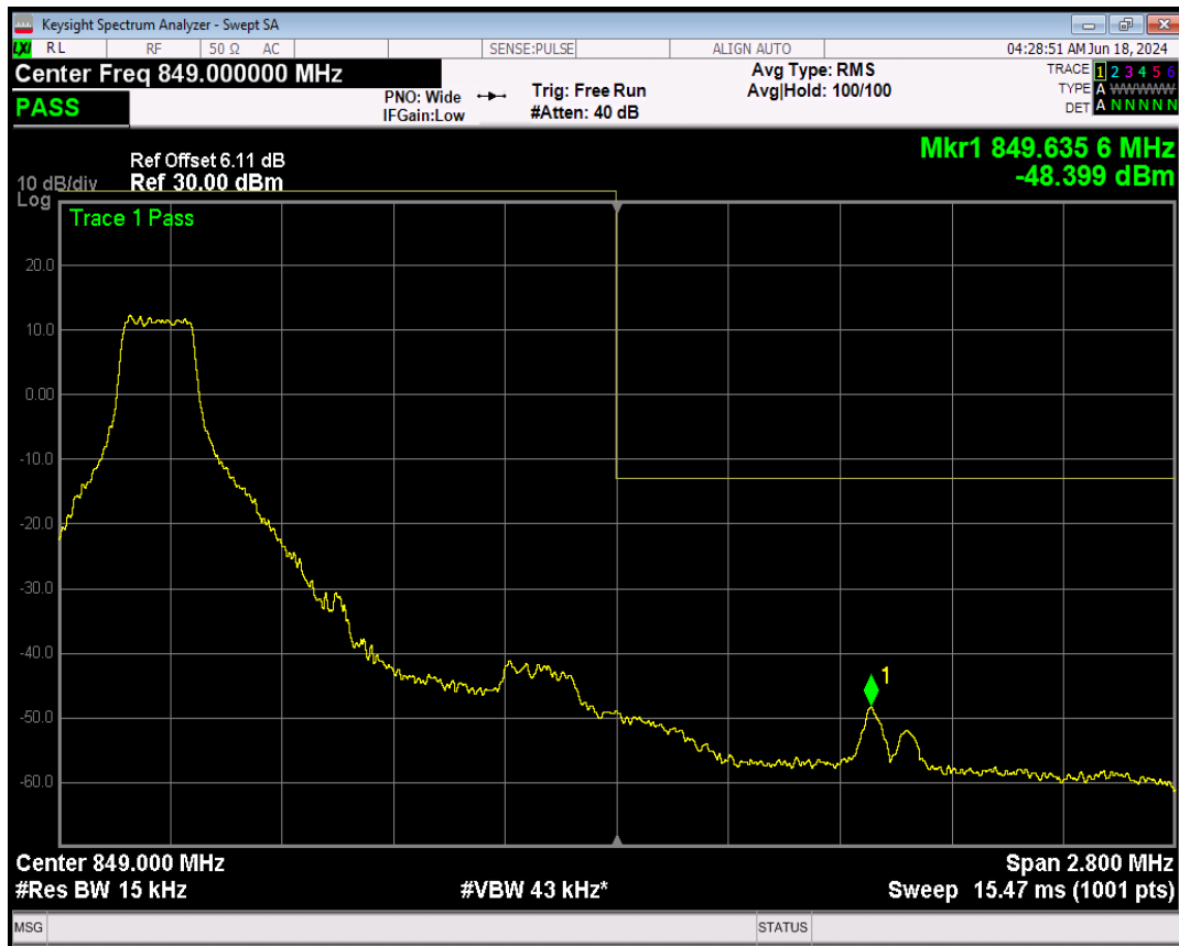
Band5 16QAM BW=1.4MHz Channel=20643 RB Size=1 Position=#Max
