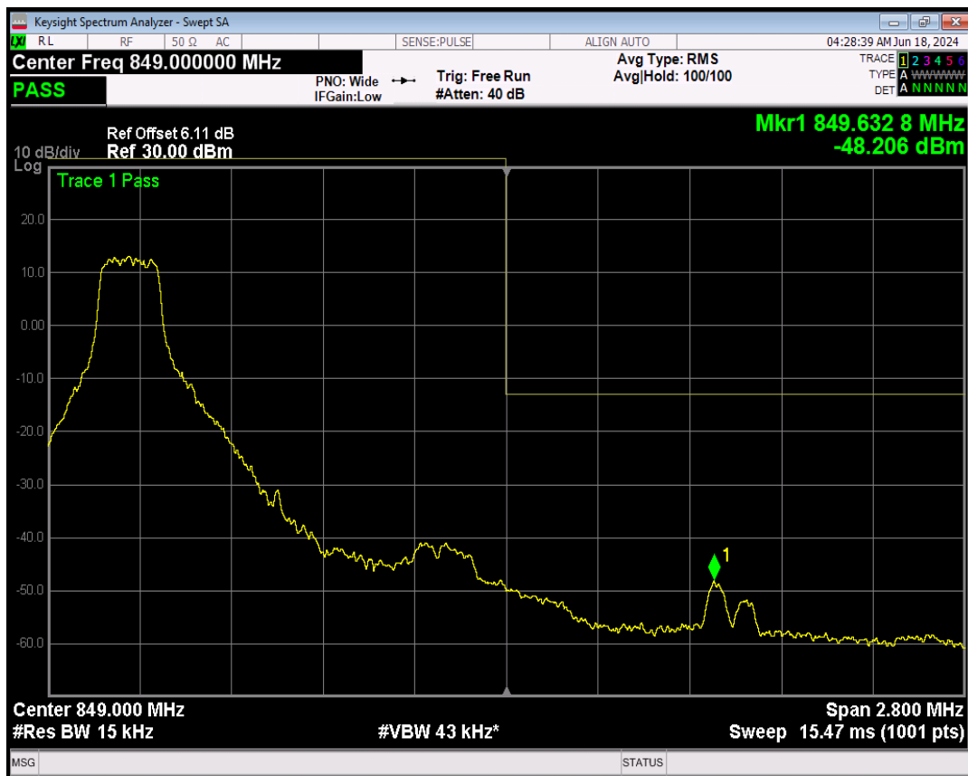
Band5 QPSK BW=1.4MHz Channel=20643 RB Size=1 Position=#Max
