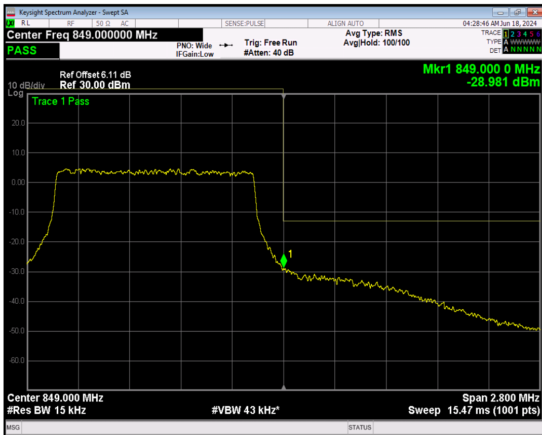
Band5 16QAM BW=1.4MHz Channel=20643 RB Size=1 Position=#0
