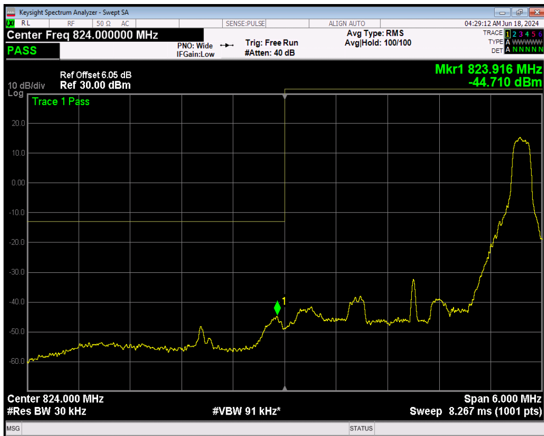
Band5 16QAM BW=3MHz Channel=20415 RB Size=15 Position=#0
