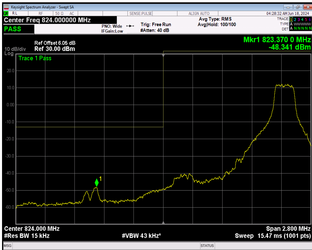
Band5 16QAM BW=1.4MHz Channel=20407 RB Size=6 Position=#0
