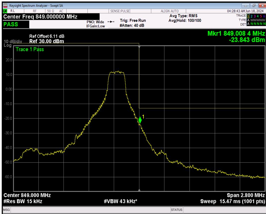
Band5 QPSK BW=1.4MHz Channel=20643 RB Size=6 Position=#0
