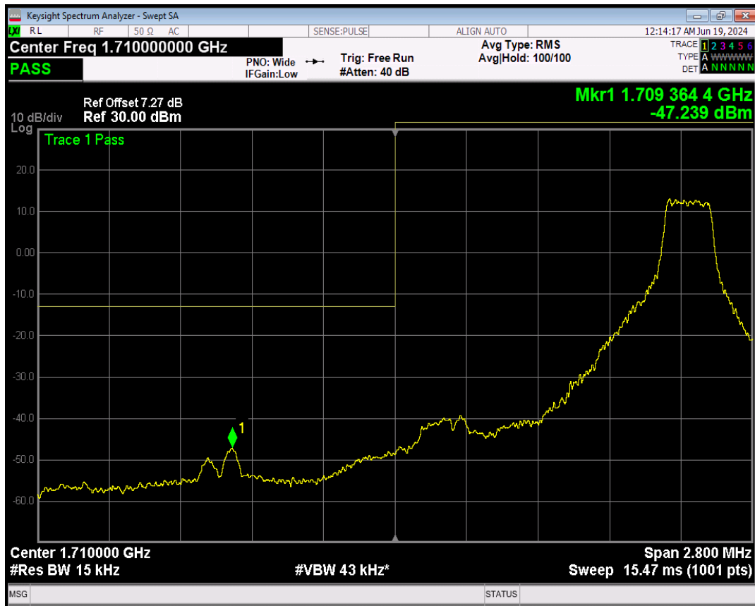
Band66 QPSK BW=1.4MHz Channel=132665 RB Size=1 Position=#0
