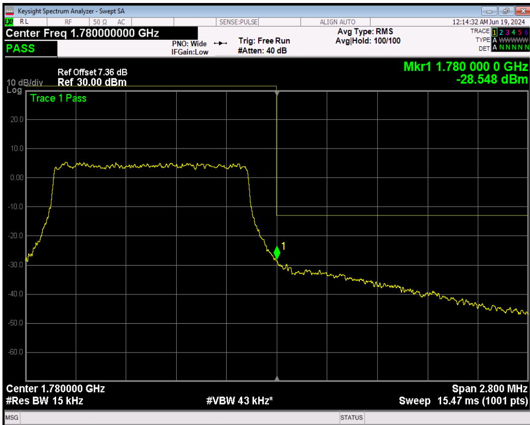
Band66 16QAM BW=1.4MHz Channel=132665 RB Size=1 Position=#0
