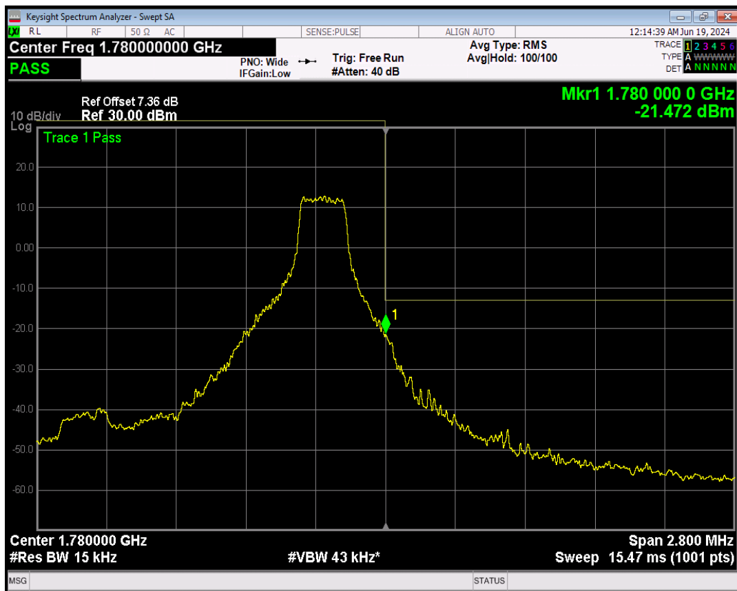
Band66 16QAM BW=1.4MHz Channel=132665 RB Size=6 Position=#0
