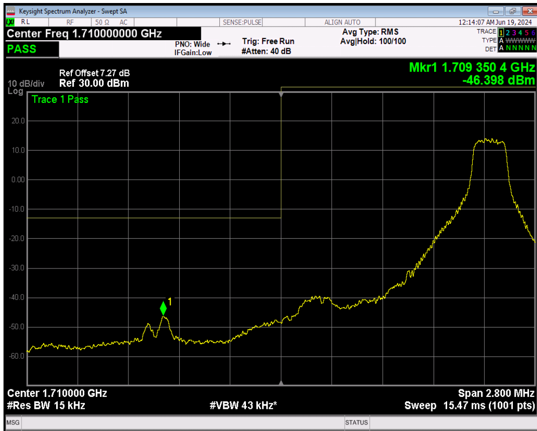
Band66 QPSK BW=1.4MHz Channel=131979 RB Size=6 Position=#0
