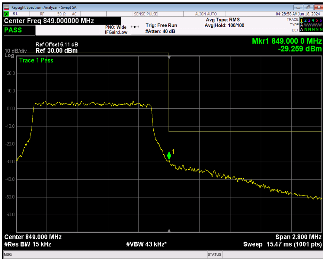
Band5 QPSK BW=3MHz Channel=20415 RB Size=1 Position=#Max
