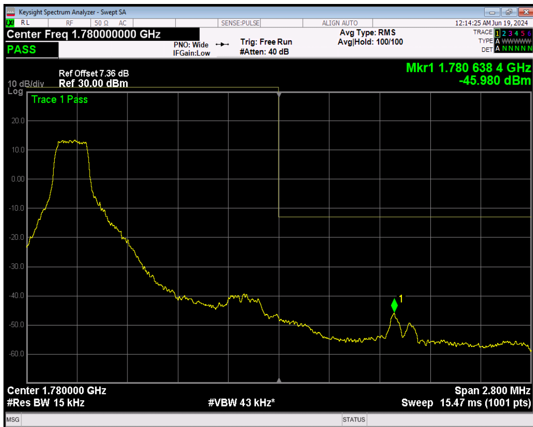
Band66 QPSK BW=1.4MHz Channel=132665 RB Size=1 Position=#Max
