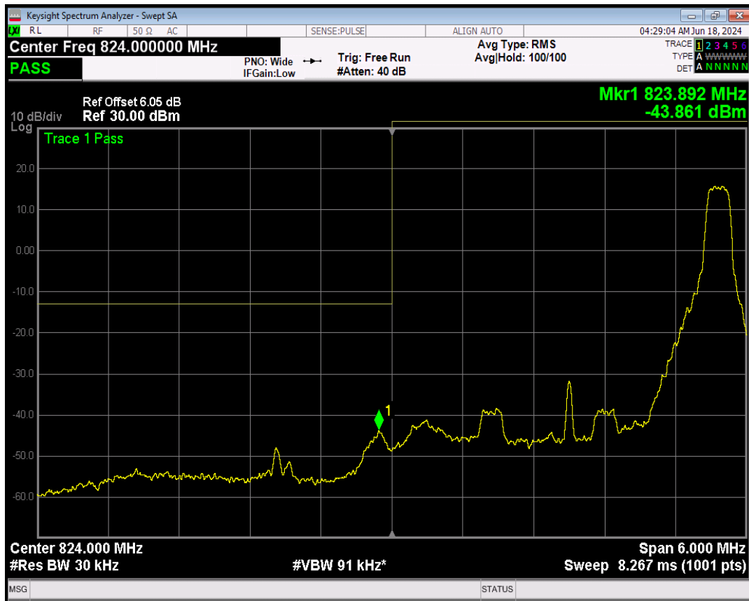
Band5 QPSK BW=3MHz Channel=20415 RB Size=15 Position=#0
