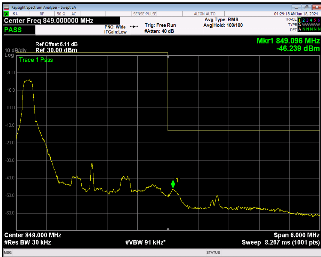
Band5 QPSK BW=3MHz Channel=20635 RB Size=1 Position=#Max
