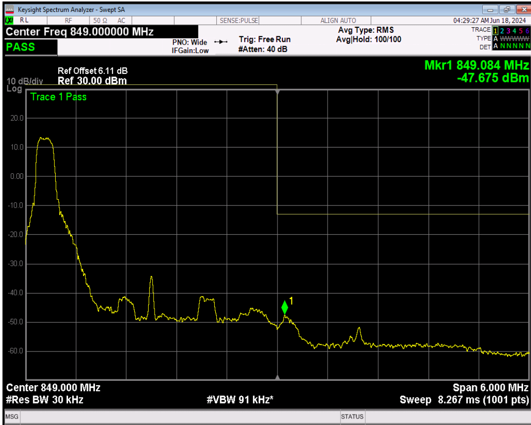
Band5 16QAM BW=3MHz Channel=20635 RB Size=1 Position=#Max
