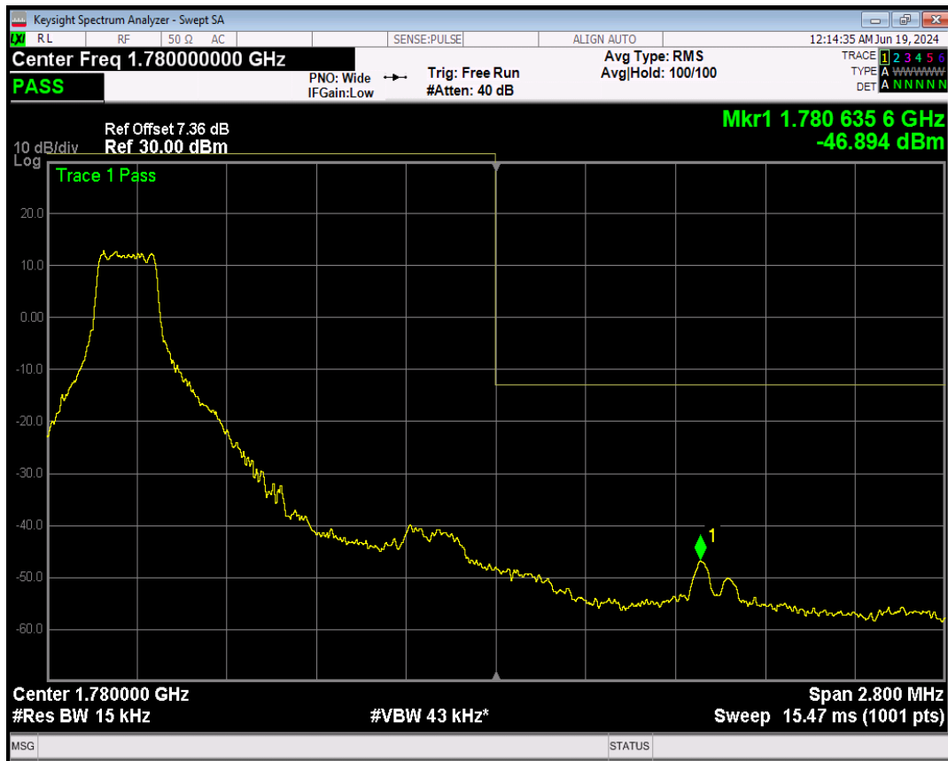
Band66 16QAM BW=1.4MHz Channel=132665 RB Size=1 Position=#Max
