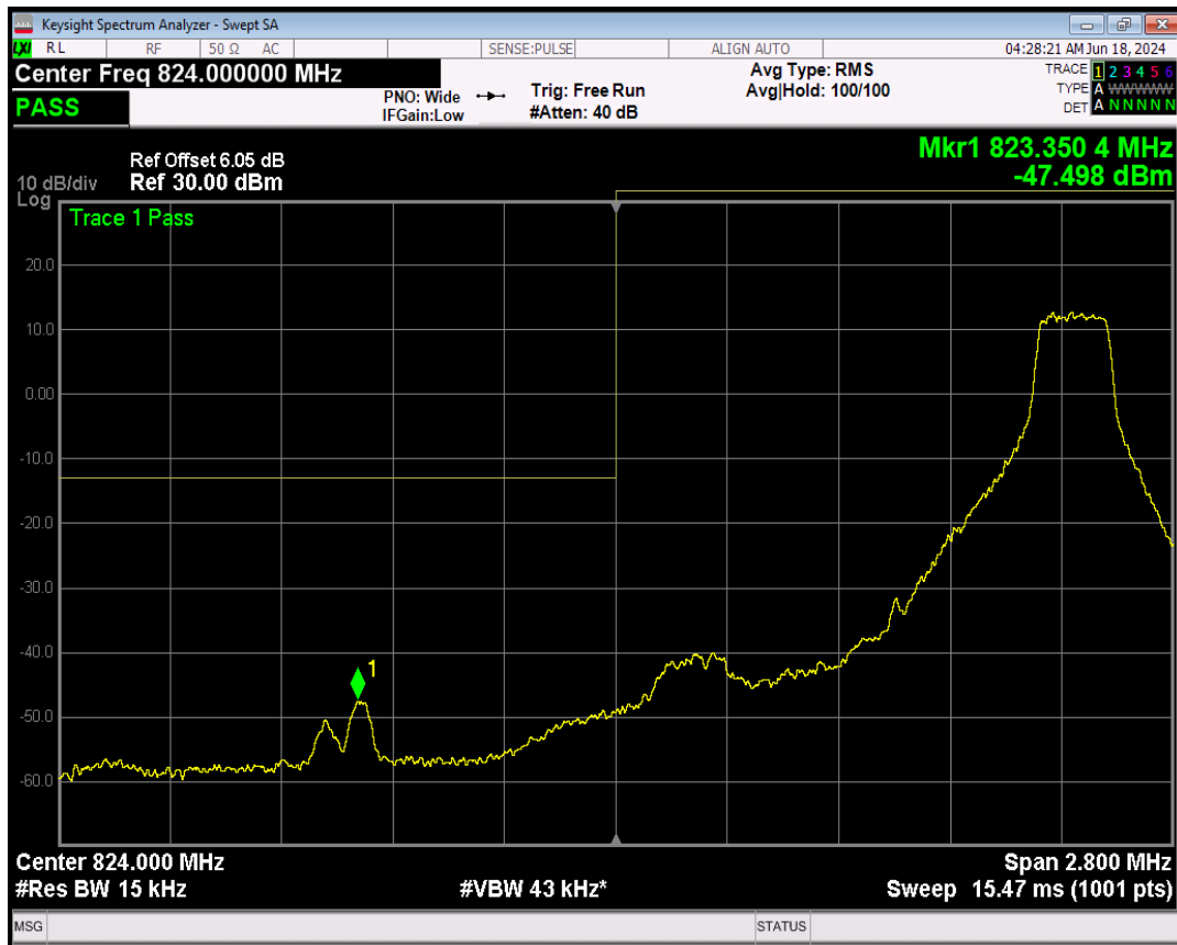
Band5 QPSK BW=1.4MHz Channel=20407 RB Size=6 Position=#0
