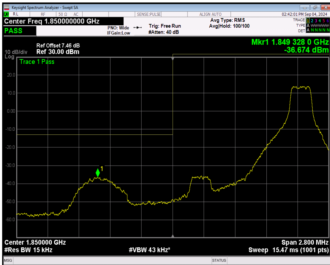
Band2 QPSK BW=1.4MHz Channel=18607 RB Size=6 Position=#0
