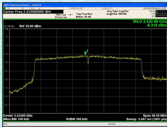
In-Band Reference Level IEEE 802.11ax_Channel 3_40MHz_Antenna 0+Antenna 1_RU&Index SU
