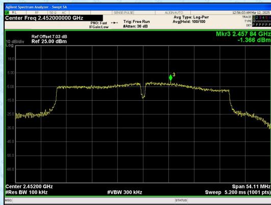
In-Band Reference Level IEEE 802.11n_Channel 9_40MHz_Antenna 0+Antenna 1
