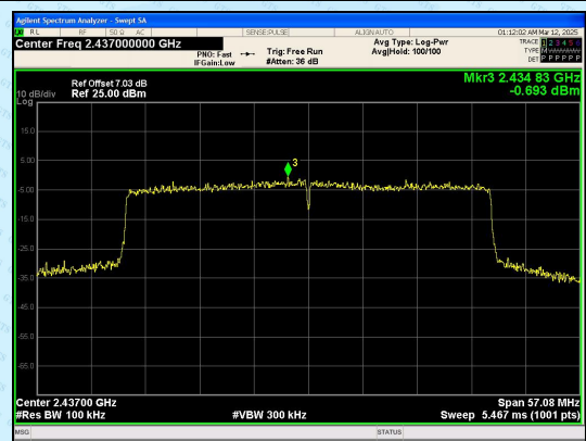
In-Band Reference Level IEEE 802.11ax_Channel 6_40MHz_Antenna 0+Antenna 1_RU&Index SU
