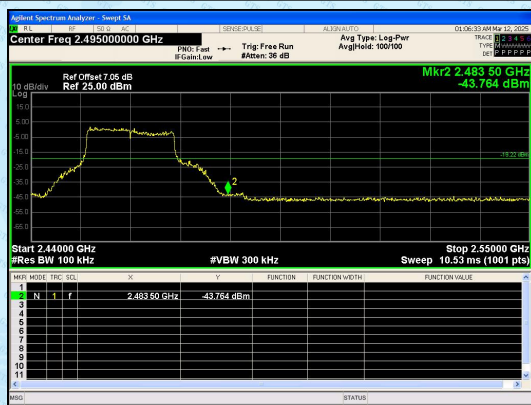
Out Of Band Emission IEEE 802.11ax_Channel 11_20MHz_Antenna 0+Antenna 1_RU&Index SU
