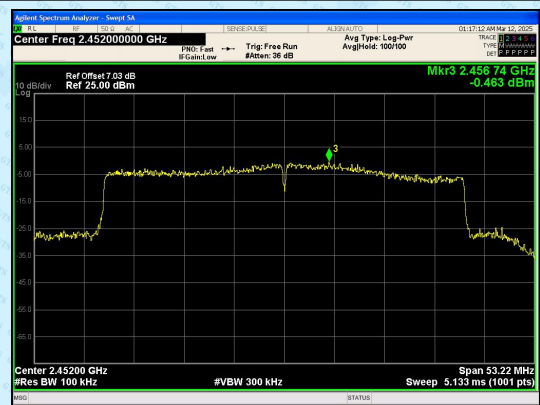
In-Band Reference Level IEEE 802.11ax_Channel 9_40MHz_Antenna 0+Antenna 1_RU&Index SU
