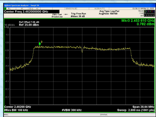
In-Band Reference Level IEEE 802.11ax_Channel 11_20MHz_Antenna 0+Antenna 1_RU&Index SU
