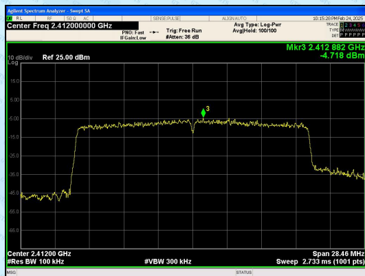
In-Band Reference Level IEEE 802.11ax_Channel 1_20MHz_Antenna 0+Antenna 1_RU&Index SU
