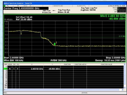
Out Of Band Emission IEEE 802.11n_Channel 9_40MHz_Antenna 0+Antenna 1
