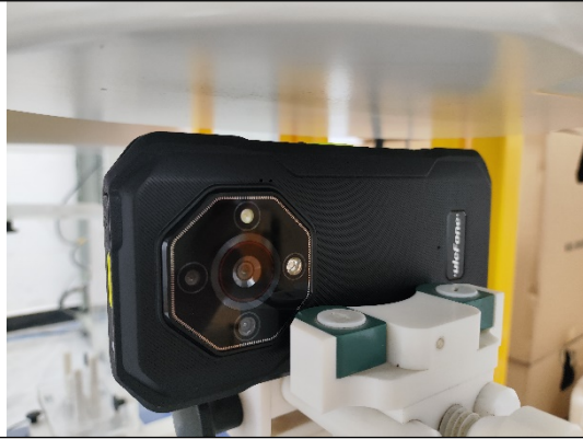
Top Side (Separation distance of 10mm)
