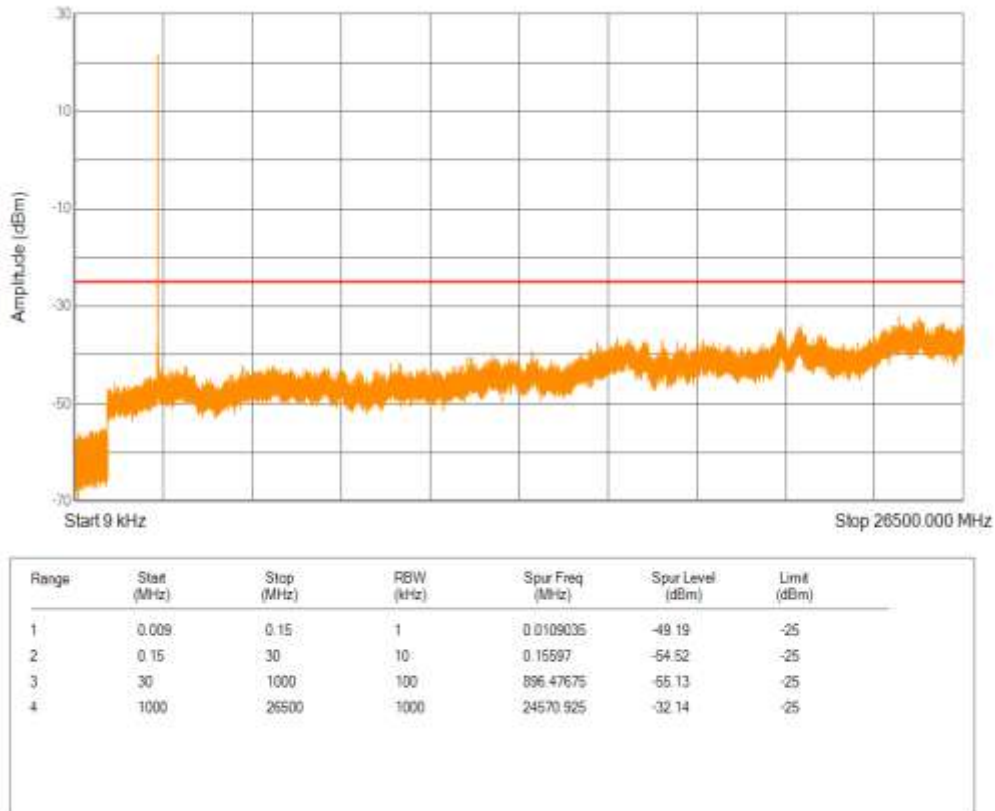
Band7 16QAM BW=5MHz Channel=21425 RB Size=25 Position=#0
