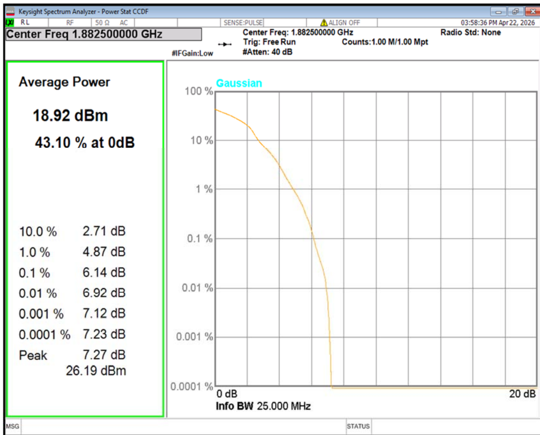
Band25 16QAM BW=5MHz Channel=26665 RB Size=1 Position=#0
