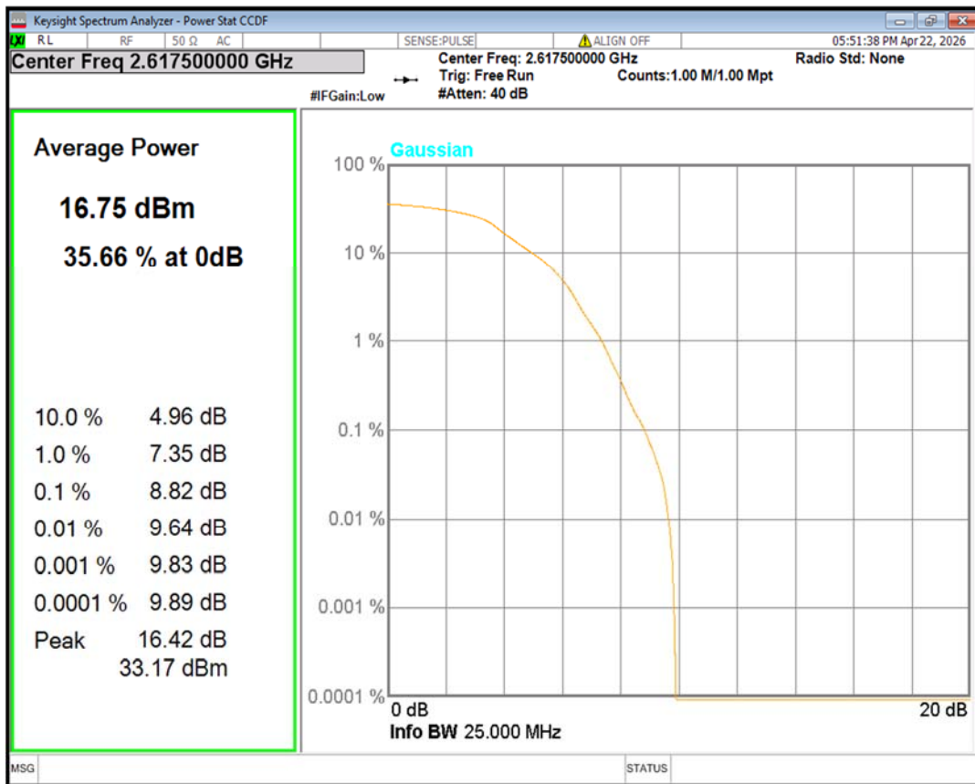
Band38 QPSK BW=10MHz Channel=37800 RB Size=1 Position=#0
