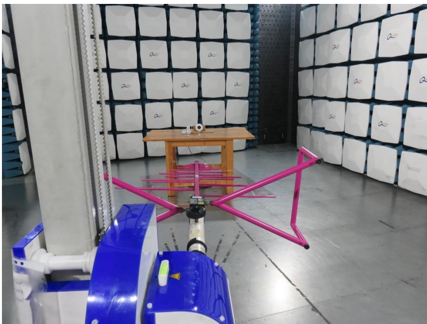
Photograph 2: Radiated Emission Testing
