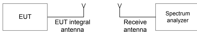
Figure 7.1.1 Setup for transmitter shut down test
