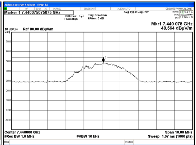
Plot 7.3.34 Radiated emission measurements at the third harmonic of high carrier frequency
