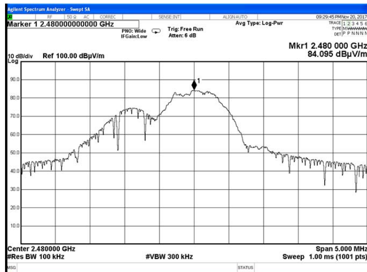
Plot 7.5.6 Peak spectral power density at high frequency in horizontal antenna polarization
