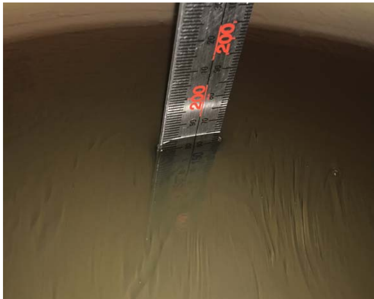
Liquid depth for SAR Measurement
