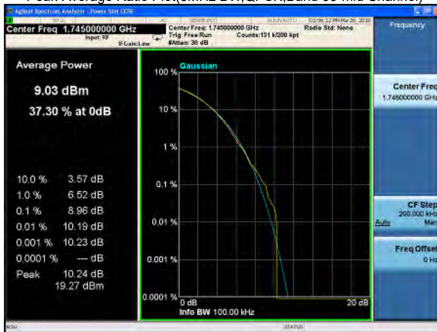
Peak-Average Ratio Plot(3MHz BW,16QAM,Band 66-mid Channel)
