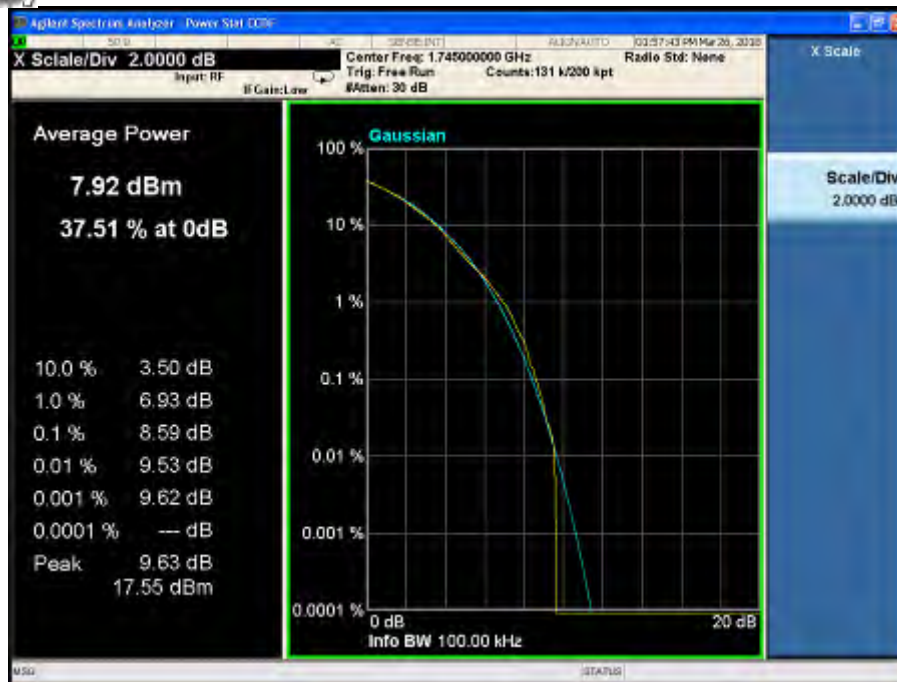
Peak-Average Ratio Plot(5MHz BW,QPSK,Band 66-mid Channel)
