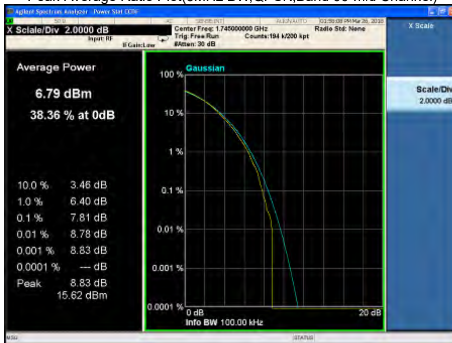
Peak-Average Ratio Plot(5MHz BW,16QAM,Band 66-mid Channel)
