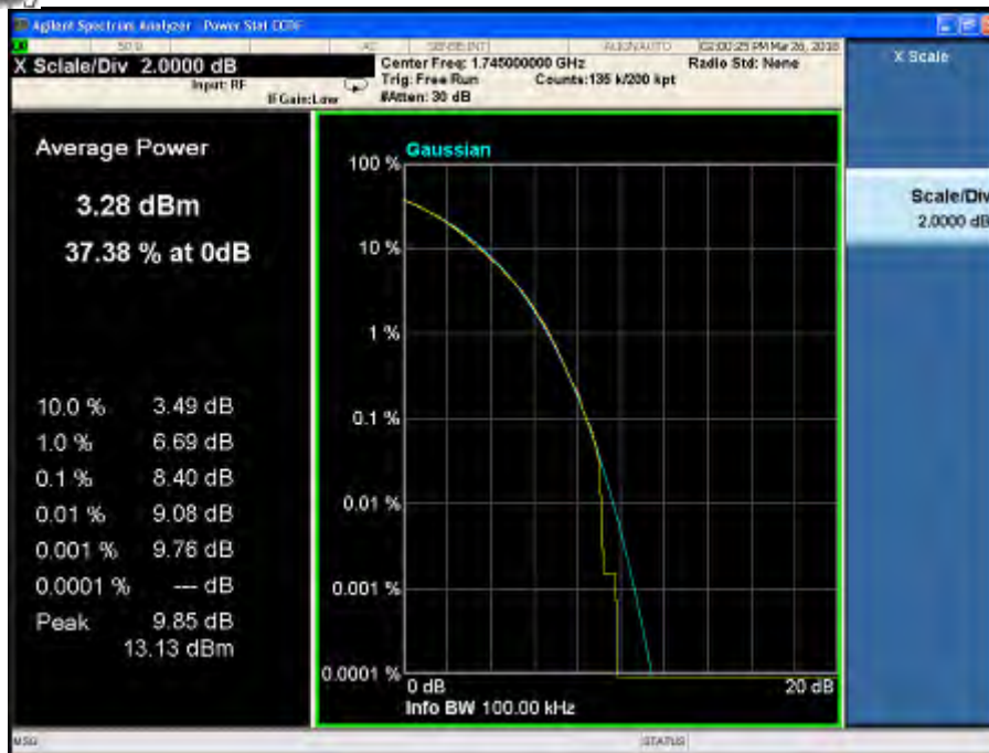
Peak-Average Ratio Plot(15MHz BW,QPSK,Band 66-mid Channel)
