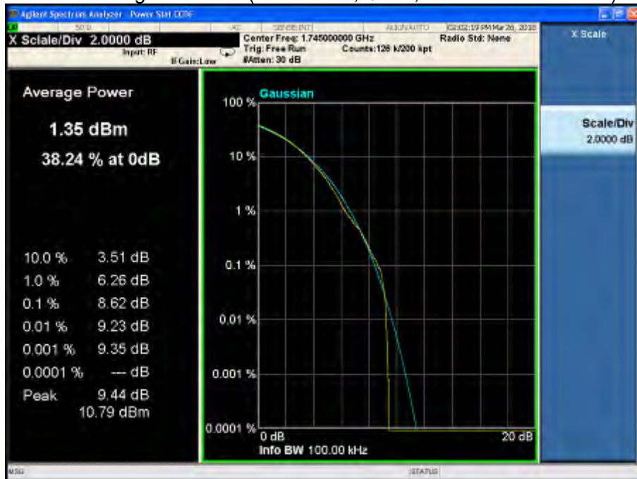
Peak-Average Ratio Plot(20MHz BW,16QAM,Band 66-mid Channel)
