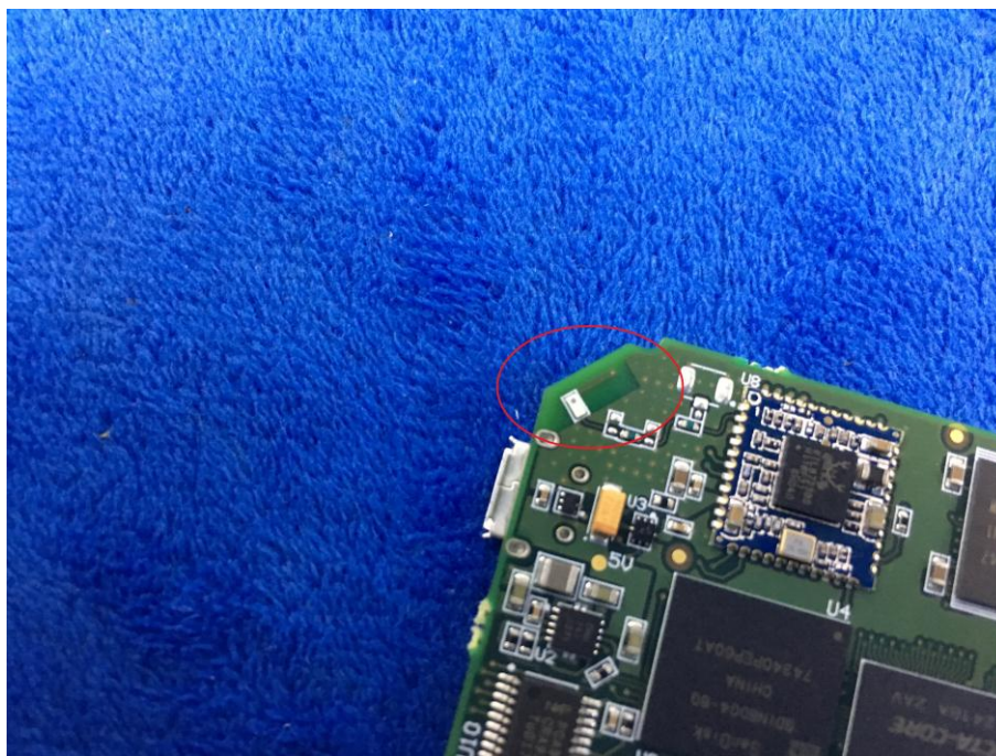
WIFI - Antenna View
