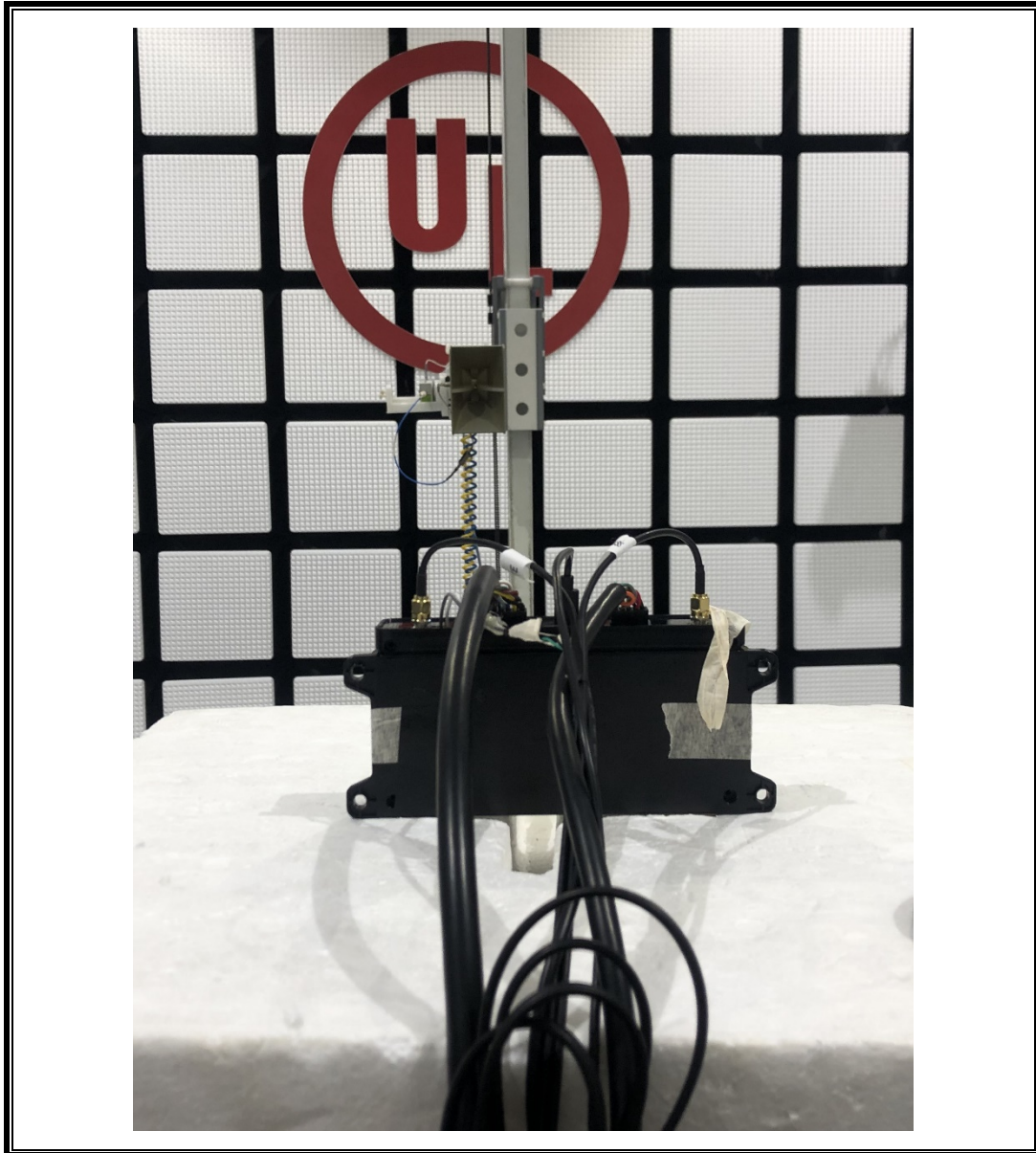
RADIATED RF MEASUREMENT SETUP (Above 1G – Z axis)
