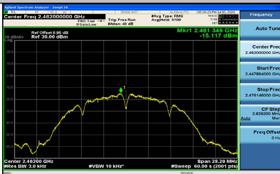
Maximum(average) power spectral density_11B_2462_Ant1
