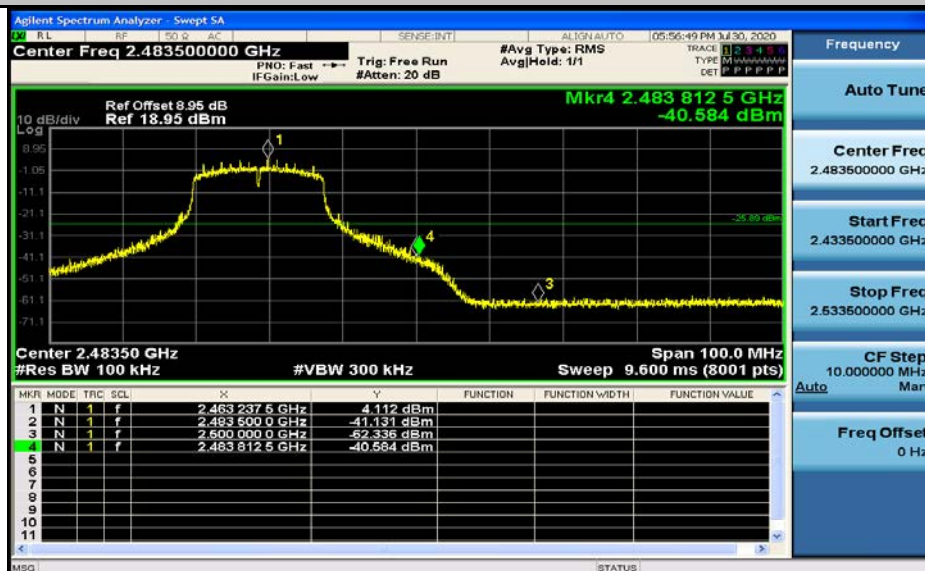
Band-edge for RF Conducted Emissions_11N20SISO_2462_Ant1
