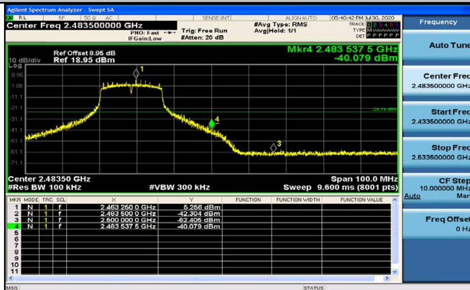
Band-edge for RF Conducted Emissions_11N20SISO_2412_Ant1
