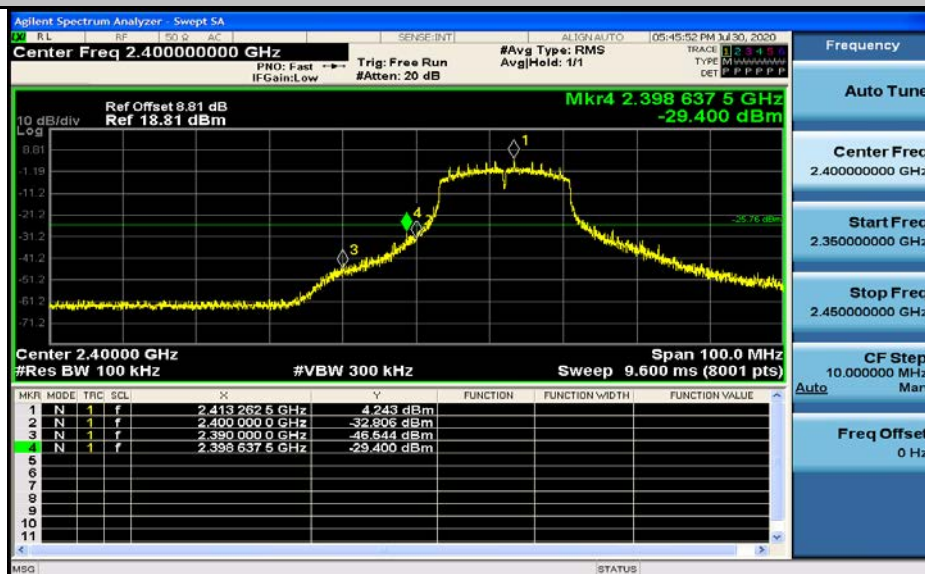
Band-edge for RF Conducted Emissions_11N20SISO_2462_Ant1
