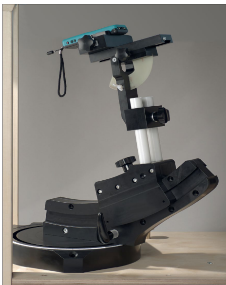
F-2. Device Holder for Transmitters
