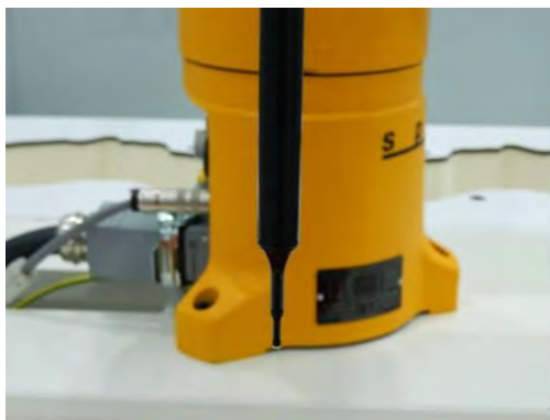
Picture 2 E-field Probe
