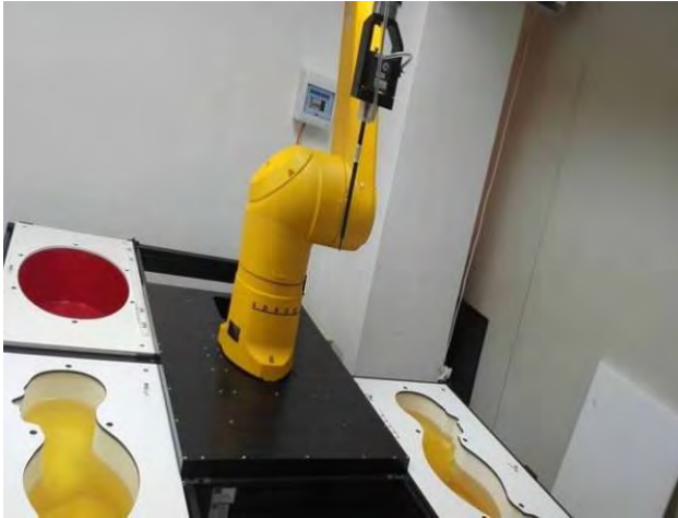
Specific Absorption Rate Test Layout
