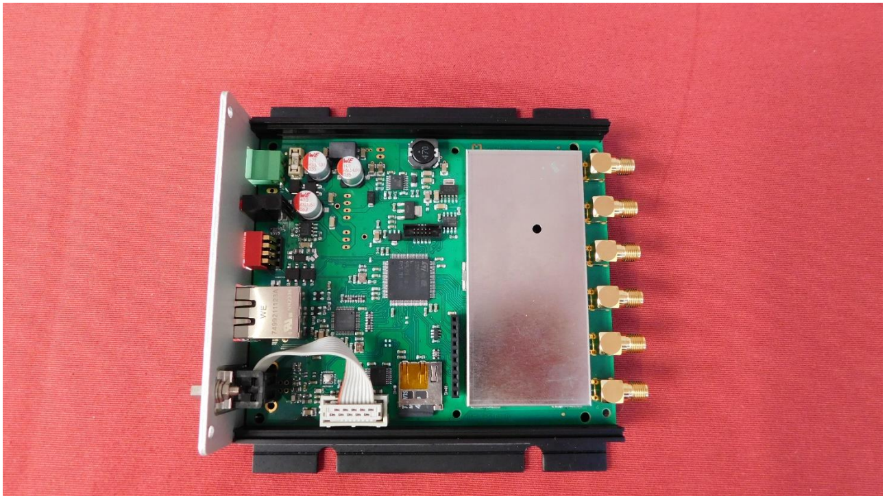
Picture 1: Top view of reading unit PCB, with shielding, inside of bottom housing
