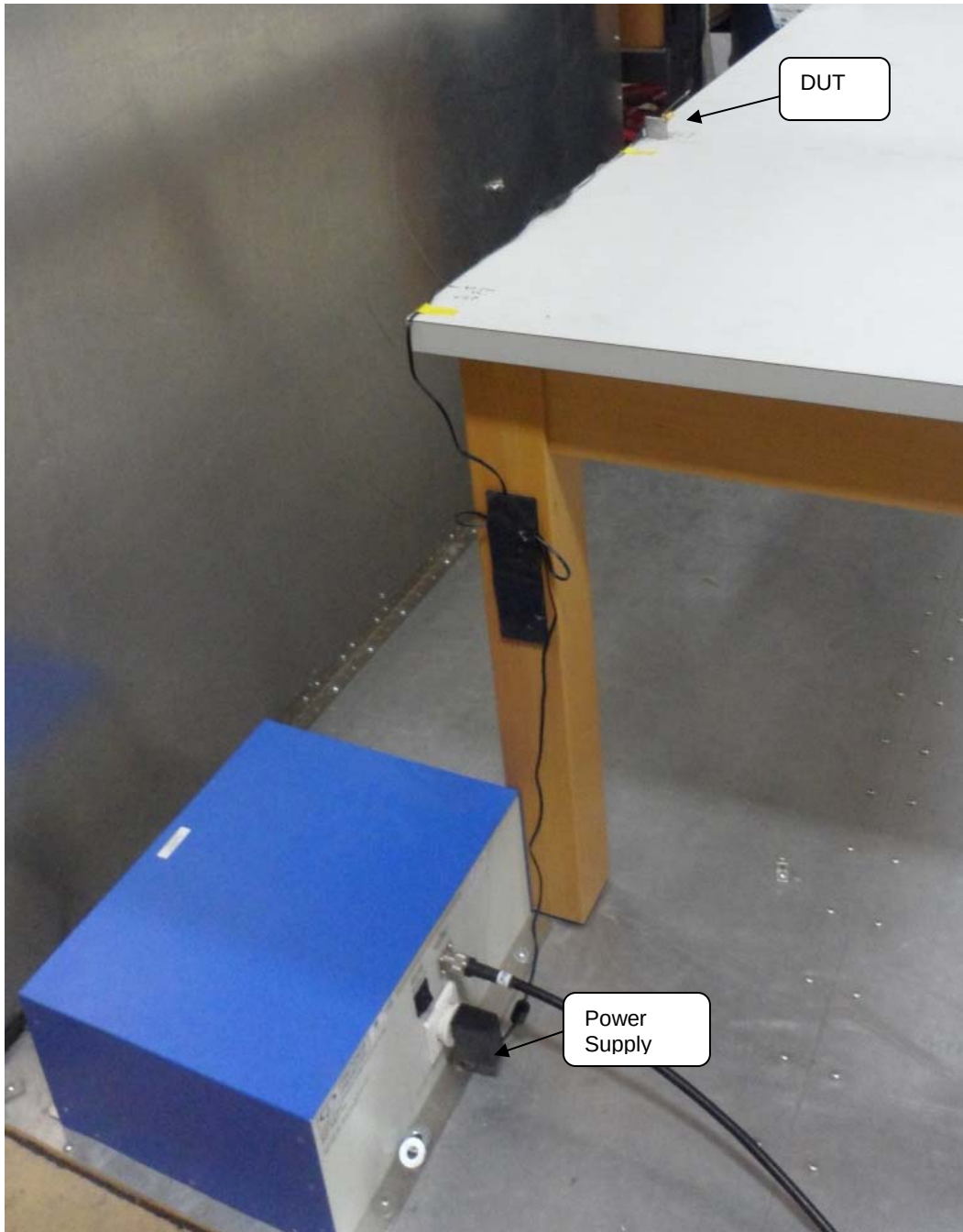
Figure E20.5 – Setup Photo – Power Line Conducted Measurements
