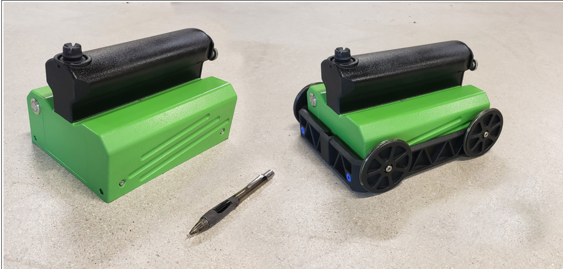
Figure 1: GPR Concrete Scanner without (left) and with (right) removable truck.
