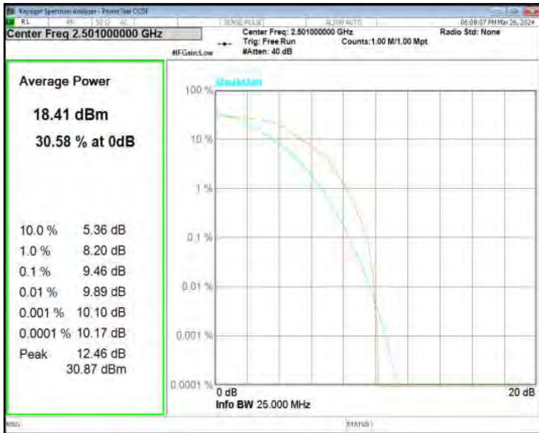
Band41 QPSK BW=5MHz Channel=40620 RB Size=1 Position=#0
