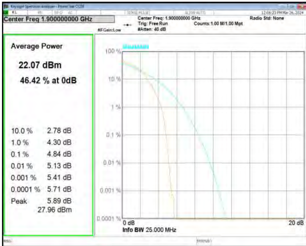
Band2 16QAM BW=20MHz Channel=18900 RB Size=1 Position=#0
