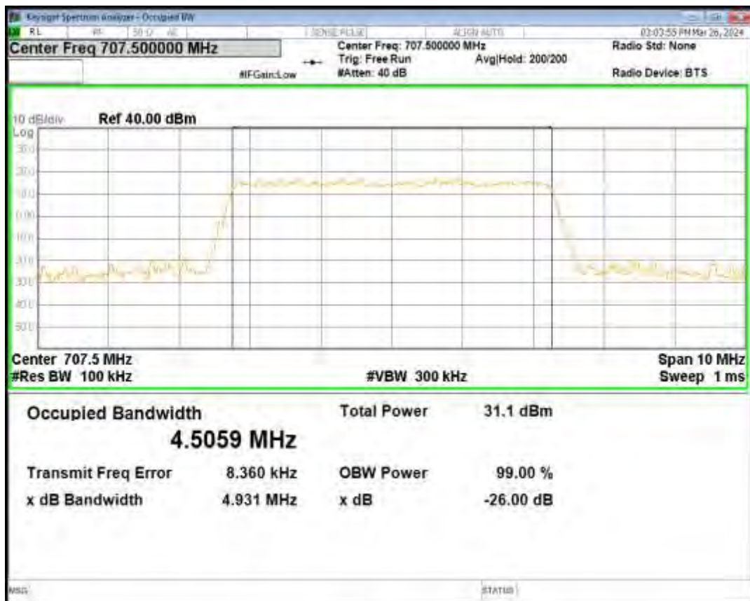
Band12 QPSK BW=10MHz Channel=23060 RB Size=50 Position=#0
