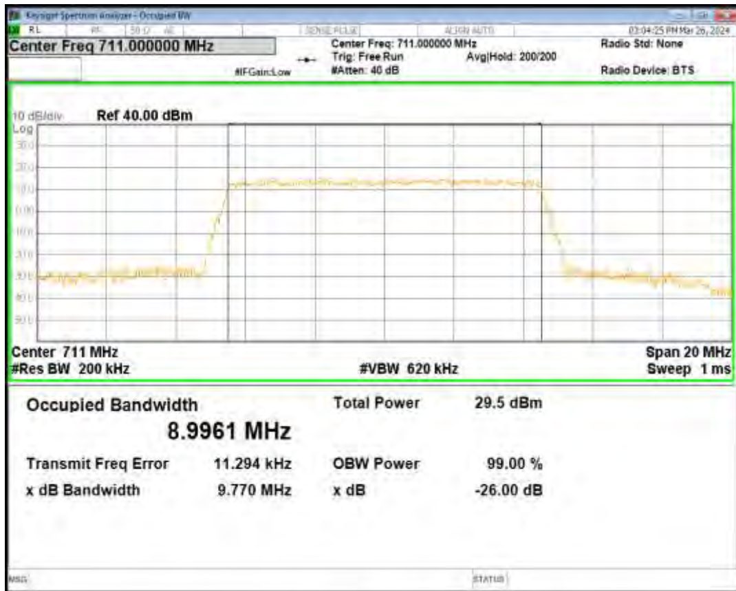
Band12 16QAM BW=10MHz Channel=23095 RB Size=50 Position=#0
