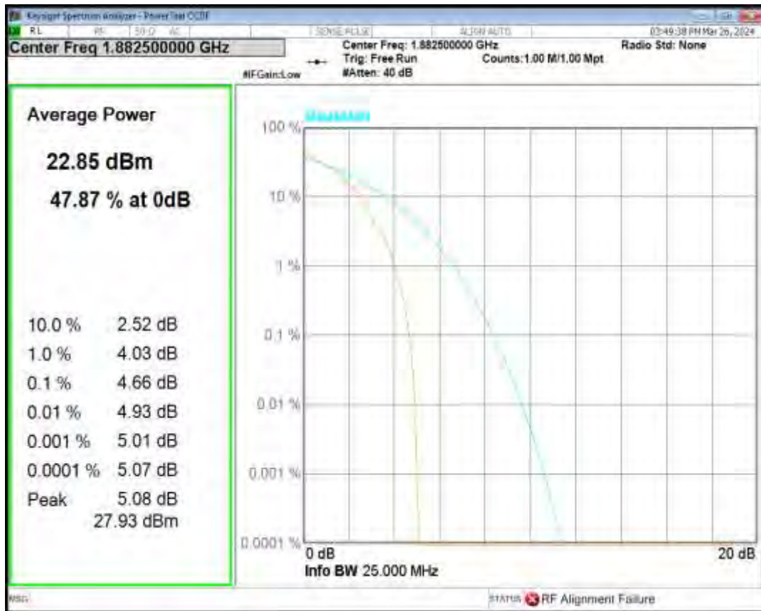
Band25 QPSK BW=10MHz Channel=26090 RB Size=1 Position=#0
