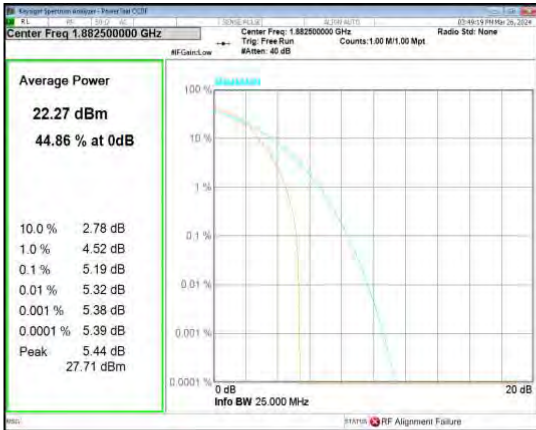
Band25 16QAM BW=5MHz Channel=26065 RB Size=1 Position=#0
