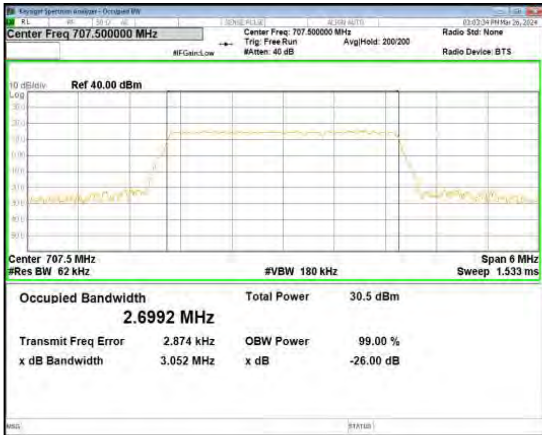
Band12 QPSK BW=5MHz Channel=23095 RB Size=25 Position=#0
