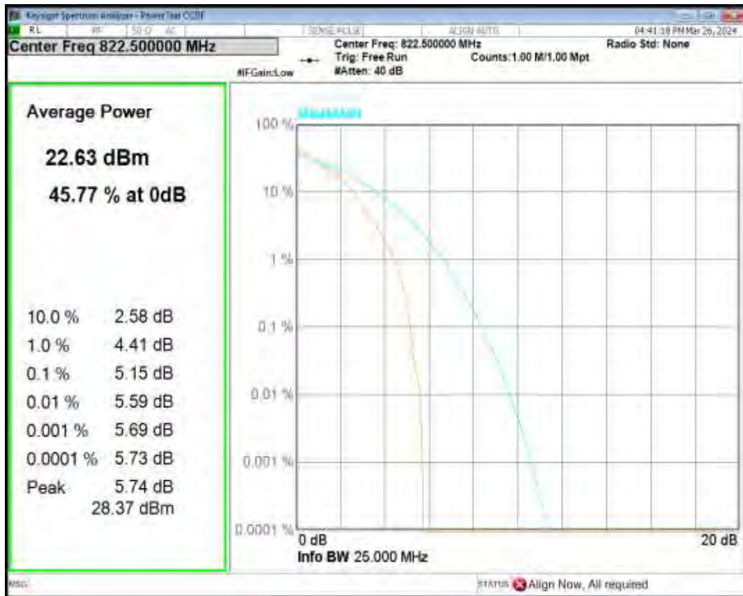
Band26(814-824) QPSK BW=5MHz Channel=26715 RB Size=1 Position=#0
