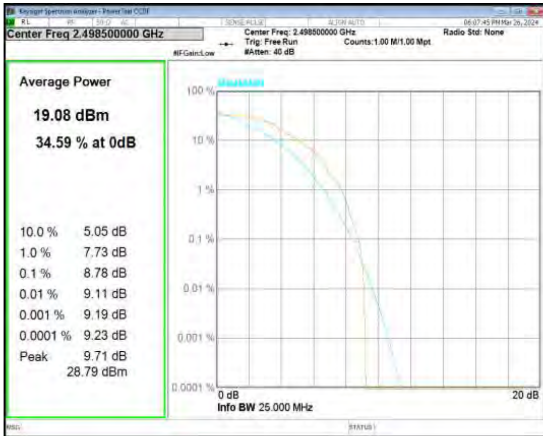
Band41 QPSK BW=20MHz Channel=41490 RB Size=1 Position=#0
