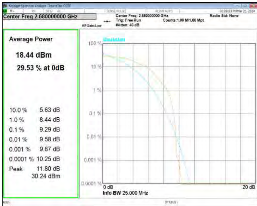
Band41 16QAM BW=20MHz Channel=40620 RB Size=1 Position=#0
