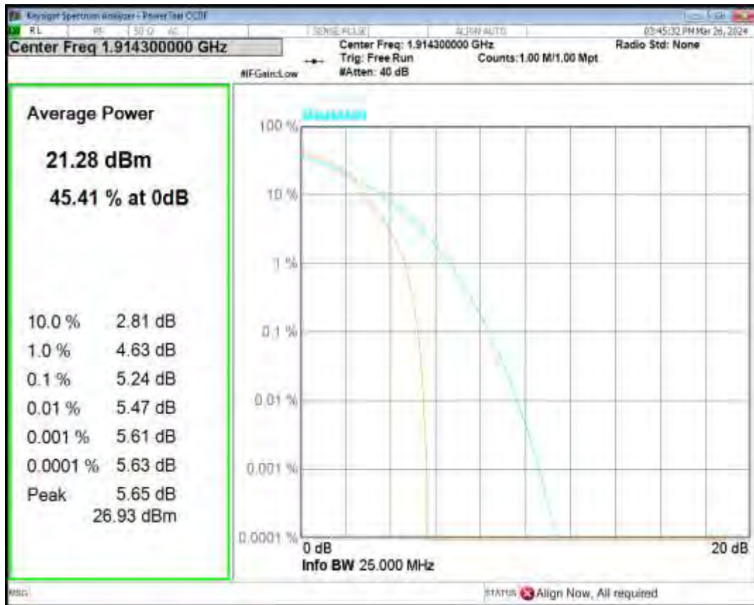
Band25 16QAM BW=10MHz Channel=26090 RB Size=1 Position=#0
