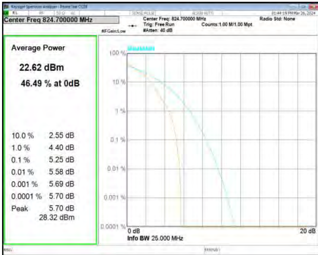
Band5 QPSK BW=5MHz Channel=20525 RB Size=1 Position=#0
