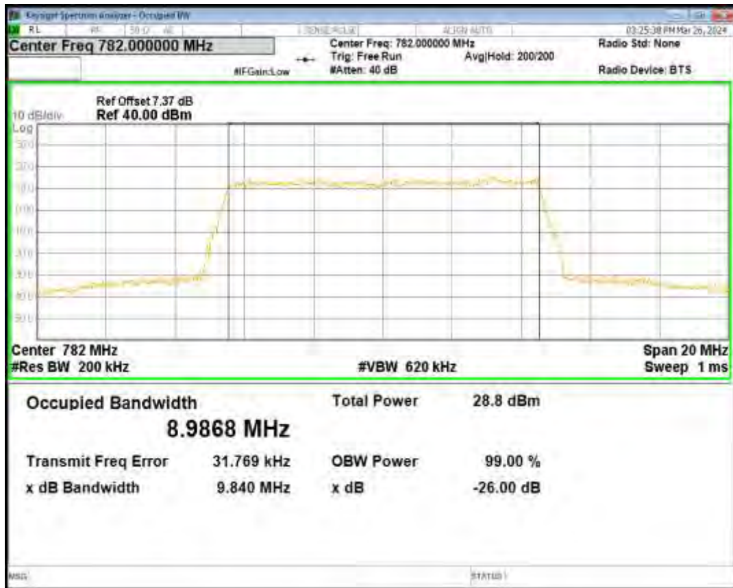
Band13 16QAM BW=5MHz Channel=23205 RB Size=25 Position=#0
