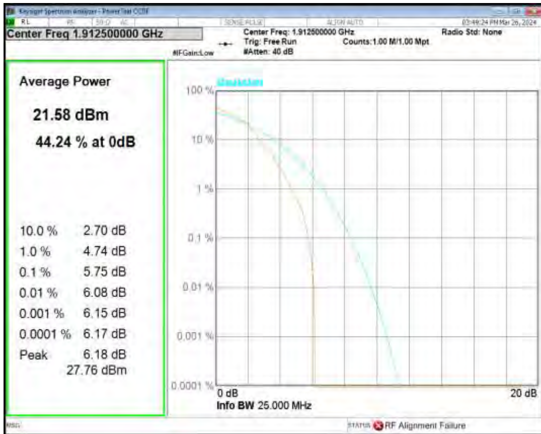
Band25 16QAM BW=3MHz Channel=26365 RB Size=1 Position=#0
