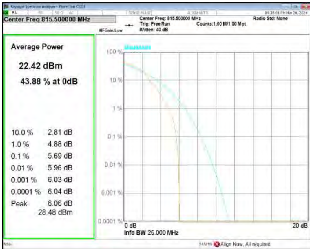
Band26(814-824) 16QAM BW=10MHz Channel=26740 RB Size=1 Position=#0
