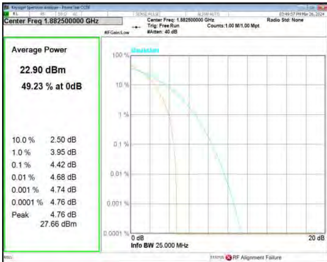
Band25 QPSK BW=15MHz Channel=26115 RB Size=1 Position=#0
