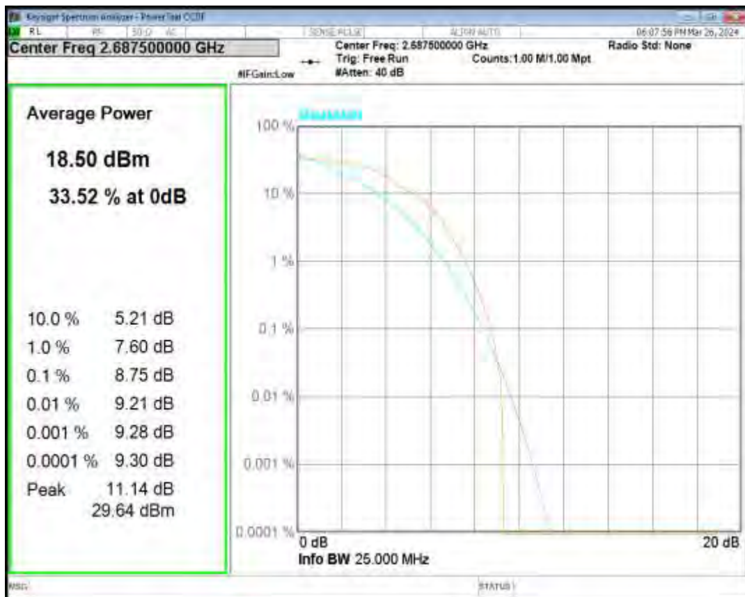
Band5 16QAM BW=1.4MHz Channel=20407 RB Size=1 Position=#0
