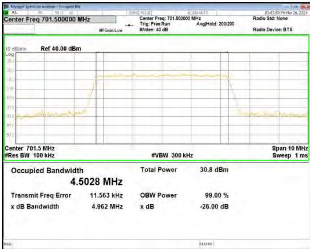
Band12 QPSK BW=5MHz Channel=23155 RB Size=25 Position=#0
