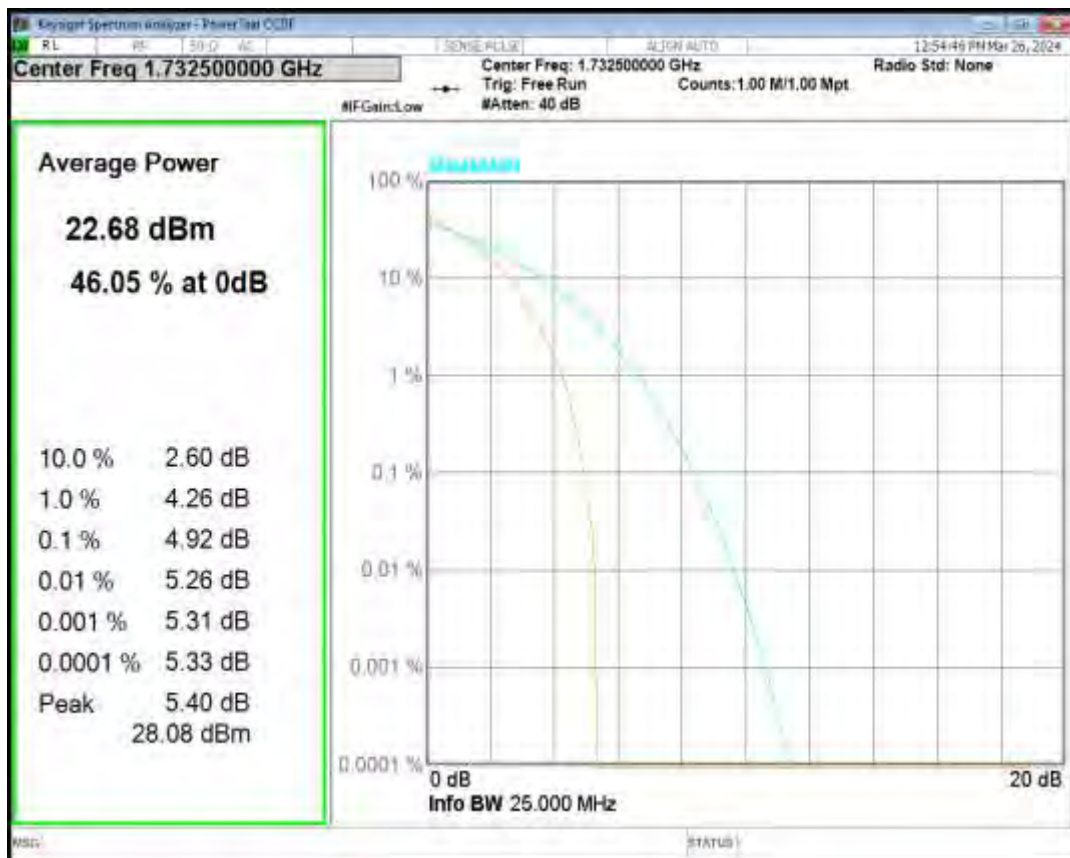
Band4 QPSK BW=20MHz Channel=20050 RB Size=1 Position=#0
