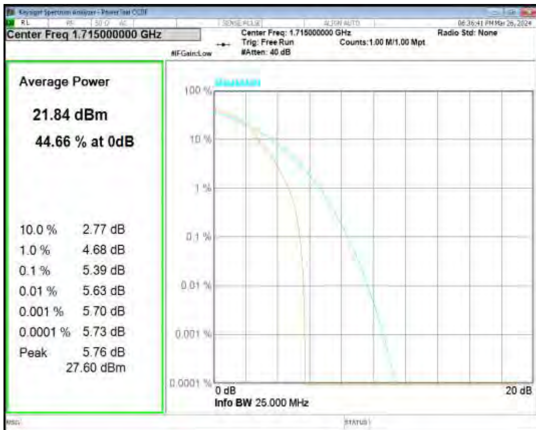
Band66 16QAM BW=10MHz Channel=132322 RB Size=1 Position=#0
