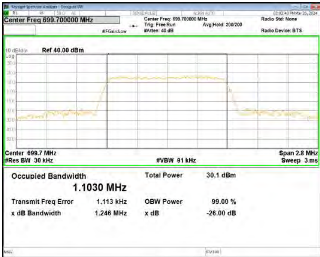
Band12 16QAM BW=1.4MHz Channel=23095 RB Size=6 Position=#0
