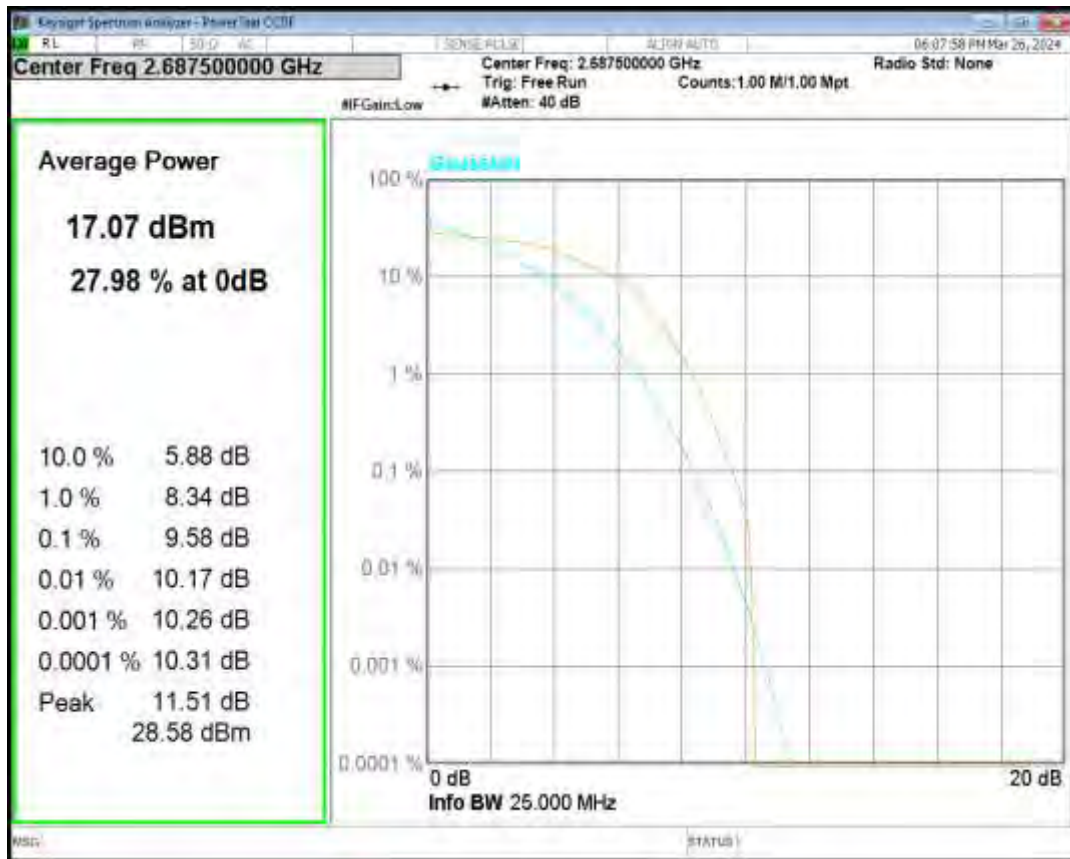
Band41 16QAM BW=15MHz Channel=40620 RB Size=1 Position=#0
