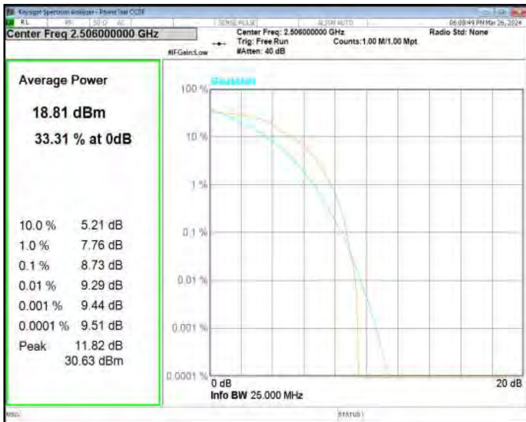
Band41 QPSK BW=15MHz Channel=41515 RB Size=1 Position=#0
