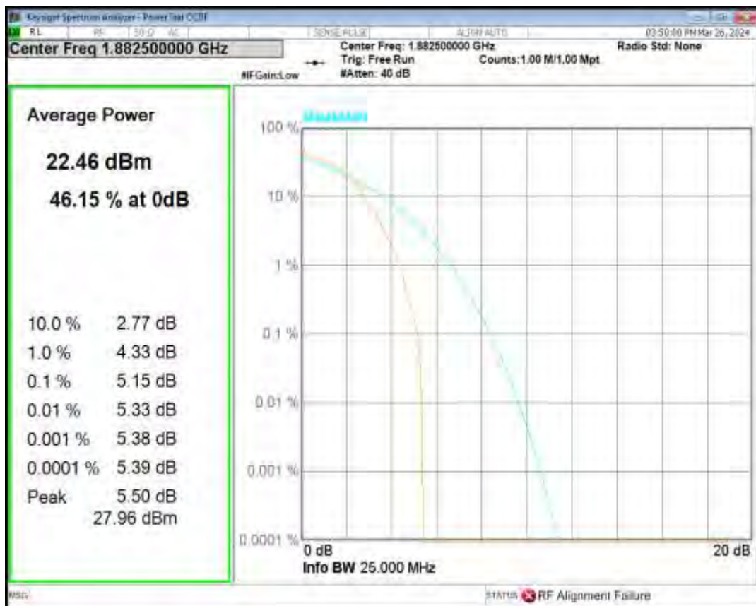
Band25 16QAM BW=15MHz Channel=26615 RB Size=1 Position=#0
