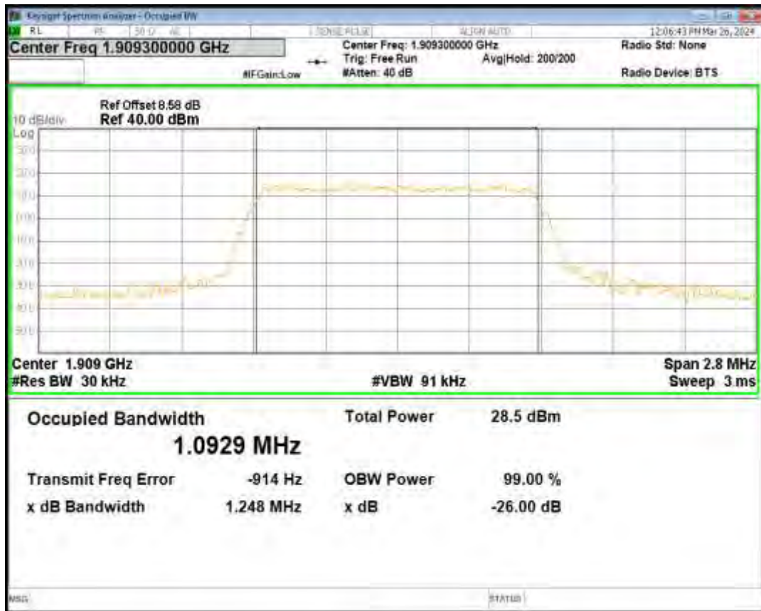
Band2 16QAM BW=10MHz Channel=18650 RB Size=50 Position=#0
