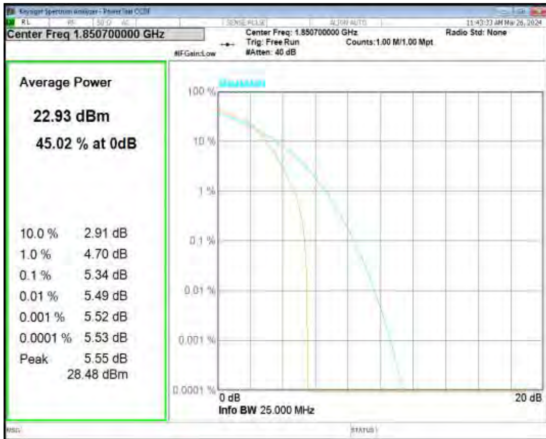
Band2 16QAM BW=1.4MHz Channel=18900 RB Size=1 Position=#0
