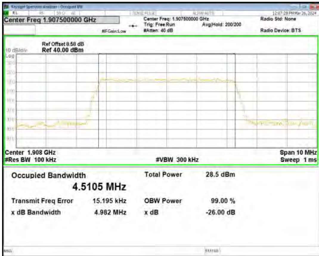
Band2 16QAM BW=3MHz Channel=18615 RB Size=15 Position=#0
