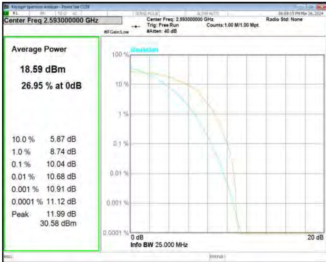
Band41 16QAM BW=15MHz Channel=41515 RB Size=1 Position=#0
