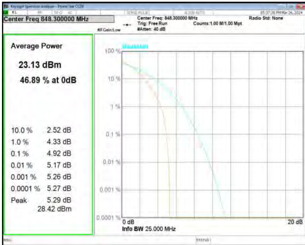
Band26(824-849) QPSK BW=1.4MHz Channel=26915 RB Size=1 Position=#0
