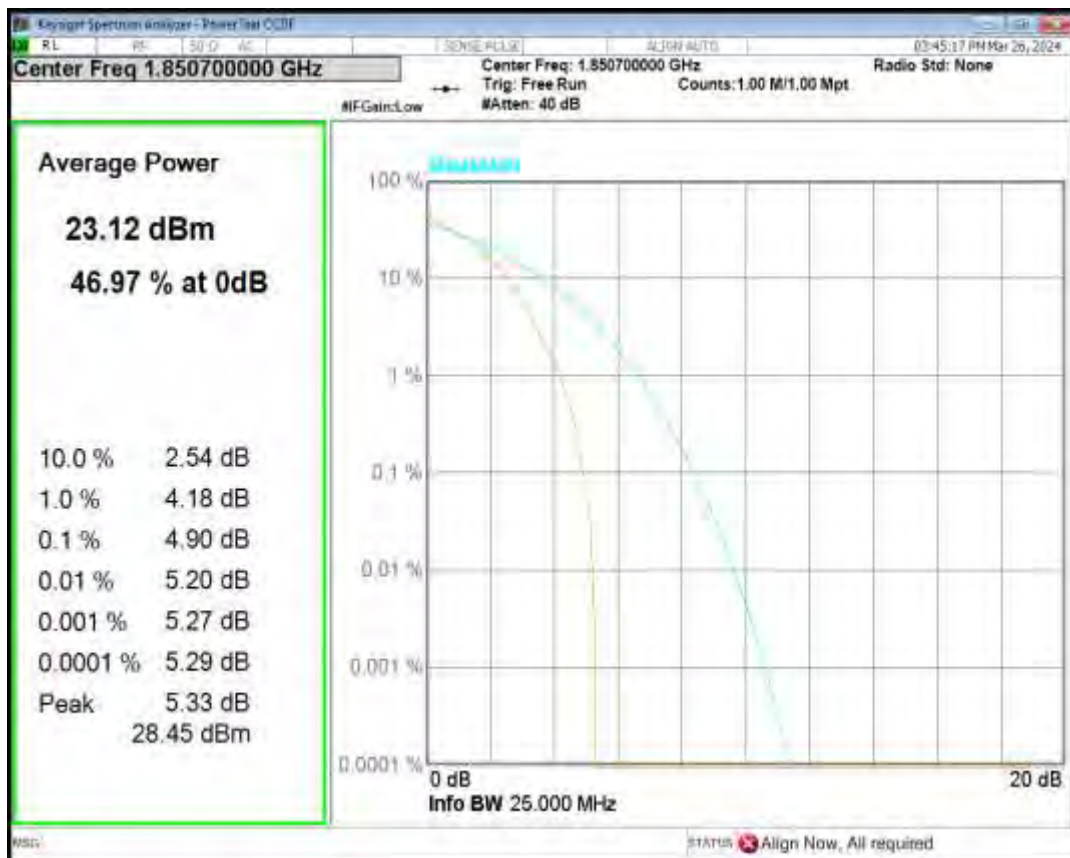
Band25 16QAM BW=5MHz Channel=26365 RB Size=1 Position=#0
