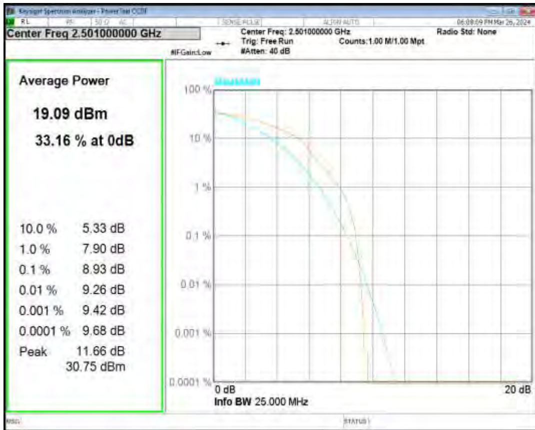
Band41 16QAM BW=5MHz Channel=40620 RB Size=1 Position=#0
