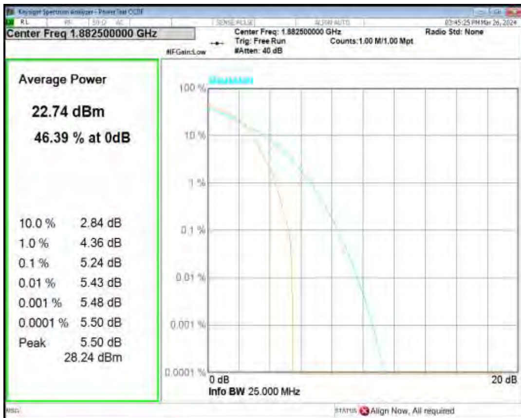
Band25 16QAM BW=1.4MHz Channel=26683 RB Size=1 Position=#0
