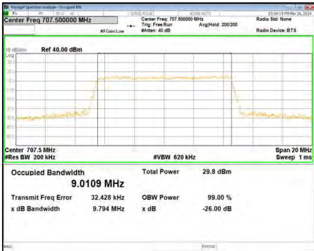
Band12 16QAM BW=10MHz Channel=23060 RB Size=50 Position=#0
