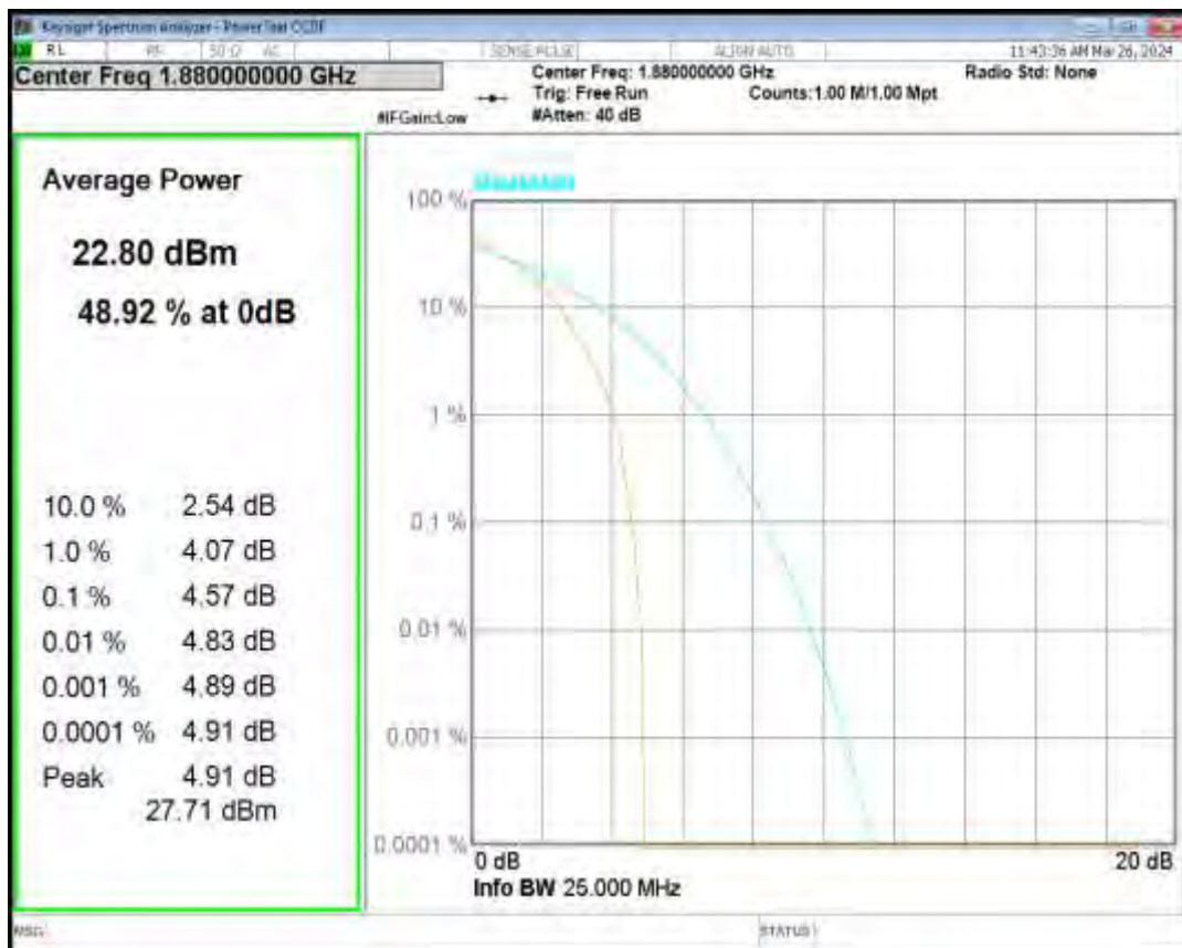
Band2 QPSK BW=1.4MHz Channel=18607 RB Size=1 Position=#0
