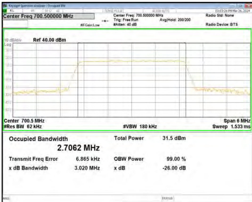
Band12 QPSK BW=3MHz Channel=23095 RB Size=15 Position=#0
