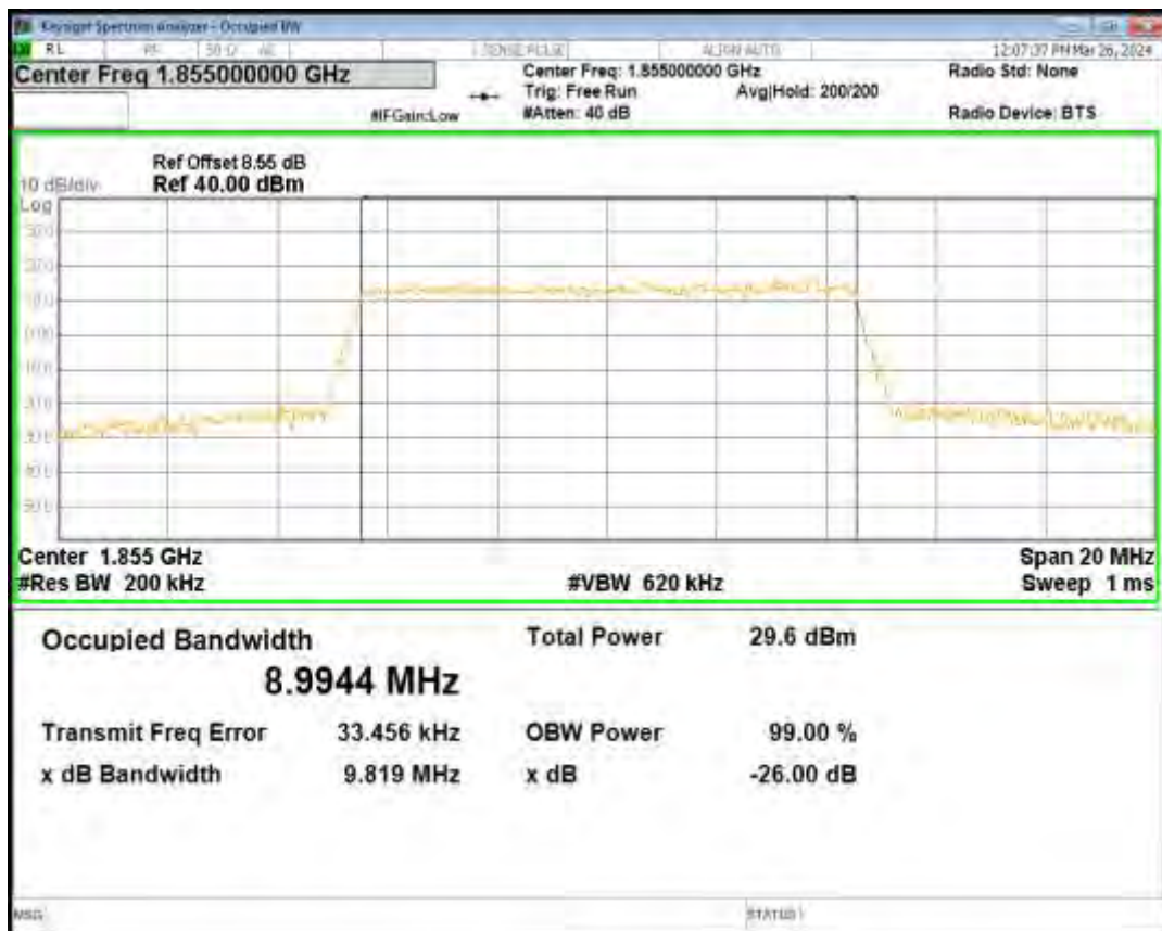
Band2 16QAM BW=10MHz Channel=18900 RB Size=50 Position=#0
