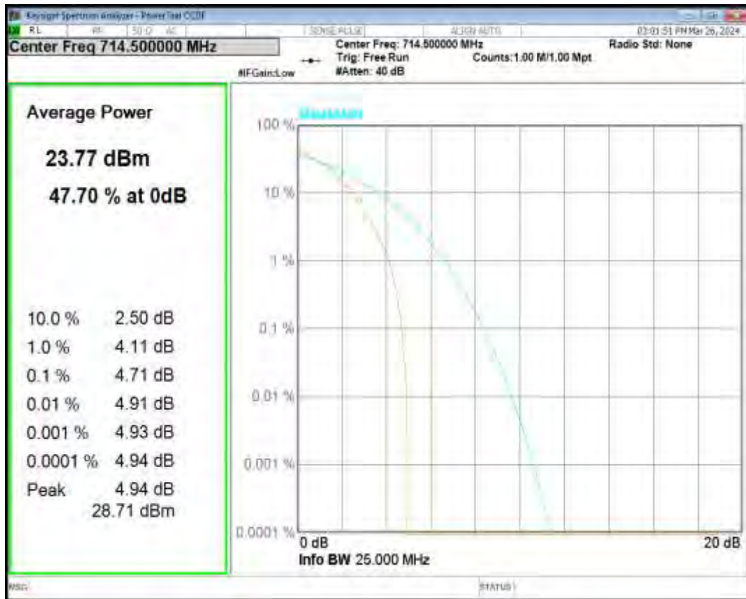
Band12 QPSK BW=5MHz Channel=23035 RB Size=1 Position=#0
