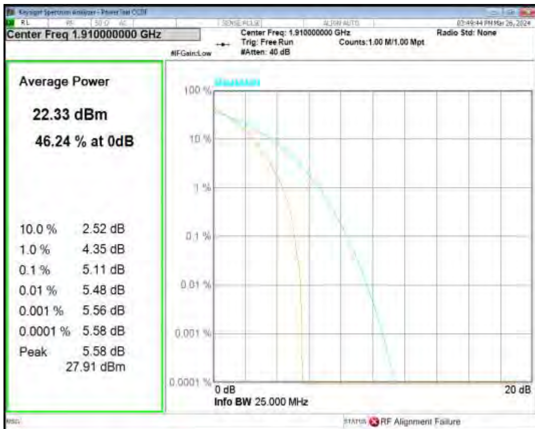
Band25 QPSK BW=10MHz Channel=26365 RB Size=1 Position=#0
