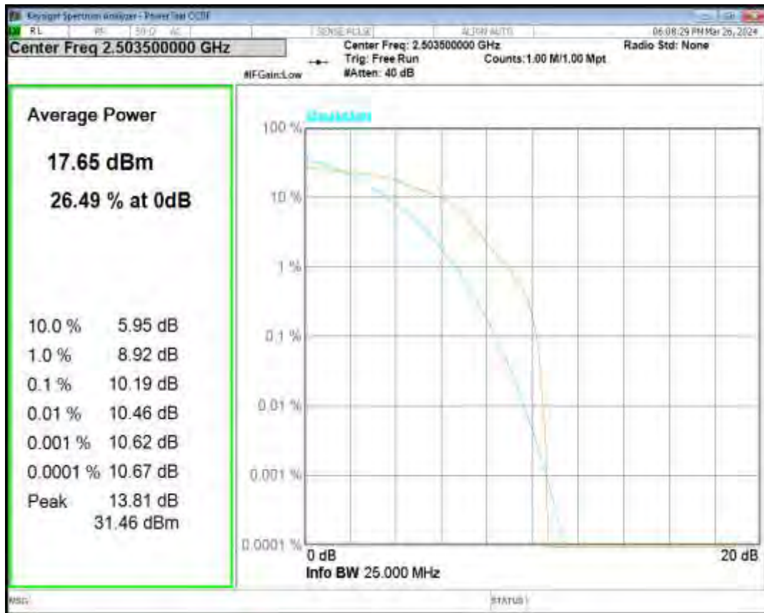
Band41 16QAM BW=10MHz Channel=41540 RB Size=1 Position=#0
