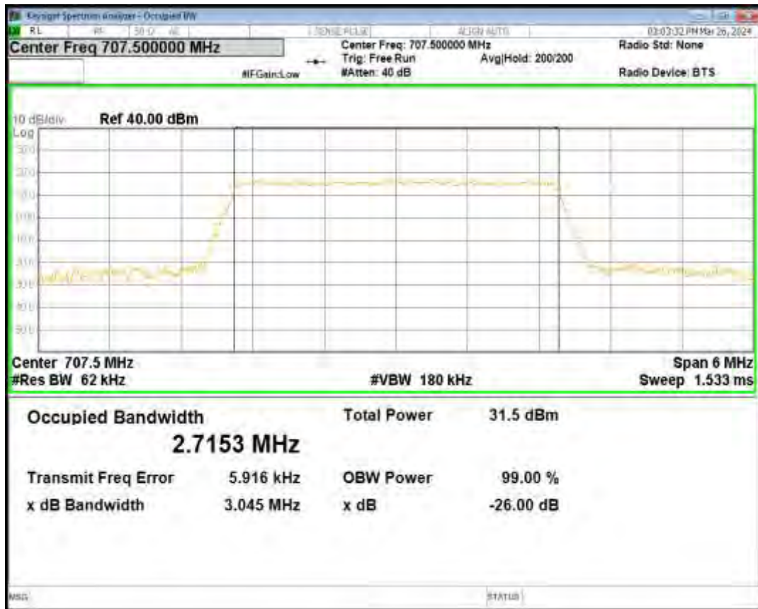
Band12 QPSK BW=3MHz Channel=23165 RB Size=15 Position=#0
