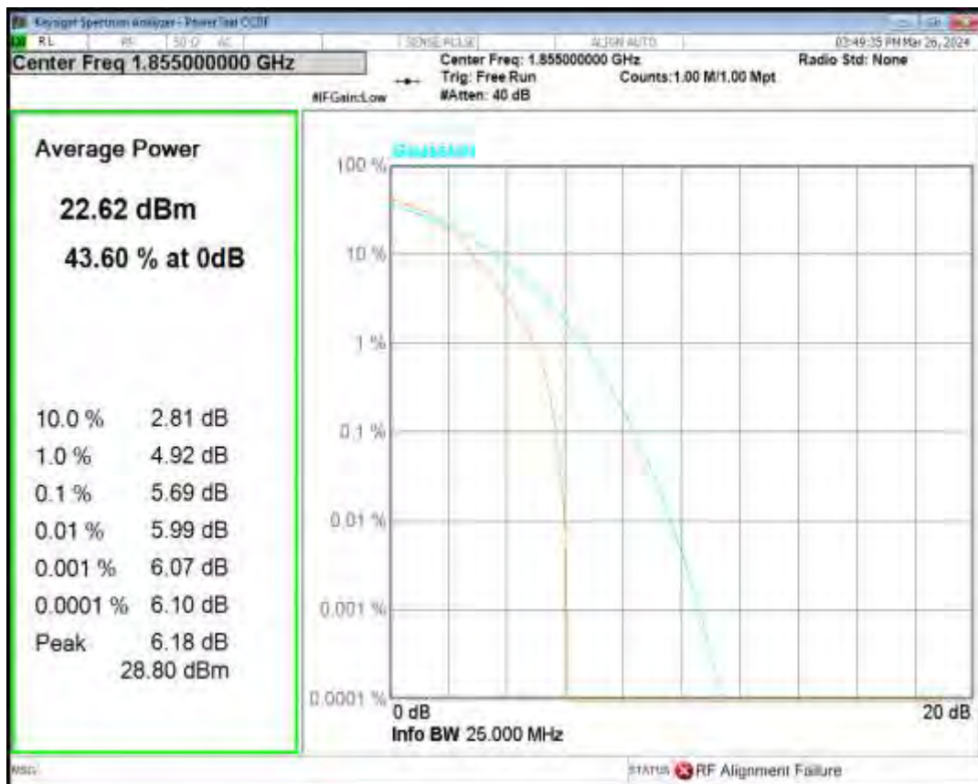
Band25 16QAM BW=10MHz Channel=26365 RB Size=1 Position=#0
