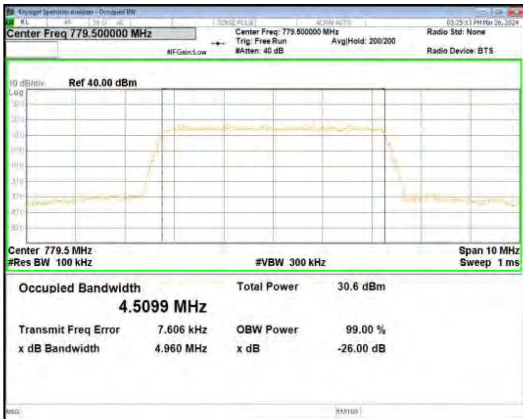
Band13 QPSK BW=5MHz Channel=23230 RB Size=25 Position=#0
