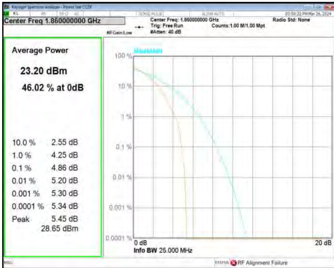
Band25 QPSK BW=15MHz Channel=26365 RB Size=1 Position=#0
