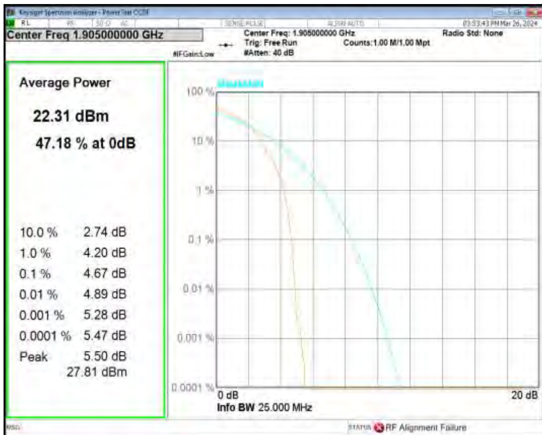
Band25 16QAM BW=20MHz Channel=26365 RB Size=1 Position=#0
