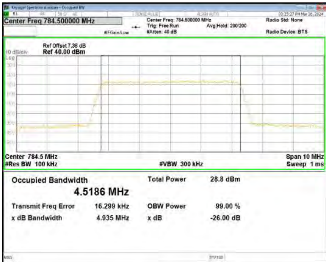
Band13 QPSK BW=10MHz Channel=23230 RB Size=50 Position=#0
