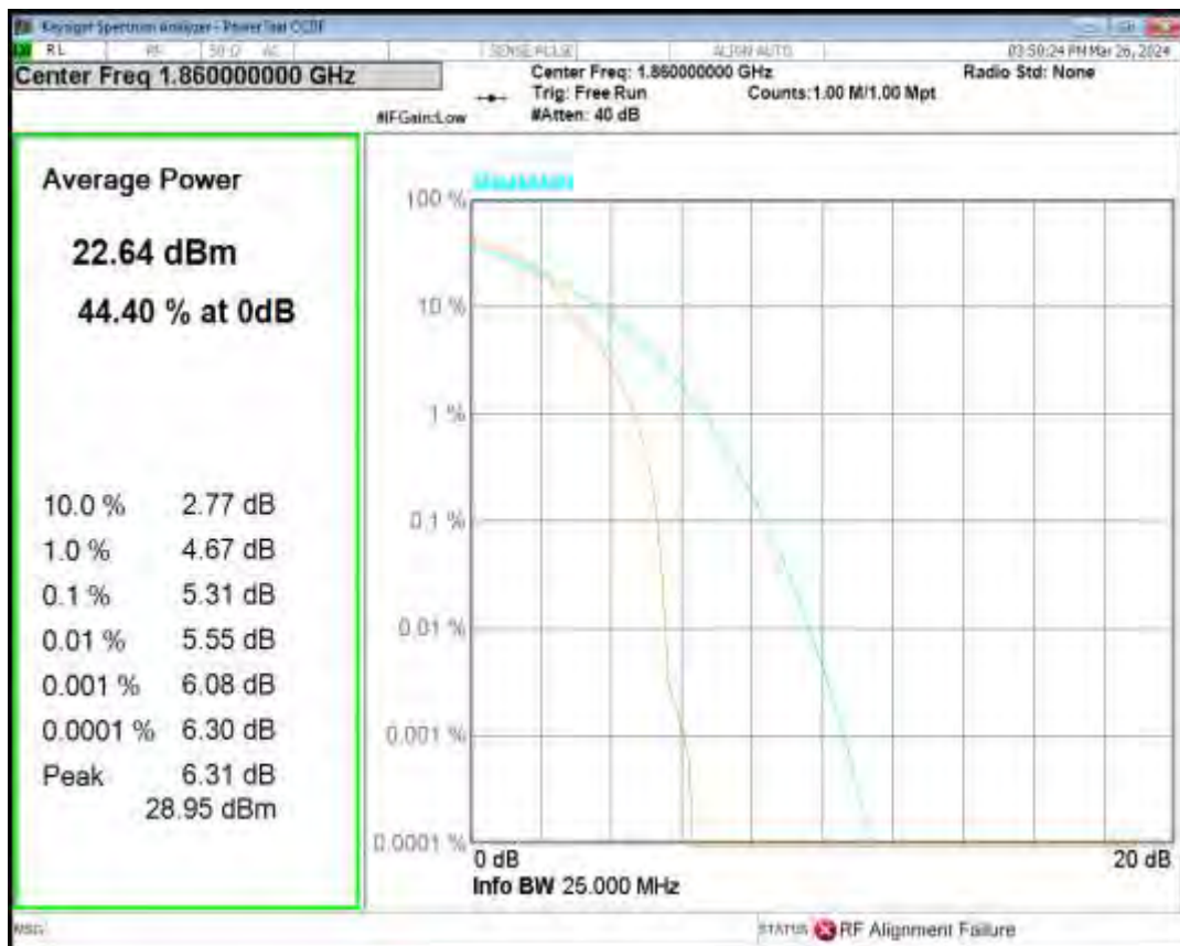
Band25 16QAM BW=3MHz Channel=26675 RB Size=1 Position=#0
