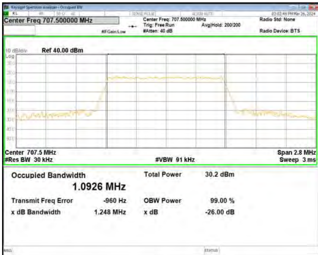
Band12 QPSK BW=1.4MHz Channel=23173 RB Size=6 Position=#0
