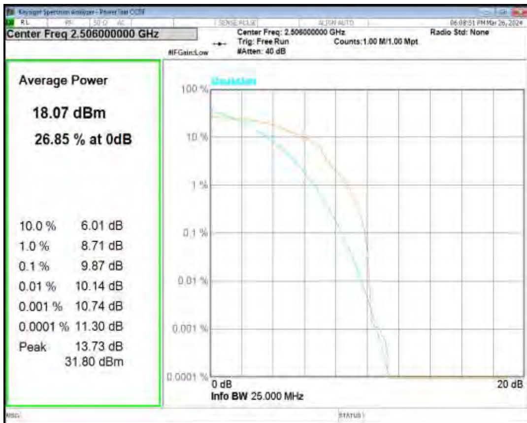
Band41 16QAM BW=5MHz Channel=41565 RB Size=1 Position=#0
