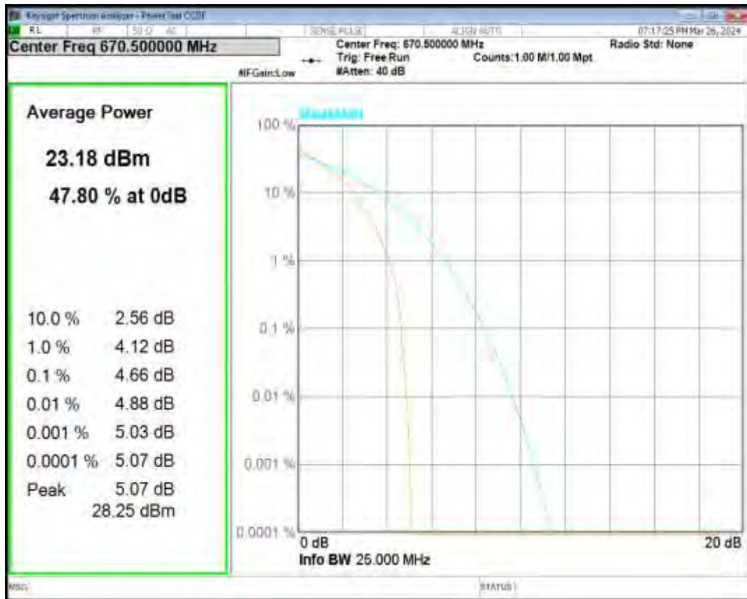
Band71 QPSK BW=15MHz Channel=133297 RB Size=1 Position=#0
