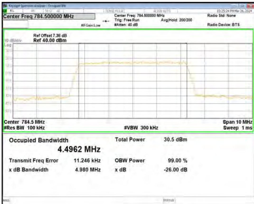
Band2 16QAM BW=1.4MHz Channel=18607 RB Size=6 Position=#0
