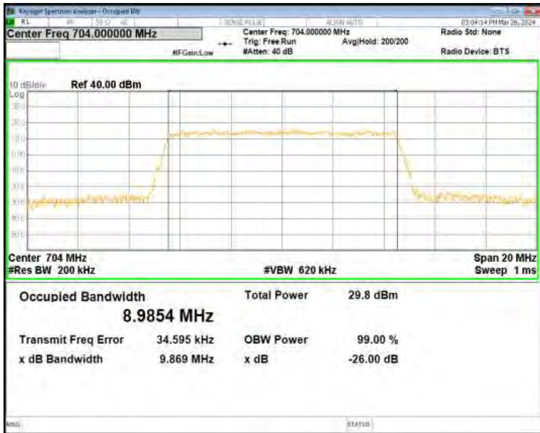
Band12 16QAM BW=1.4MHz Channel=23173 RB Size=6 Position=#0
