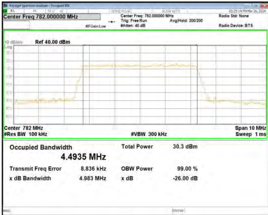
Band13 QPSK BW=5MHz Channel=23255 RB Size=25 Position=#0
