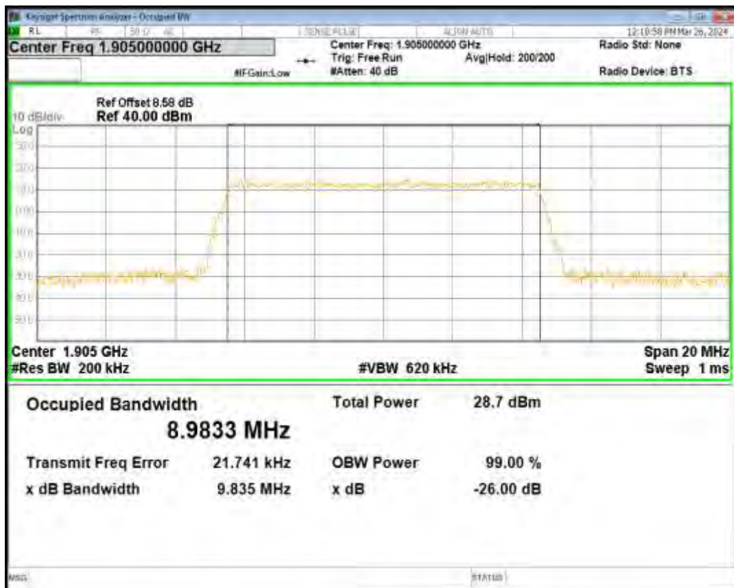
Band2 16QAM BW=15MHz Channel=18675 RB Size=75 Position=#0
