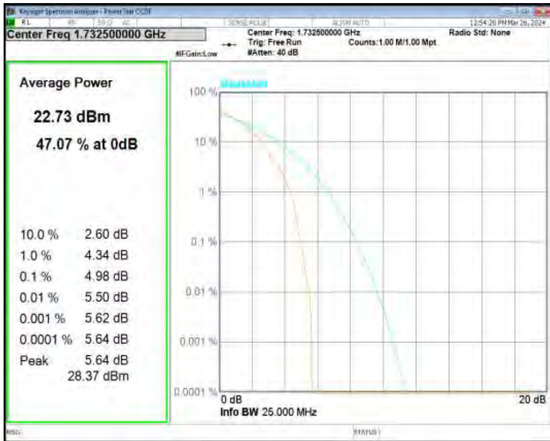
Band4 QPSK BW=3MHz Channel=20385 RB Size=1 Position=#0
