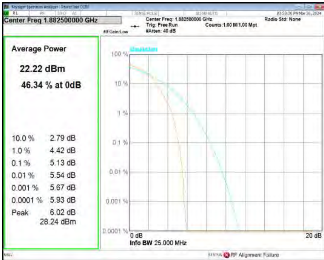
Band25 16QAM BW=20MHz Channel=26140 RB Size=1 Position=#0
