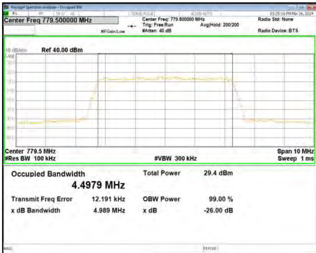
Band13 16QAM BW=5MHz Channel=23230 RB Size=25 Position=#0
