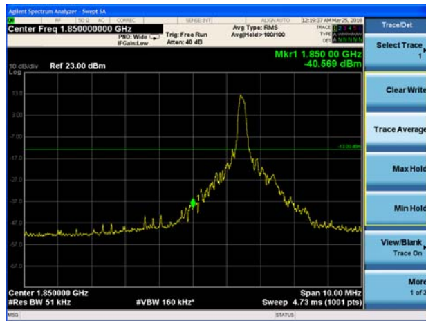
LTE Band 2 20MHz 16QAM 100%RB CH-Low
