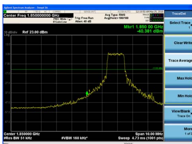
LTE Band 2 20MHz QPSK 100%RB CH-Low
