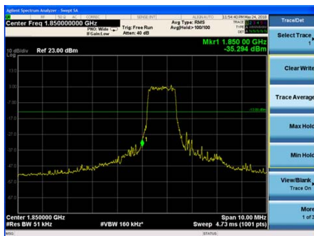
LTE Band 2 5MHz QPSK 100%RB CH-Low
