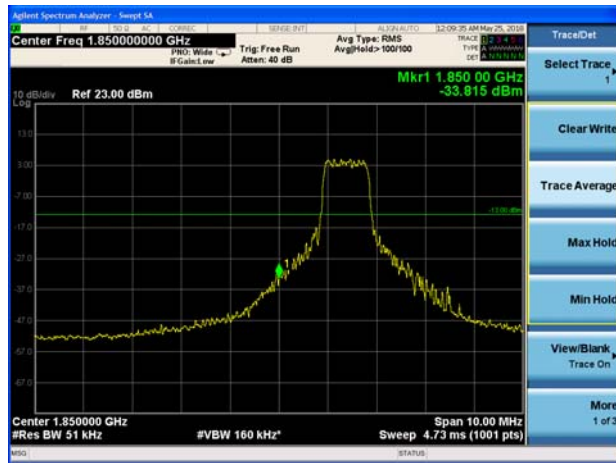
LTE Band 2 20MHz 16QAM 1RB CH-Low
