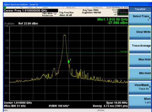
LTE Band 2 5MHz QPSK 100%RB CH-High
