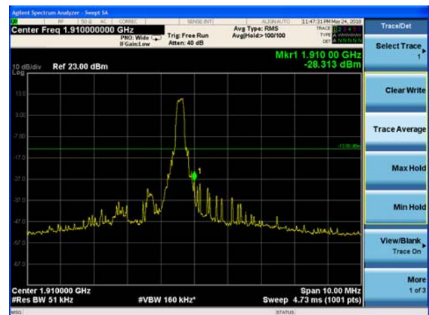
LTE Band 2 3MHz QPSK 1RB CH-High
