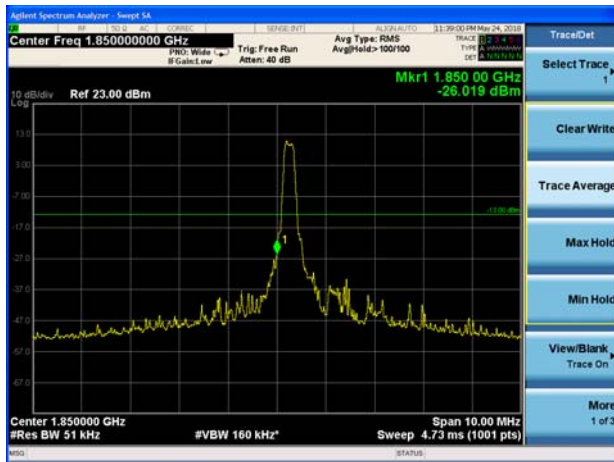
LTE Band 2 1.4MHz QPSK 100%RB CH-Low
