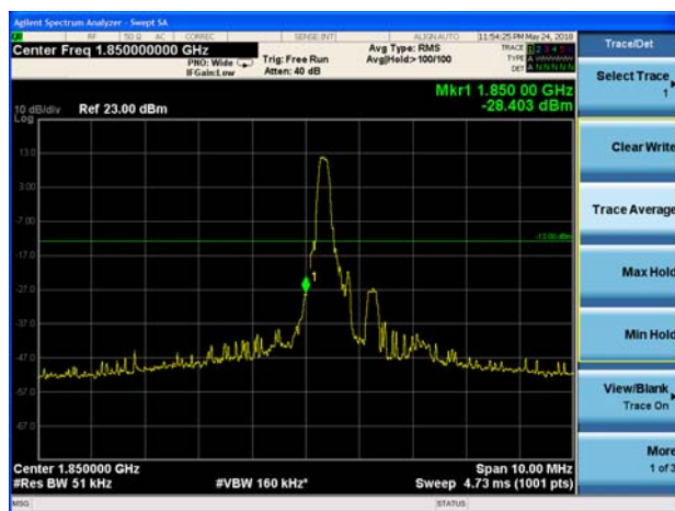
LTE Band 2 5MHz 16QAM 100%RB CH-Low
