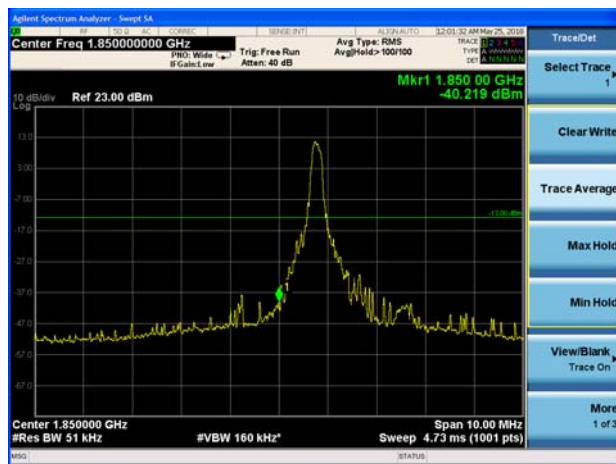
LTE Band 2 10MHz 16QAM 100%RB CH-Low
