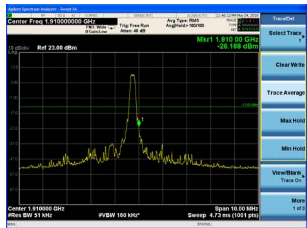
LTE Band 2 1.4MHz 16QAM 100%RB CH-High
