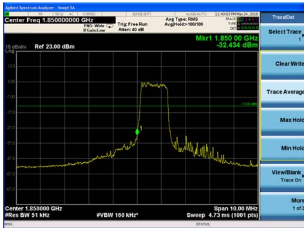
LTE Band 2 3MHz QPSK 1RB CH-Low
