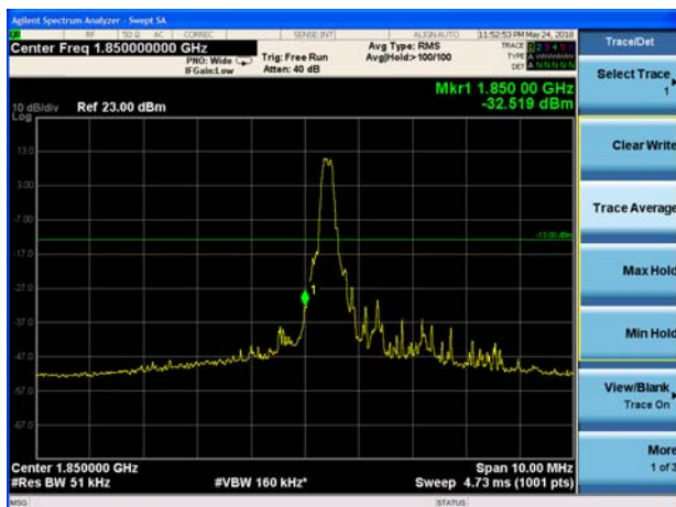
LTE Band 2 3MHz QPSK 1RB CH-Low
