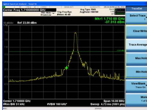
LTE Band 4 16QAM 10MHz CH-Low, 100%RB
