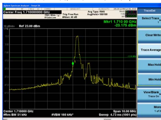
LTE Band 4 16QAM 5MHz CH-Low, 100%RB
