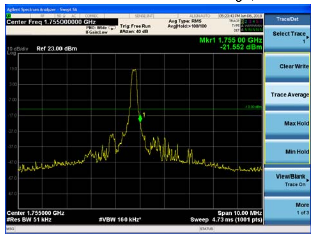
LTE Band 4 QPSK 1.4MHz CH-High, 100%RB
