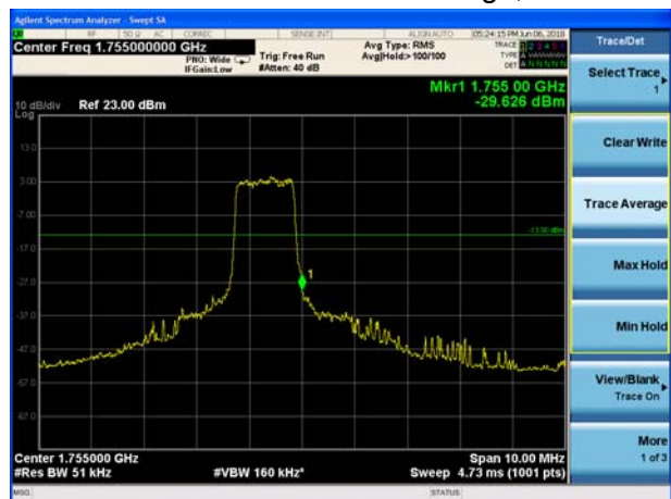
LTE Band 4 QPSK 3MHz CH-High, 1 RB
