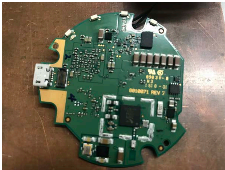
main PCB, top side with Bluetooth SoC
