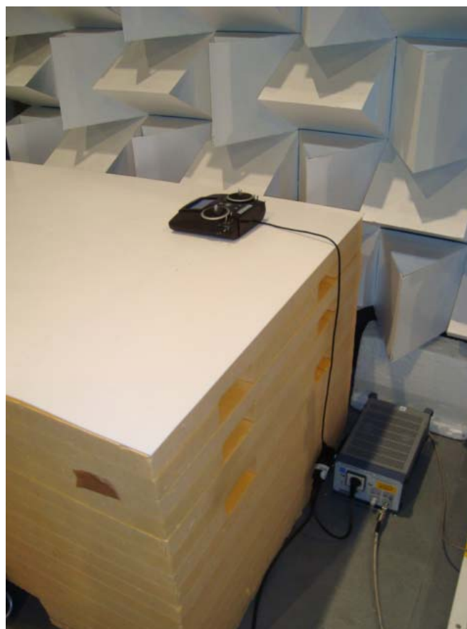
Figure 4 EUT / test set up - spurious conducted emissions
