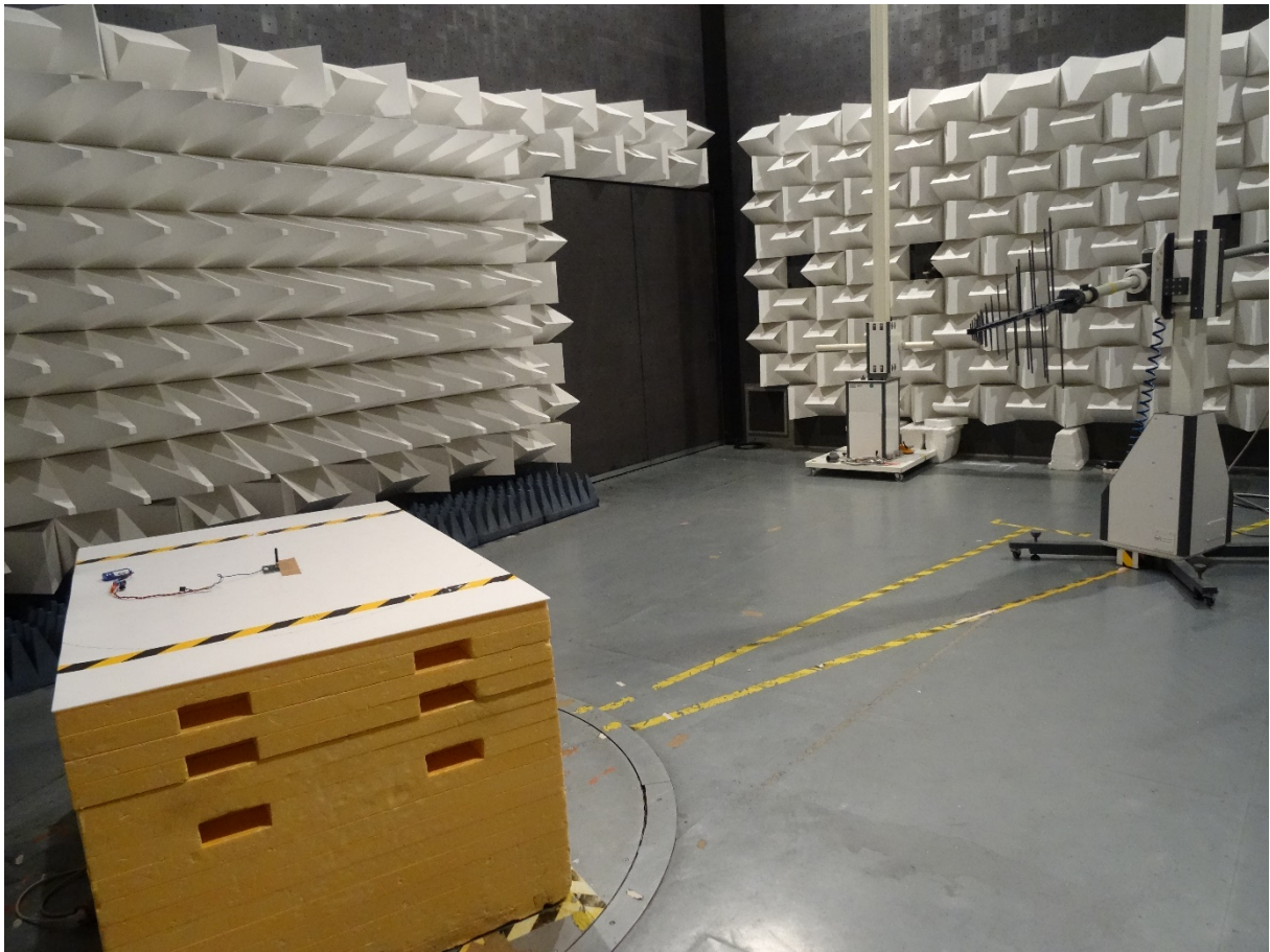
TX radiated emission (Air modem)
